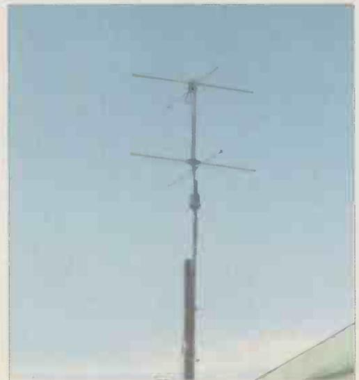
**Fig. 1: Crossed dipole 137MHz antenna (on my roof).**
