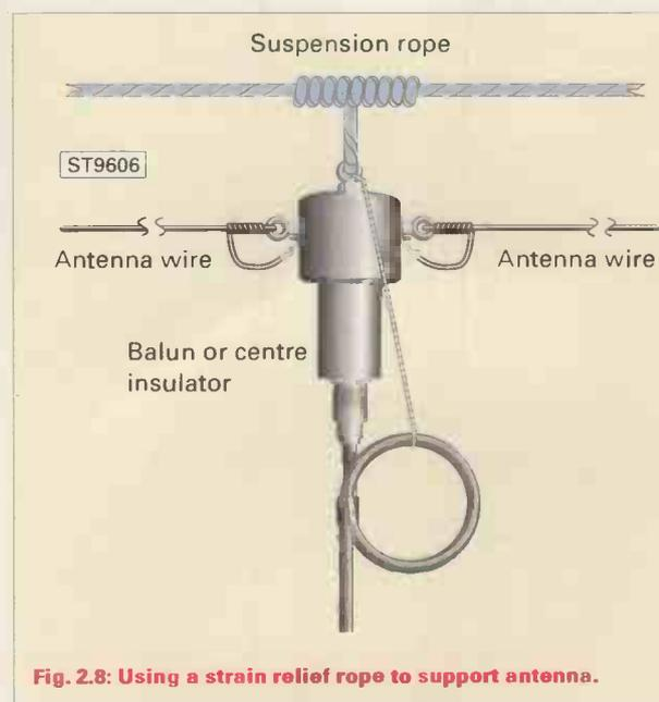
Fig. 2.8: Using a strain relief rope to support antenna.
