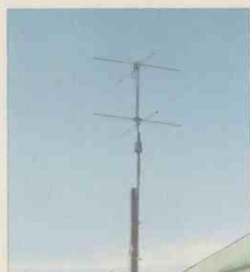
**Fig. 1:** Crossed dipole 137MHz antenna (on my roof).
