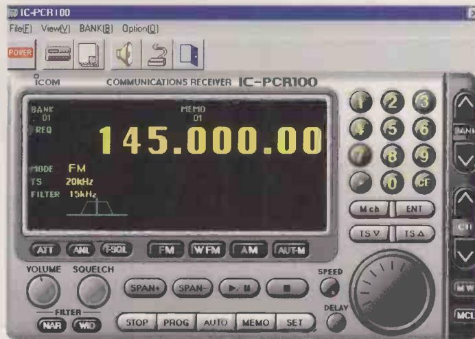
As you can see from the screen shot, the main component of this mode is the status and frequency display area, where the frequency you are listening to is shown.
