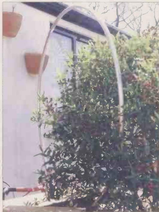
**Even here with a plant growing through the middle, the ALA 1530 is a great performer. I didn't notice any measurable difference with out the horticulture so this is where it ended up. Note the paving slab supporting the antenna.**
