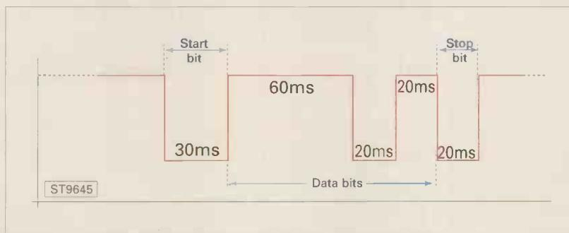
**Fig. 1: RTTY Signal Timings and Signal Elements.**
