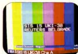
**SNG colour bars ex Serbia from SISLinks UK based truck. Note the service ident data flagged across the lower screen, the '151' relates to my receiver memory for this channel.**
