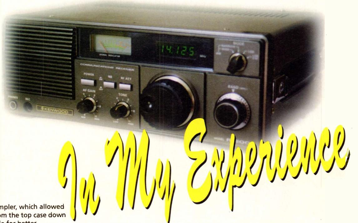
R-1000, the back-lit 0 to 1000 analogue dial is not provided, so loss of the digital display would leave you flying blind. The only other rotary controls are 'Volume' and 'Tone' - no r.f. gain control for the purist.
