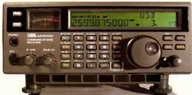
True base receivers are few and far between, some have simply evolved from the hand held equivalents with little tangible improvement in performance or facilities over their smaller counterparts - the AR5000 is not like this! High performance, top quality build and true wide coverage all mode receive. The "+3" version offers even more with synchronous AM, AFC and Noise Blanker. Popular with government agencies throughout the world.
