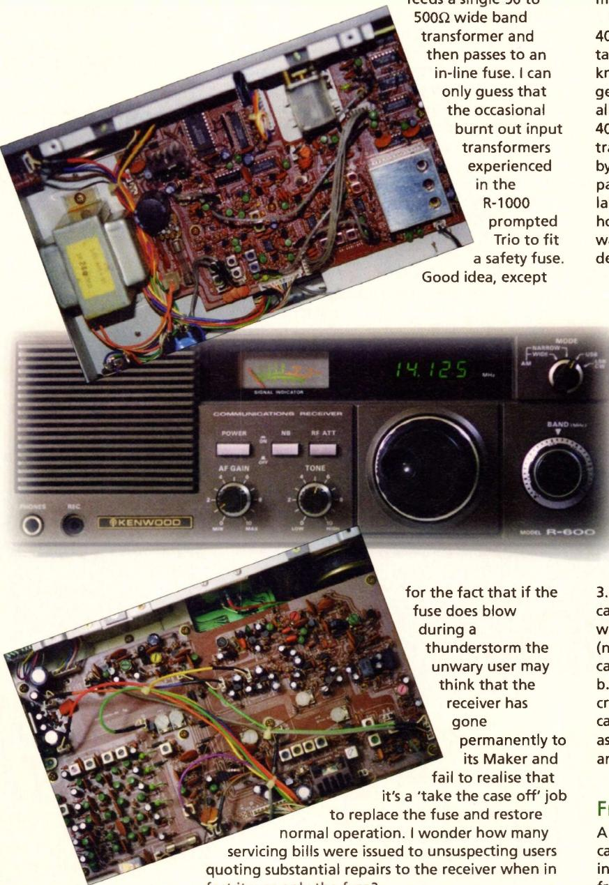
for the fact that if the fuse does blow during a thunderstorm the unwary user may think that the receiver has gone permanently to its Maker and fail to realise that it's a 'take the case off' job to replace the fuse and restore normal operation. I wonder how many servicing bills were issued to unsuspecting users quoting substantial repairs to the receiver when in fact it was only the fuse?
