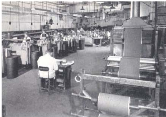
• This picture shows a stage in the making of magnetic tape. Note the wide strip unrolling from the machine on the right.
