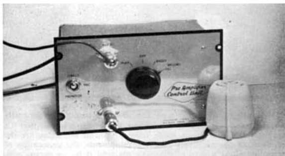
The pre-amplifier/control unit is as simple as it is efficient. A co-axial socket at the foot of the panel accepts the co-axial plug of the selected microphone. Connection to the tape head, is made via the second co-axial socket at the top of the panel. The main control knob is a switch with 4 positions for replay, off, and radio or mic record.
