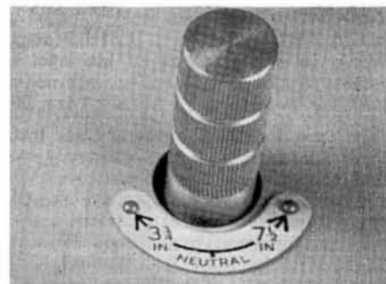
Figs. 4 and 5: Above, is the speed control, 3\frac{1}{2} i/s on left, neutral in centre, and 7\frac{1}{2} i/s on right. The photo on the left shows the push-button arrangement. As can be seen by the engraving, the centre three buttons are grouped for pre-set control. The right (green) button is for "run" and the left (red) button is "stop".
