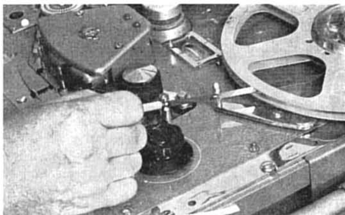
Accurate marking is essential, and when the replay head is inaccessible you should find a fixed offset point, e.g. a tape guide as shown. (BBC Photo).
