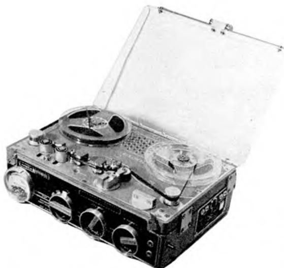
Left: The Nagra 111B battery or mains-operated portable recorder
