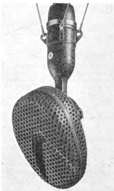
ST & C 4038, a ribbon microphone based on the BBC-designed PGS
