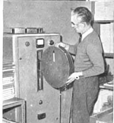
*When Emitape returns from the studios to the BBC Central Maintenance Unit, it is re-serviced, passing through this 'washing machine'. A giant electromagnet finally wipes off any signals remaining on the tape.*
