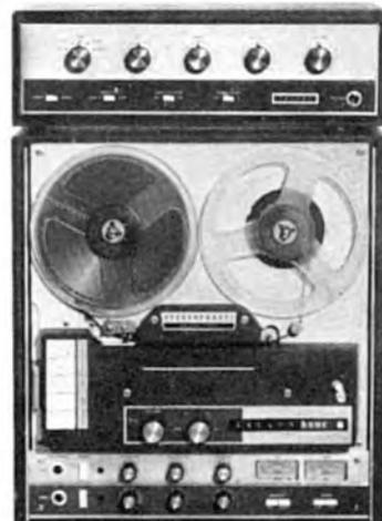
The recorders incorporate built-in 8 x 5 inch elliptical loudspeaker units handling the five watt power output. The two PD tape units include one volt emitter follower output sockets.
