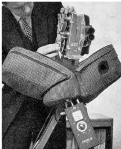
**A synchroflex magnetic film recorder fitted to the side of a Bolex H.16 for shooting in lip-sync. The large chequered bag is the soundproof blimp which zips up round the camera. The amplifier is hanging on the tripod below the blimp**
