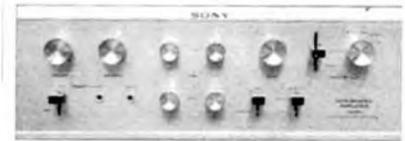
circuit on the incoming signal can be switched out to present an absolutely flat response for comparative purposes. A mode selector is provided for reverse stereo, left, right, and left and right combined. Silicon transistors are used throughout and the rated output is 30 watts with a distortion figure quoted as less than 0.1 per cent. In modern styling, with an oil stained wooden case as an optional accessory, the recommended retail price is 99 guineas.
