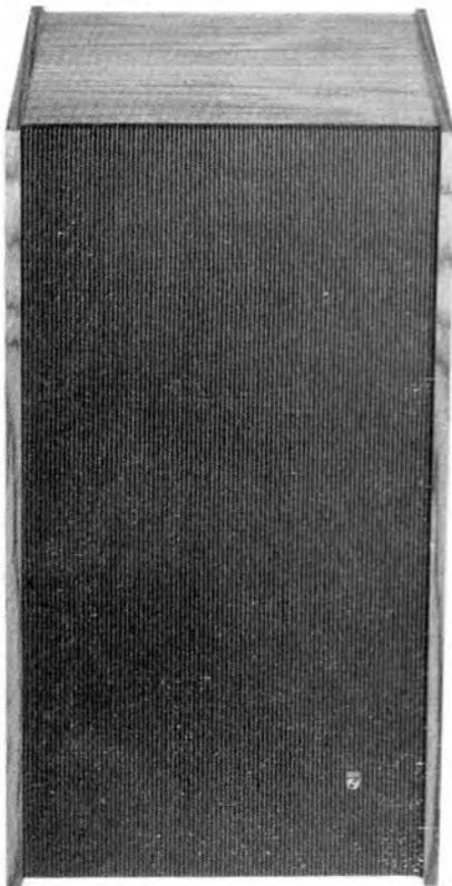
The enclosure contains a 7-inch low frequency pump employing a rigid light-weight expanded polystyrene cone and a 4-inch dual cone high frequency reproducer. The crossover frequency is 550 cycles.
