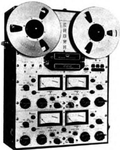
Three speeds, 15, 7½ and 3½ ips are standard, but other speeds can be supplied to order. Typical performance figures are 15 ips for a two-channel half-track recorder which is quoted as ± 2 dB from 50 to 30,000 Hertz, wow and flutter better than 0.06 per cent and signal-to-noise ratio better than 60 dB.
