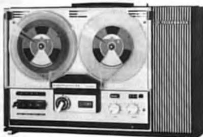
Frequency response is given as 60-13,000 Hertz, wow and flutter as better than 0.3 per cent and signal-to-noise ratio as 46 dB. Output power is claimed to be 2.5 watts and sockets are provided for microphone, radio pickup, headphones and external speaker. The Plexiglass lid can be left on the machine during operation as it is designed in such a way that access is still freely available to the control panel. Recommended retail price of the Magnetophon 202 is £72 12s 6d inclusive of purchase tax.
