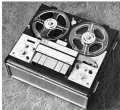
The RR100 is said to allow the user to perfect his technique by frequent repetition, comparing his recordings with a master track if required. The recording is made in short sections with rapid playback and re-recording of each section until the passage is correct, when that section of tape is allowed to feed on to the take-up spool.
