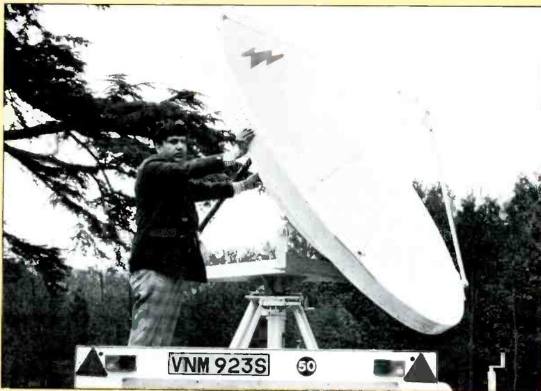
▲ This trailer-mounted 14 GHz transmitting antenna forms part of the IBA's transportable up-link terminal – the first of its type to be built in Europe. IBA
