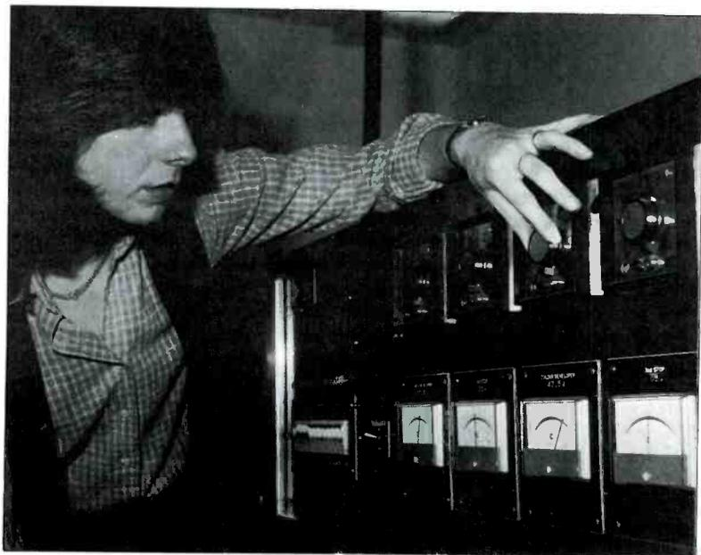
◀ Good colour pictures in the home depend to a large extent on the quality of the original film or recording. Here the film processor adjusts the temperature of the colour development on a 16mm VNF 1 process machine.
