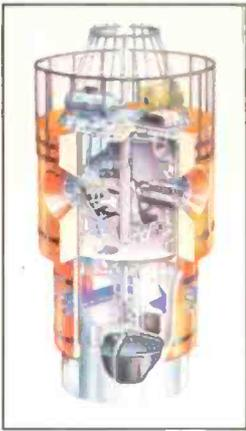
▲ **Project Aries.** This 16 ft. tall double-deck gondola is designed to attach to a massive Helium hot air balloon (1 million cubic feet) which will travel at 80 m.p.h., 7 miles above the ground, in an attempt to complete a first non-stop round-the-world voyage. *ATV*
