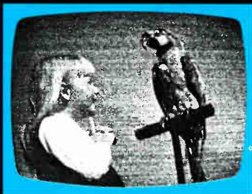
**Weak Signal.** Low signal strength, often resulting from an inadequate or poorly adjusted aerial, can result in a 'noisy' or grainy picture.
