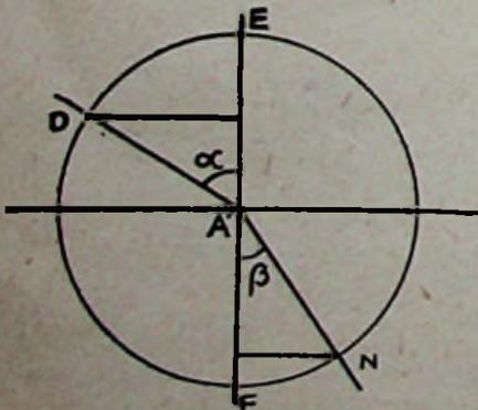
Fig. 3.—Diagram illustrating Snell's law of refraction.
