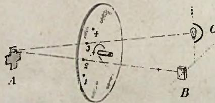
A beam of light from the source C shines through the lens 3 of the revolving disc on to the object A. Light reflected from A passes through lens 2 of the disc and strikes the light-sensitive cell B.
