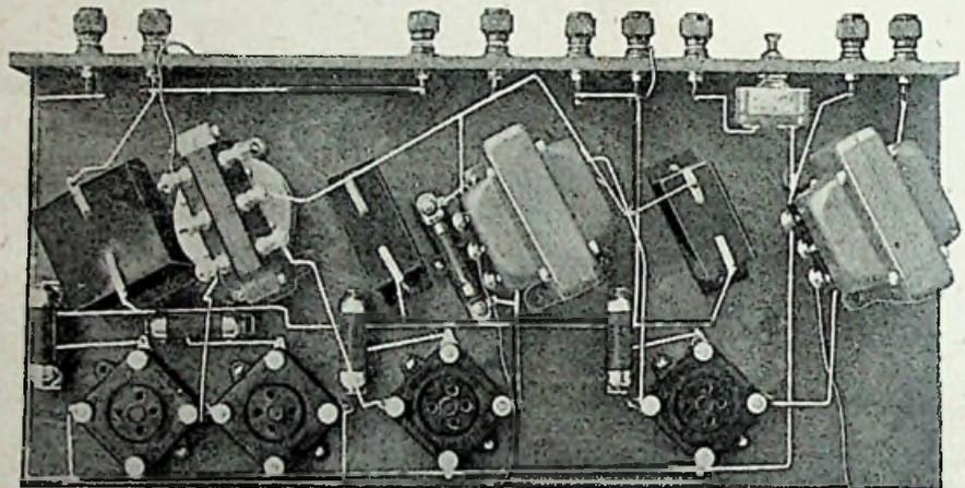
A plan aspect showing the baseboard layout. It is important to follow this closely as any modification may result in instability. Across the centre L.F. transformer is connected the 100,000 ohm resistance.
