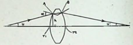
Fig. 4.—Illustrating trigonometrical ray-tracing.
