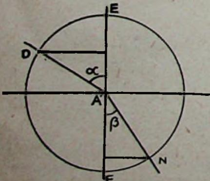
Fig. 3.—Diagram illustrating Snell's law of refraction.
