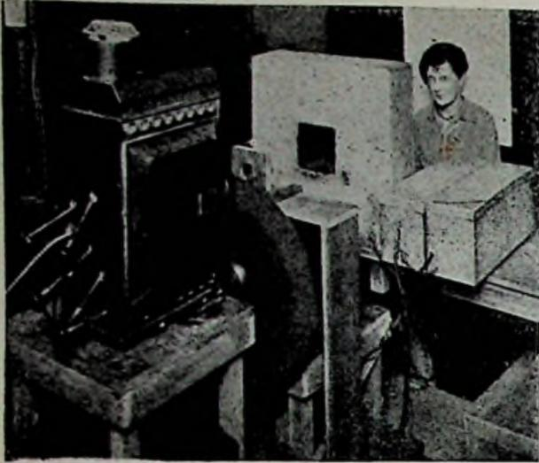
The projector lamp and revolving disc. The beam of light shines through the square opening on to the figure to be transmitted. Behind the opening, and round it, are grouped three photo-electric cells. (See "Technical Notes," page 12.)
