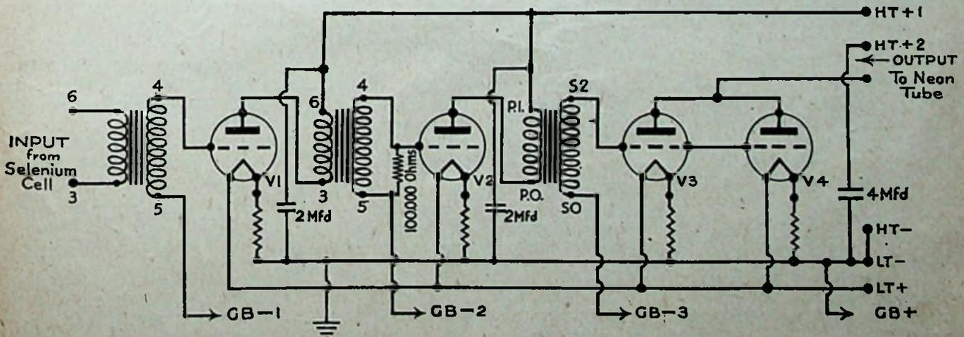
The complete theoretical diagram of the amplifier showing exact connections
