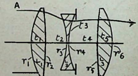
Fig. 5.—The Cooke photographic lens.
