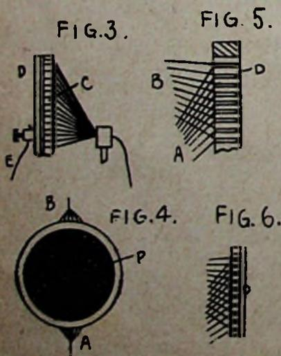
Figure 5 is a sectional view of disc P (Figure 1) showing selenium points and conducting wires.
