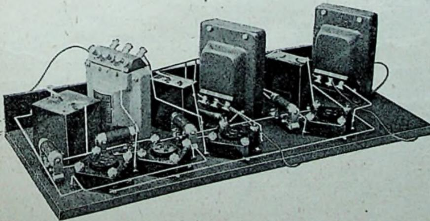
The layout of the amplifier is clearly shown by this illustration. It will be noted that large by-pass condensers are arranged across the high-tensionappings.
