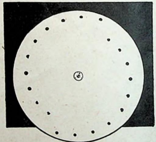
Spiral Disc as specified, 20 in. diam. aluminium.
