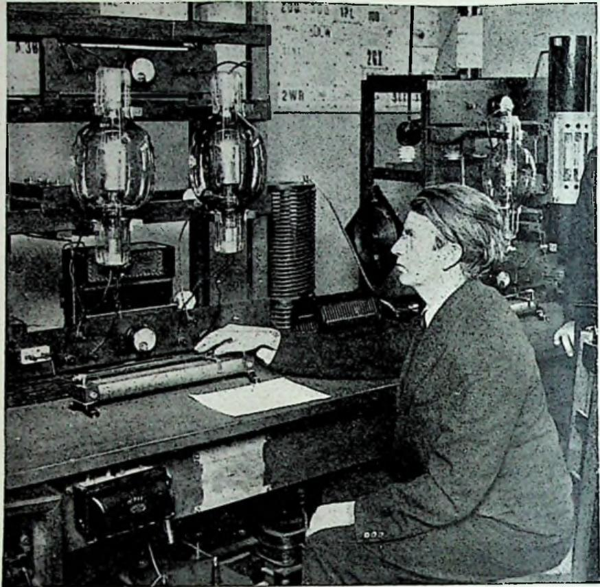
Mr. J. L. Baird seated before the 2 kw. amateur wireless transmitter which performed such yeoman service in the recent transatlantic experiments. The station is at Coulsdon, Surrey; its call sign is 2 KZ, and its wave-length is 45 metres. Television transmissions may sometimes be heard from this station after midnight.
