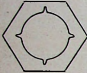
Fig. 2. Actual size of nut used for threading ebonite bushes. Note the four cuts in the thread of the nut, which can be used as a die.
