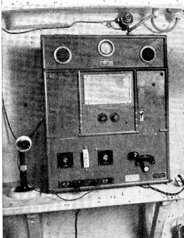
*Marconi wireless telephone transmitter type XMB1 installed on the new Dover lifeboat of the Royal National Lifeboat Institution. This lifeboat (which is the fastest in the world) has been specially designed for the rescue of aeroplanes which have fallen into the sea.*
