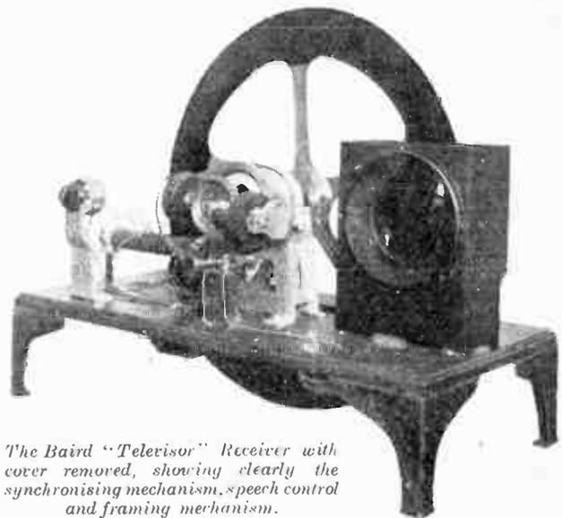
The Baird "Televisor" Receiver with cover removed, showing clearly the synchronising mechanism, speech control and framing mechanism.
