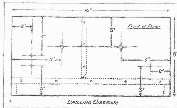
Fig. 1.—All the dimensions for marking out the panel are shown here.
