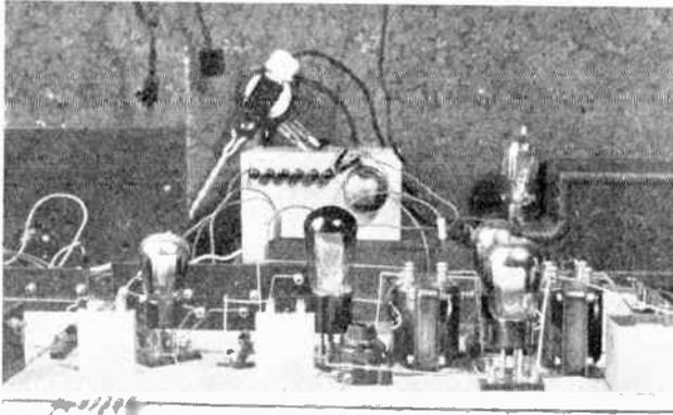
Mr. J. W. A. van Schie has made up this amplifier for use in connection with the reception in Holland of the Baird television broadcast.
