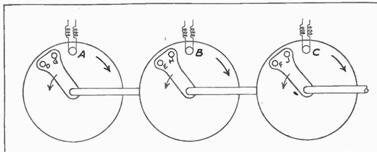
Fig. 1.—Indicating in diagrammatic form how magnetic recording is carried out for expediting the transmission of television signals.
