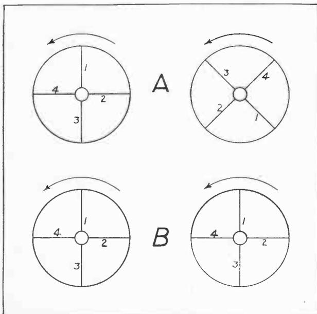
Fig. 2.—Synchronism is established at B but only isochronism at A.
