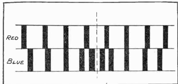
Fig. 3.—Interference fringes produced by red and blue light.
