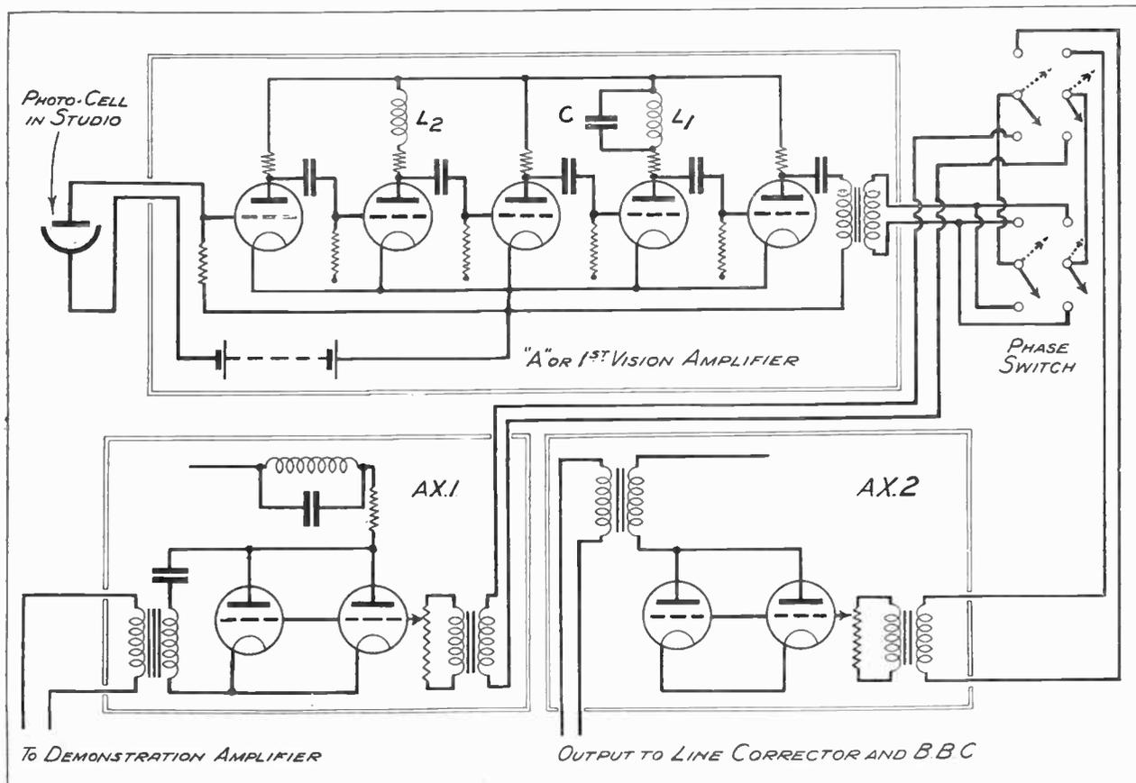
Fig. 2.—Special amplifiers are required for handling the vision signals with a change-over switch for line demonstrations or B.B.C. working.
