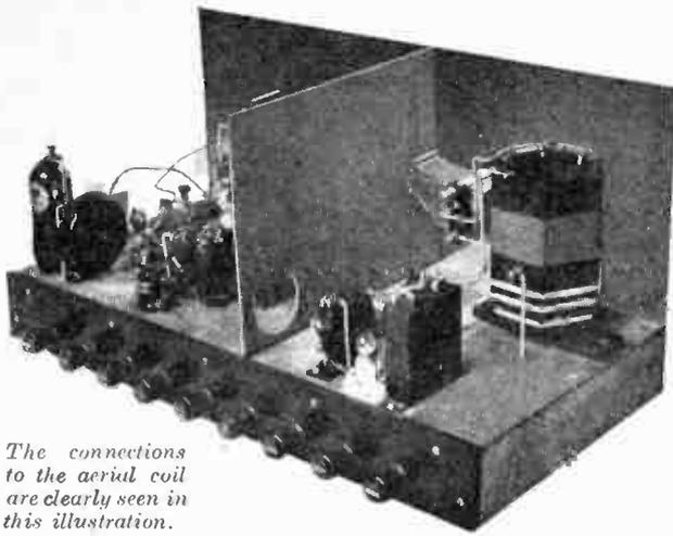
*The connections to the aerial coil are clearly seen in this illustration.*
