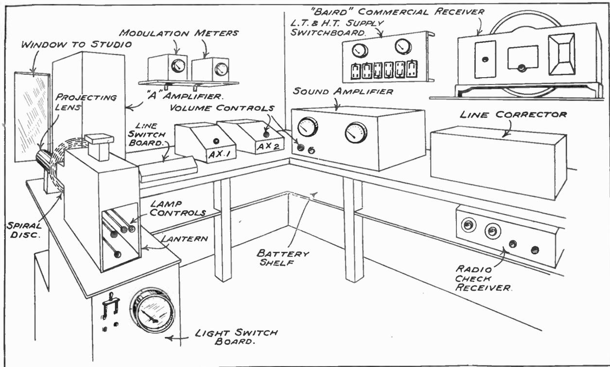
Fig. 1.—The general lay-out of the control room is made quite clear by studying this sketch. All the controls are readily accessible and arranged with extreme care.
