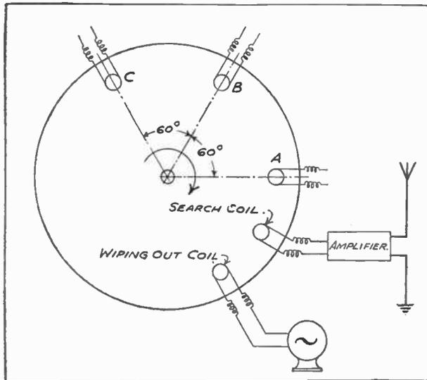
Fig. 2.—Another suggested method whereby a magnetic disc is employed for simultaneous exploration.
