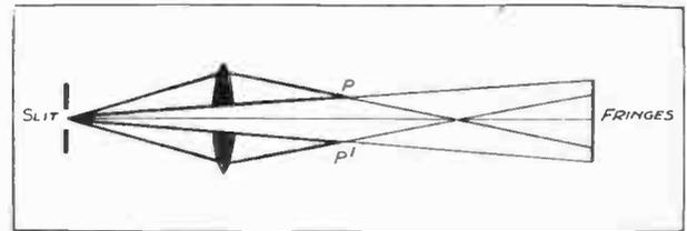
Fig. 6.—Billet's split lens method.  $P$  and  $P^1$  are the two sources.
