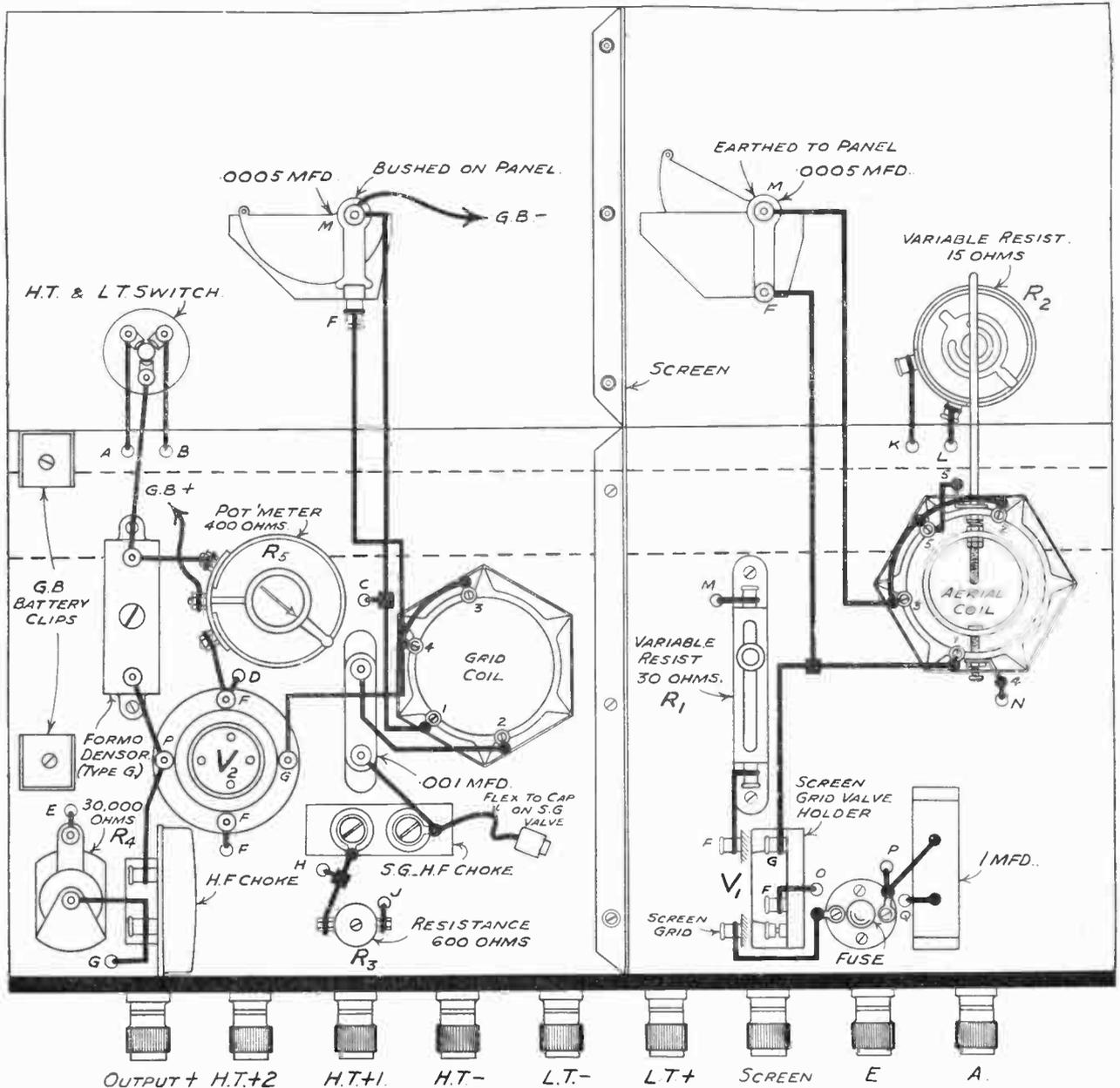
Fig. 2.—The complete wiring diagram for the panel and above baseboard. Note the lettered holes for wires passing through the baseboard.
