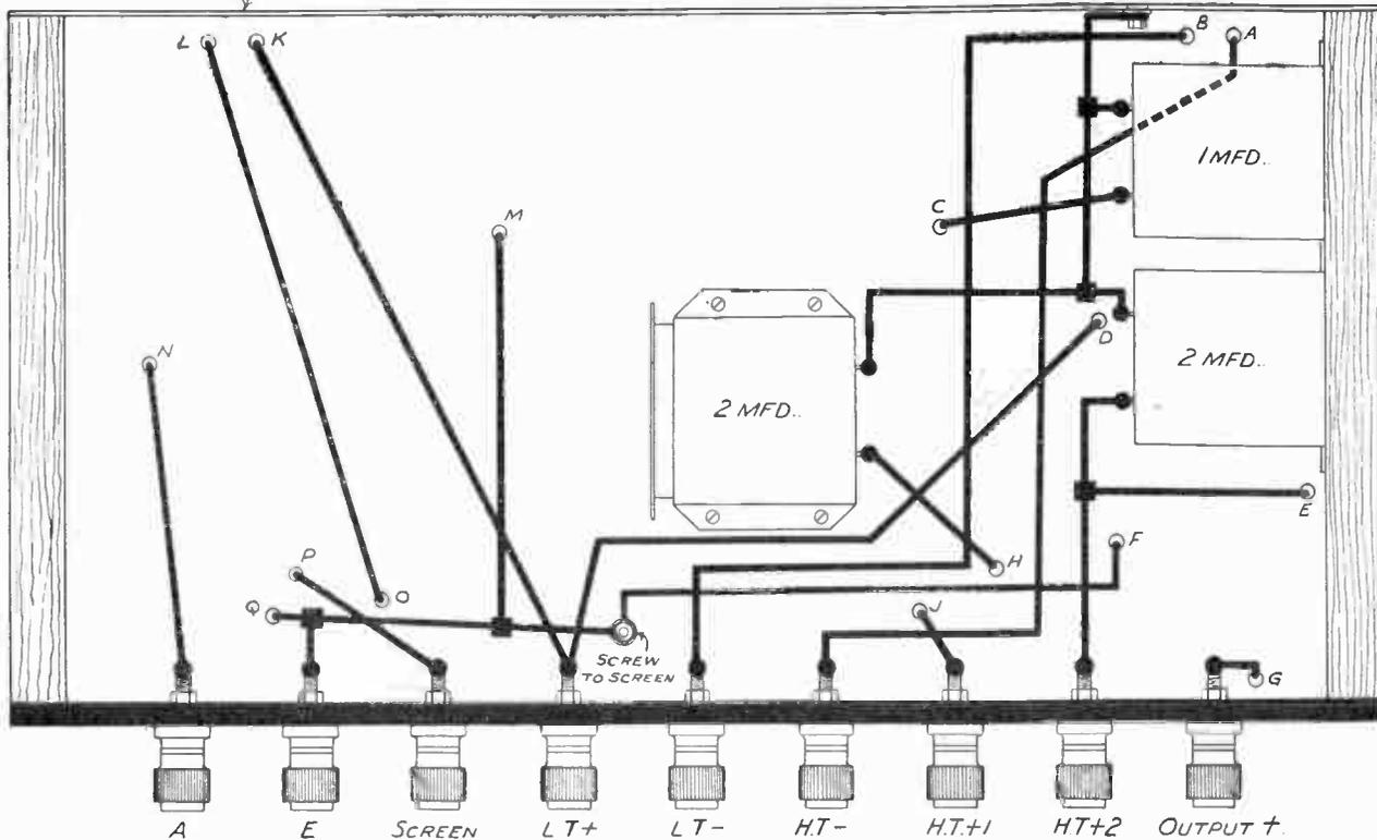
Fig. 3.—Details of the wiring which must be executed under the baseboard. Do not omit the earthing screen screw.
