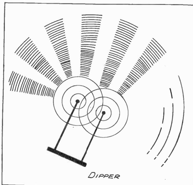
Fig. 1.—Picture of interference fringes on the surface of water or mercury.
