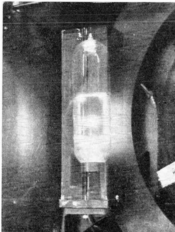
Showing a flat plate neon being scanned while glowing.
