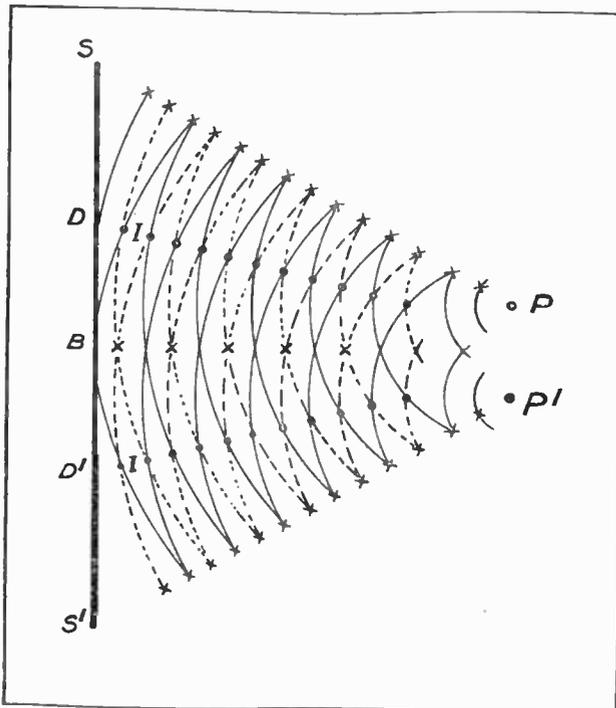
Fig. 2.—Illustrates the interference of waves.
