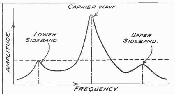
An asymmetric resonance curve showing amplitudes and relative sharpness of the upper and lower sidebands.
