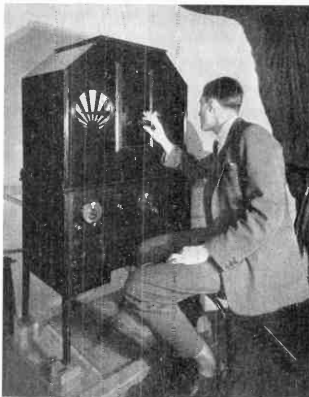
Receiving a Television transmission on a Baird Dual Exhibition Receiver. The apparatus shown contains two wireless receiving sets, one for speech and one for vision. The "televicser" is fitted with a Baird automatic synchronising apparatus.
