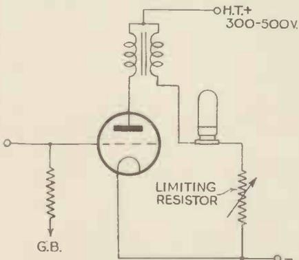
Transformer-coupled arrangement of mercury lamp where H.T. voltage is limited. The resistor is essential for current limitation.
