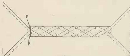
Fig. 7. Diagram showing the internal reflection.
