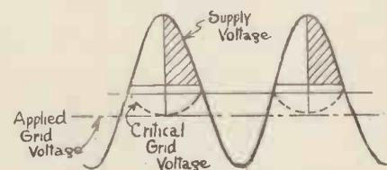
Fig. 7 Condition when critical bias is applied.
