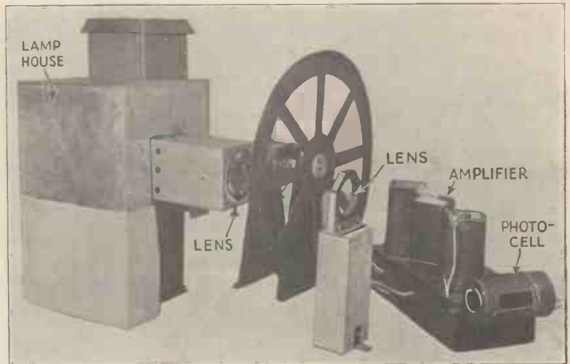
Here are the units of the simple transmitter arranged in "hook-up" form.
