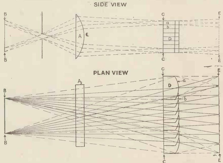
Fig. 6. The complete Stixograph optical system
