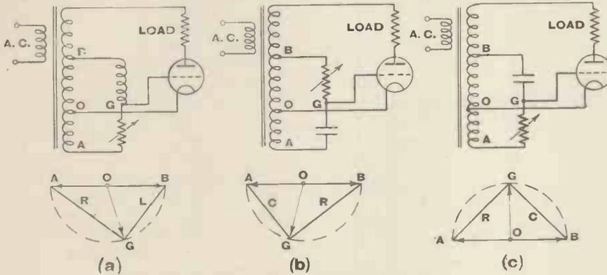
Fig. 8 Three typical grid-circuit arrangements.
