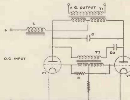
Fig. 13. A self-exciting inverter circuit.
