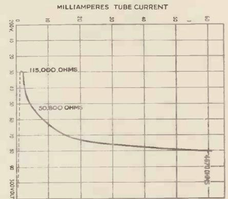
Characteristic curve of mercury-vapour tube.
