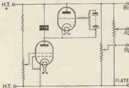
Fig. 4. Simple time base adapted for use with mains valves. The letters refer to the plates of the oscillograph
