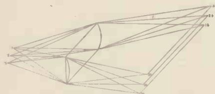
Fig. 3. The focus of points lying in a line not parallel to axis of curvature
