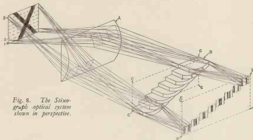
Fig. 8. The Stixograph optical system shown in perspective.
