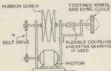
A suggested layout for driving a mirror screw by step-down belt gearing.
