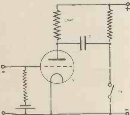
Fig. 10 A method of resetting the relay.
