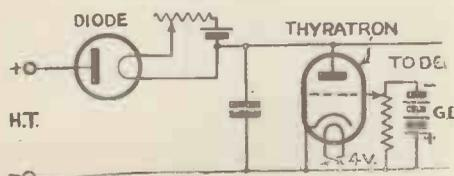
Fig. 1. The circuit with a saturated diode in place of the resistance
