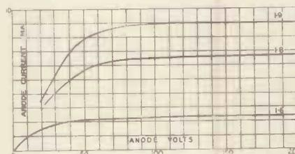
Fig. 2. Characteristic curve of the CR2
