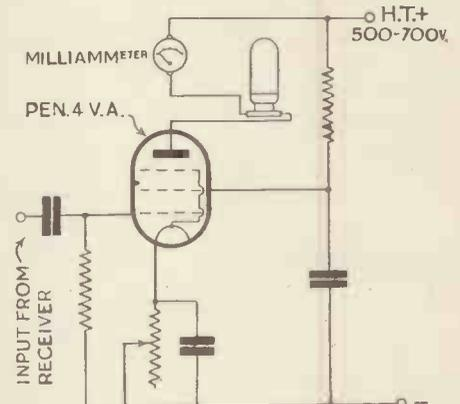
Recommended circuit for use with a mercury-vapour lamp, the current is controlled by means of the bias resistor.
