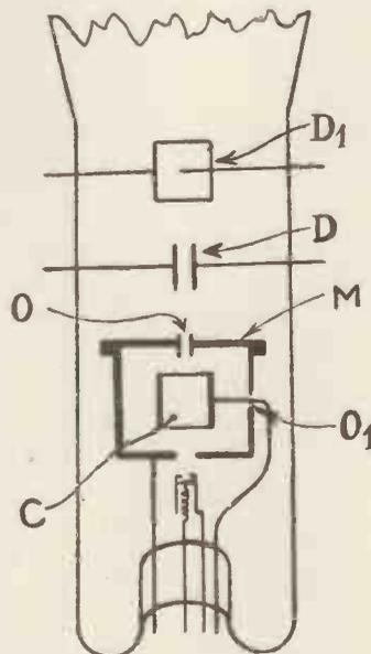
A method of obtaining sharply defined scanning at high speeds.
