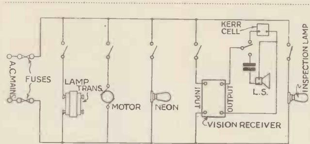
Circuit diagram showing how the various connections are made.
