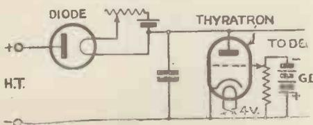
Fig. 1. The circuit with a saturated diode in place of the resistance
