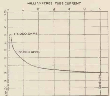
Characteristic curve of mercury-vapour tube.
