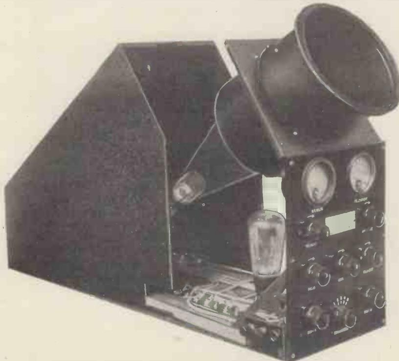
Ediswan portable cathode-ray tube equipment shown partly withdrawn from its case. Underneath the tube can be seen the thyatron for the time-base. On the front panel are the controls for the time-base and for the focusing tube
