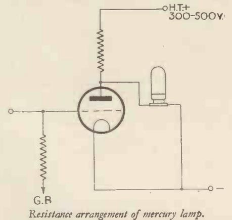
Resistance arrangement of mercury lamp.
