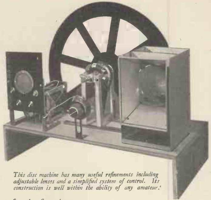
*This disc machine has many useful refinements including adjustable lenses and a simplified system of control. Its construction is well within the ability of any amateur.*
