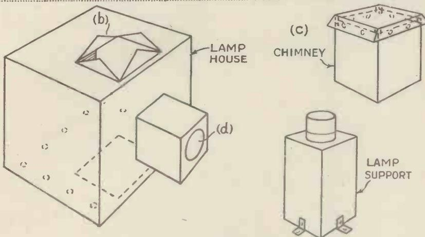
Details of lamp house, chimney and lamp support.
