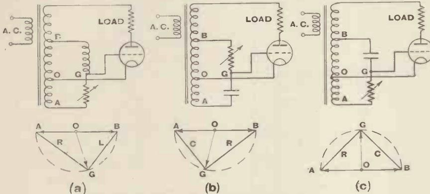
Fig. 8 Three typical grid-circuit arrangements.
