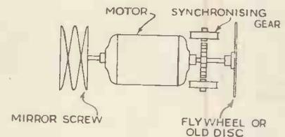
A simple way of stabilising motor speed
