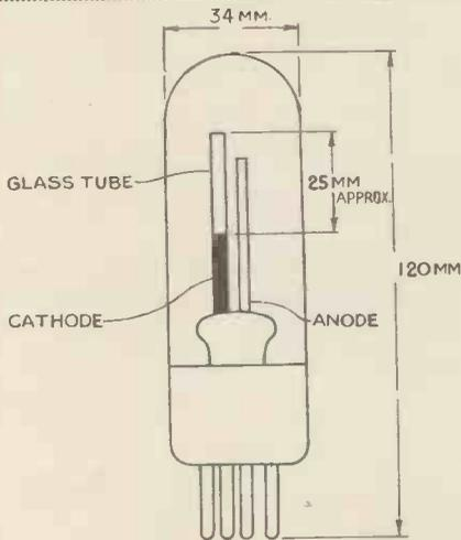
A diagram of the type D2 G.E.C. mercury recording tube.
