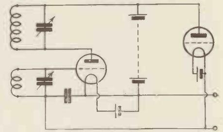
Fig. 6. "Ticking-grid" time-base circuit, developed by Appleton, Watson-Watt and Herd, using a valve oscillator
