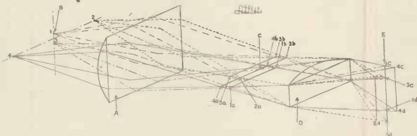
Fig. 4. Diagram showing the action of two cylindrical lenses
