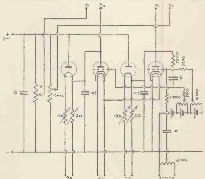
Fig. 3. The circuit of the complete double time base employing saturated diodes
