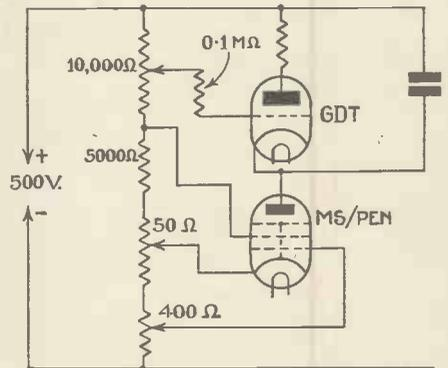
Fig. 2. Fine adjustment on the 375 base is essential.
