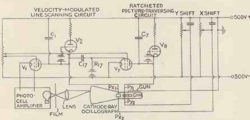
Fig. 1. The schematic circuit of the transmitter for producing velocity-modulated scanning.
