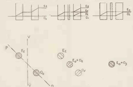
Fig. 1. A diagram explaining the action of the double-image polariscope.
