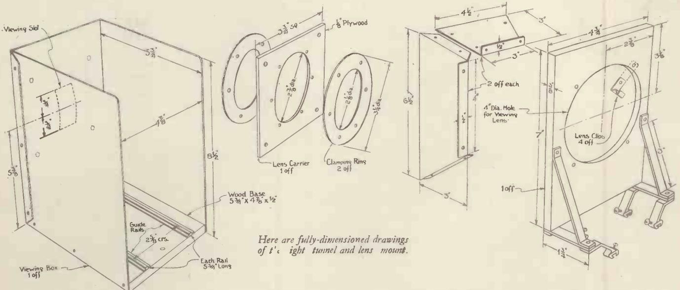
Here are fully-dimensioned drawings of the light tunnel and lens mount.
