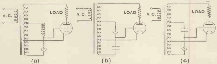
Fig. 9. Three arrangements showing how the gas-filled relay is adapted to be worked from a photo-cell.
