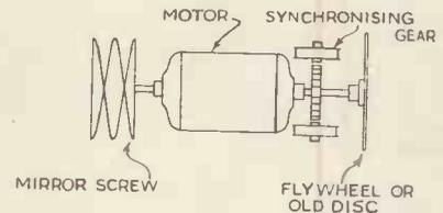
A simple way of stabilising motor speed
