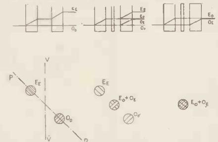
Fig. 1. A diagram explaining the action of the double-image polariscope.
