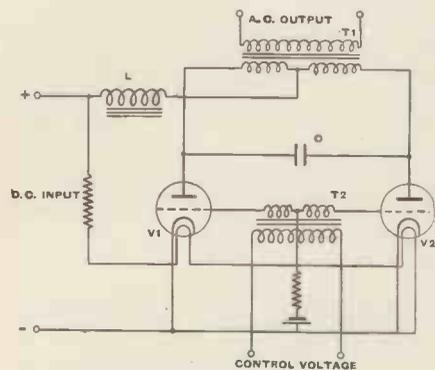
Fig. 12. An inverter circuit.
