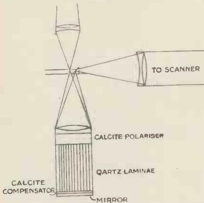
Fig. 4. Quartz aperiodic modulator.
