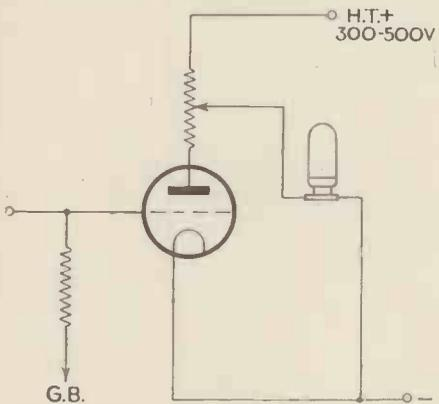
A useful circuit where voltage is limited; the value of the resistor should be equal to the optimum load of the valve, the amount of modulation being controlled by moving the slider.
