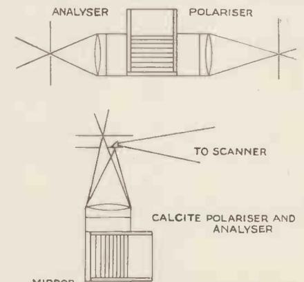
Fig. 2. Two forms of light modulator.
