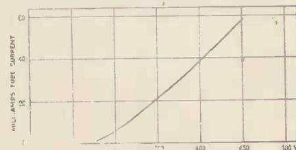
The characteristic curve of the G.E.C. D2 recording tube.
