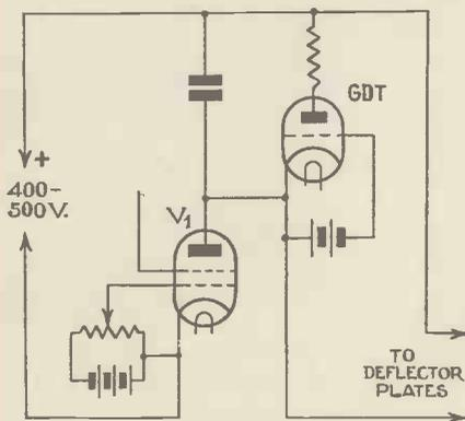
Fig. 1. A simple gas-discharge time base.
