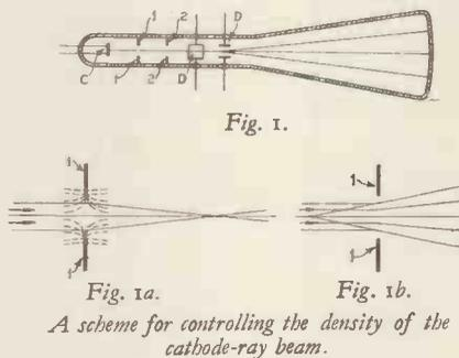
whilst a positively-charged ring is the equivalent of a concave lens. This enables a reduced or enlarged image of the spot to be produced on the fluorescent screen as desired. A combination of ring and disc may be used to produce a sharper focal effect.—(*Siemens-Shuckertwerke Akt.*)
