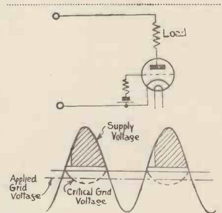
Fig. 6 Showing the effect of biasing the grid of the gas-filled relay.
