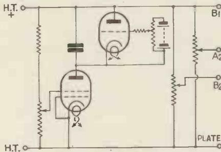
Fig. 4. Simple time base adapted for use with mains valves. The letters refer to the plates of the oscillograph
