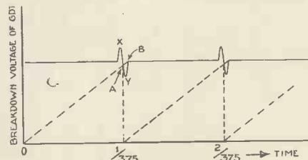
Fig. 3. Illustrating the mechanism of synchronising.
