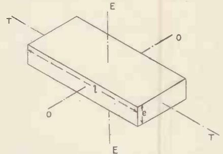
Fig. 5. Piezo-electric quartz showing how the application of an electric field brings about a strain.
