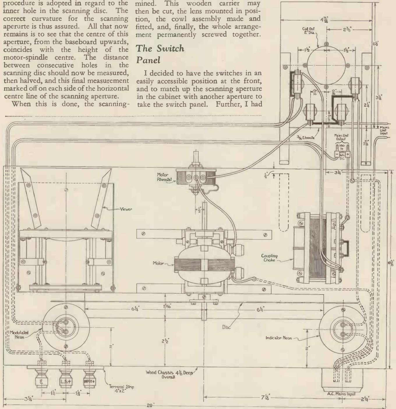
A plan view of the disc receiver showing the wiring. A large-scale blueprint is available, price 1/-
