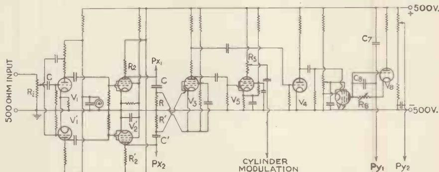
Fig. 2. The circuit of the receiver which comprises a line-scanning amplifier, picture-traversing time-base and an intensifying system.
