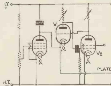
Fig. 5. Time base employing hard valves used by the Cossor Co.
