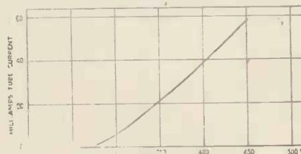
The characteristic curve of the G.E.C. D2 recording tube.
