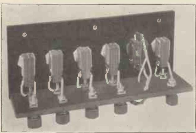
The switches are connected to terminals to facilitate coupling up the several circuits. These terminals may be omitted if desired.
