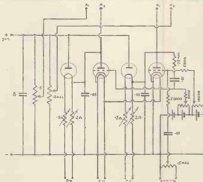
Fig. 3. The circuit of the complete double time base employing saturated diodes
