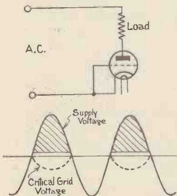
Fig. 5 Diagram showing the formation of unidirectional pulses when A.C. is applied to a resistance loaded gas-filled relay.
