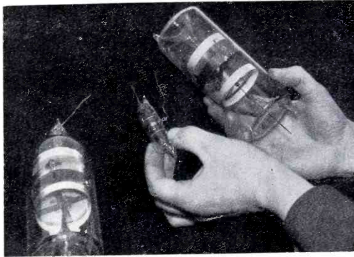
Three forms of electron multiplier are shown by this photograph.
