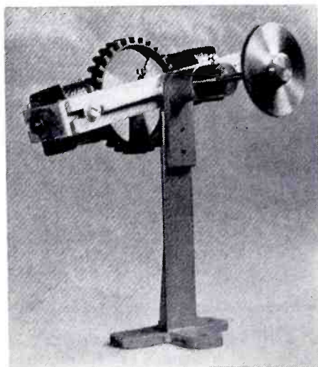
The Sanders synchronising gear is adaptable for every type of mechanical scanner.
