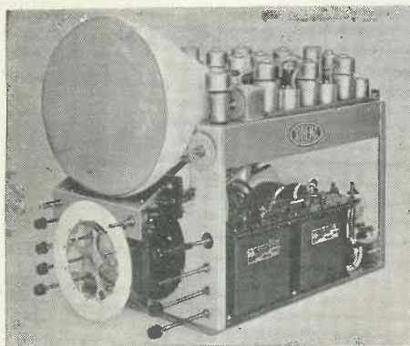
This photograph shows the chassis of the Lorenz receiver.
