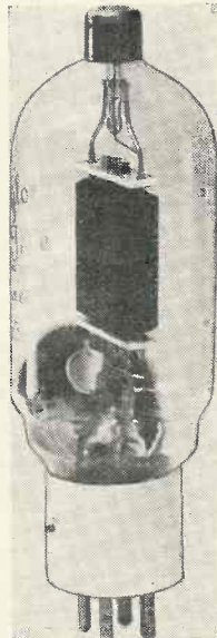
The T-40 and TZ-40 both of which have carbon anodes and are suitable for an anode dissipation of 40-watts, are very small in dimensions, being only 2-ins. in diameter: It is, however, possible to obtain an audio output of 170-watts from a pair of TZ-40's and 85-watts carrier power from one T-40.
