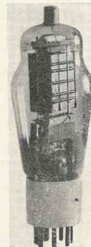
As the maximum grid driving power of this Tungram valve OS12-500 pentode is only 1/10th-watt, it is possible to construct a multi-band transmitter with one of these valves driven by a 6L6 tri-tet oscillator.
