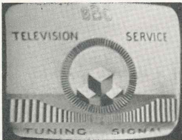
Fig. 2.—Here the effect of poor line synchronism during the framing period is revealed. Note the instability present at the top of the picture.
