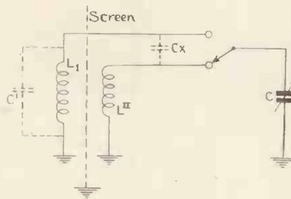
Fig. 3.—Absorption due to coupling by stray capacity.
