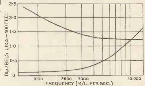
Fig. 6.—Twisted pair feeder characteristics. Velocity of propagation is 61.6 per cent. of free space at 1,210 k.c., 64.2 per cent. of free space at 3,300 k.c. and 68 per cent. of free space at 7,350 k.c.
