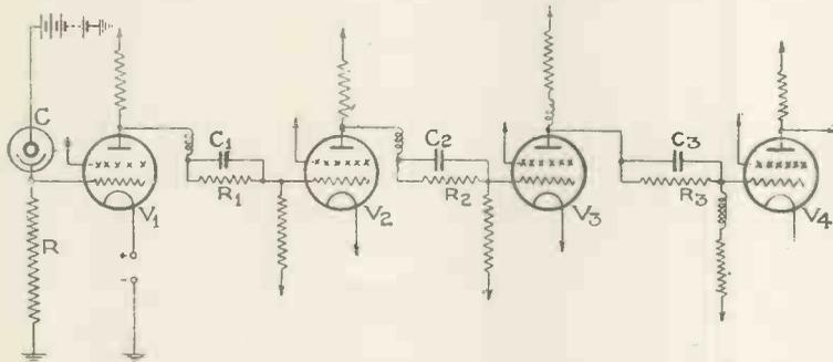
*Circuit of photo-cell amplifier, Patent No. 436,734.*
