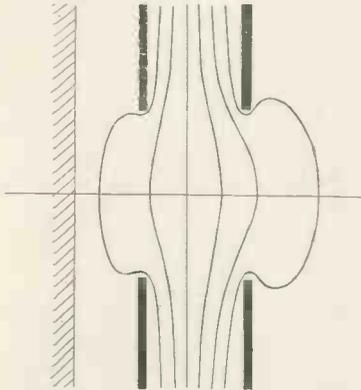
Fig. 3. Electron lens consisting of two apertures.
