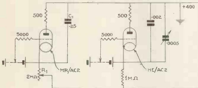
Fig. 1.—Time base circuit suitable for high-definition television employing gas discharge tubes.
