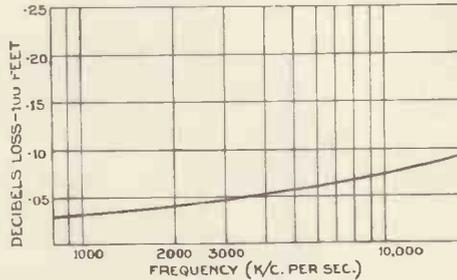
Fig. 4.—Loss versus Frequency with copper tube spaced 1. ins. Velocity of propagation is equal to 95 per cent. of free space measured loss.
