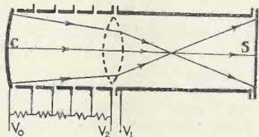
Fig. 1.—A simple electron lens system. Electrons from the cathode C are focused by the potentials applied to the cylinders and form an image on the screen S.
