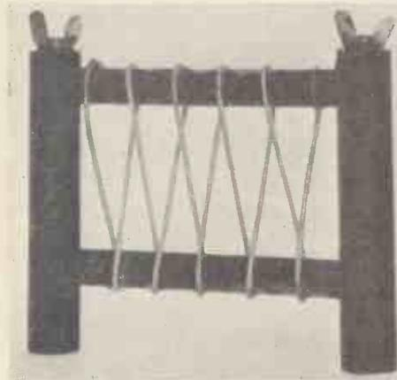
Fig. 32. A recommended type of grid and anode resistance wound non-inductively.
