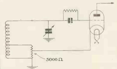
Fig. 2. Electron coupling is an arrangement that should be more widely used. This is a particularly good circuit.
