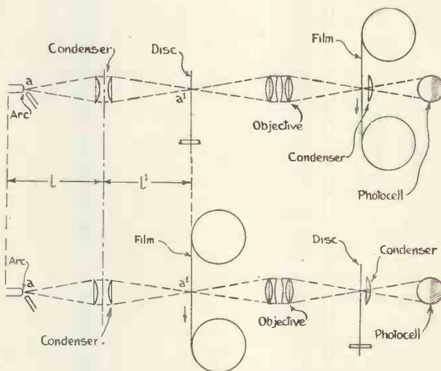
Fig. 1.—Simple optical layout of disc film transmitter.
