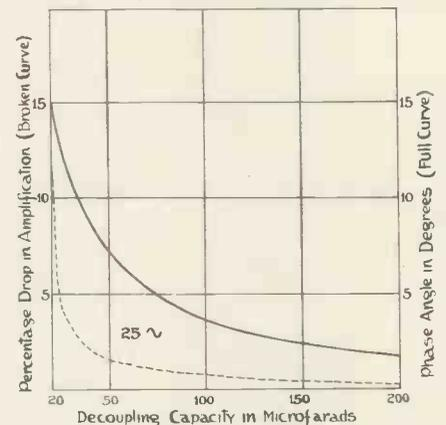
Fig. 5.—Showing effect with second method of decoupling for same valve as in Fig. 3.  $R_v = 10,000$ ,  $R_1 = 20,000$ ,  $R_3 = 100,000$ ,  $\mu = 30$ ,  $R_2 = 1,000$ .
