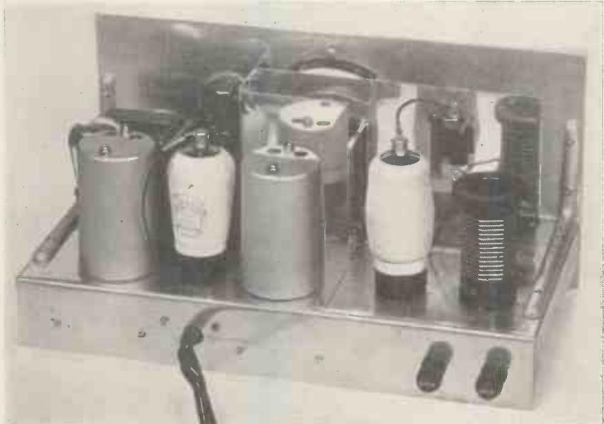
*The triode-pentode valve can be seen on the right-hand side next to the aerial coil.*
