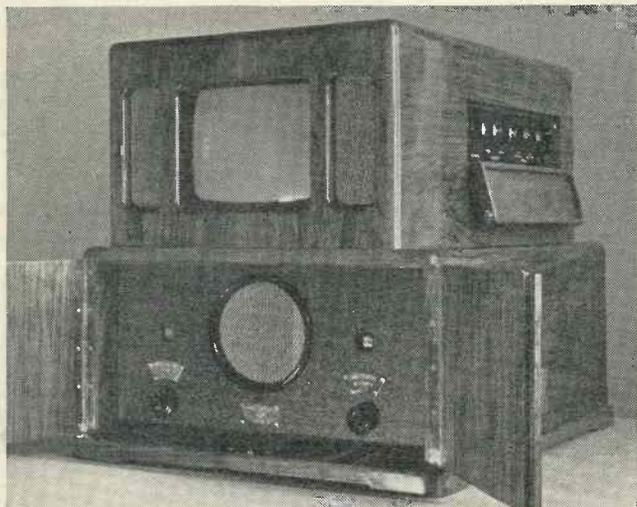
*Fernseh cathode ray tube receiver.*
