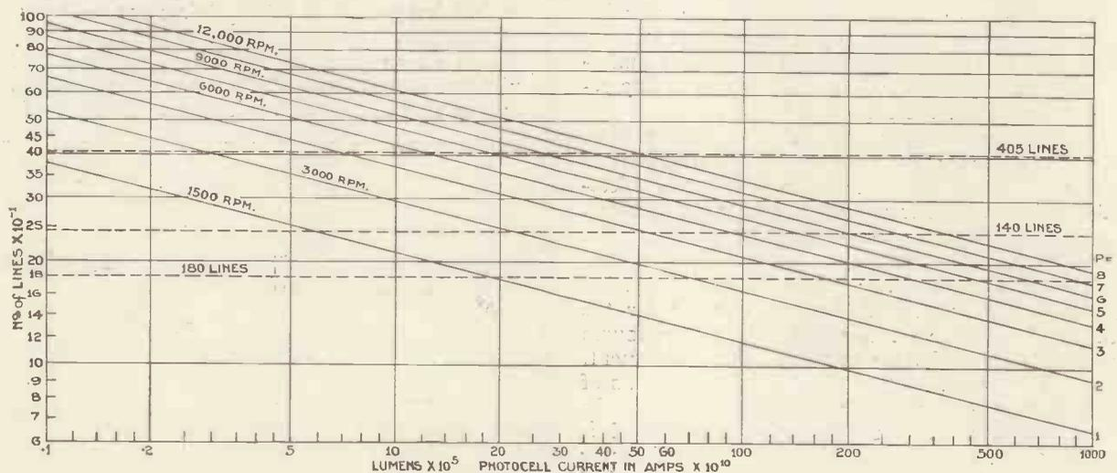
Fig. 2.—Graph showing the efficiency of the apertured disc film transmitter.
