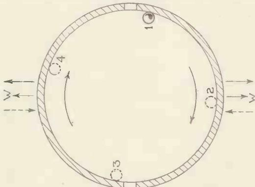
Fig 3.—An analogy of the method of operation of the split-anode magnetron.
