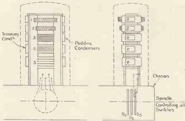
(Above) Fig. 9.—Arrangement of padding and trimming condenser for switched coil assembly. (Right) Fig. 10.—Complete circuit diagram for all-wave receiver with signal frequency and oscillator circuits.
