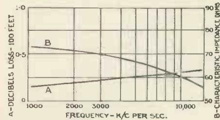
Fig. 5.—Concentric transmission line characteristics. Velocity is equal to 86.1 per cent. of free space between 2 and 10 M.C.
