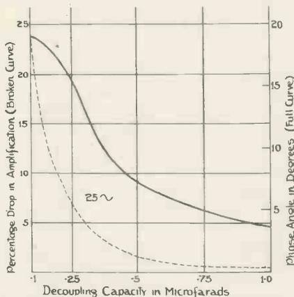
Fig. 4.—Showing effect of using screen grid valve.  $R_v = 500,000$ ,  $R_1 = 20,000$ ,  $R_2 = 500$ ,  $\mu = 1,000$ .
