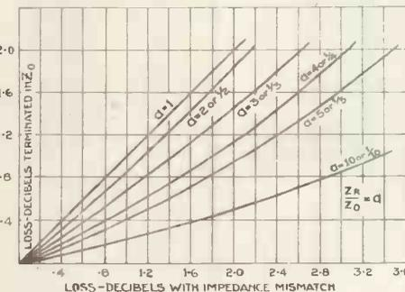
Fig. 2.—Chart for determining loss in given transmission line due to impedance mis-match.
