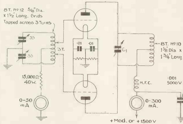
Fig. 3. A circuit of this type can be adapted to use any type of valve. Of course the anode voltage has to be re-adjusted, otherwise the circuit remains unchanged.
