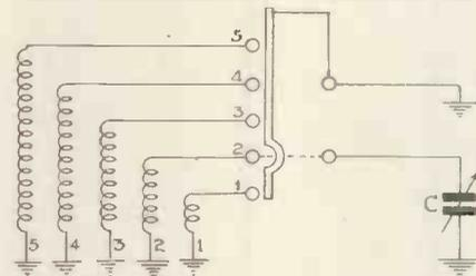
Fig. 7.—All unused coils short-circuited by single switch.
