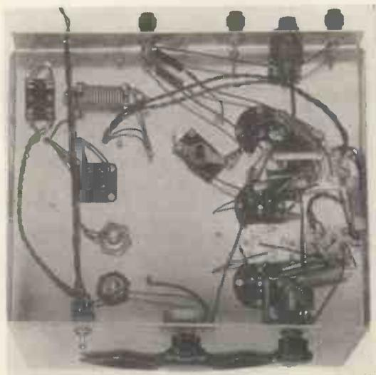
On the left of the photograph can be seen the 7,500 ohm. bleeder resistance which is across the main supply.
