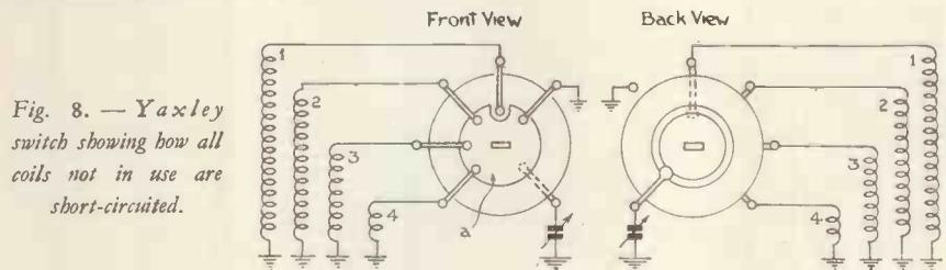
Fig. 8.—Yaxley switch showing how all coils not in use are short-circuited.
