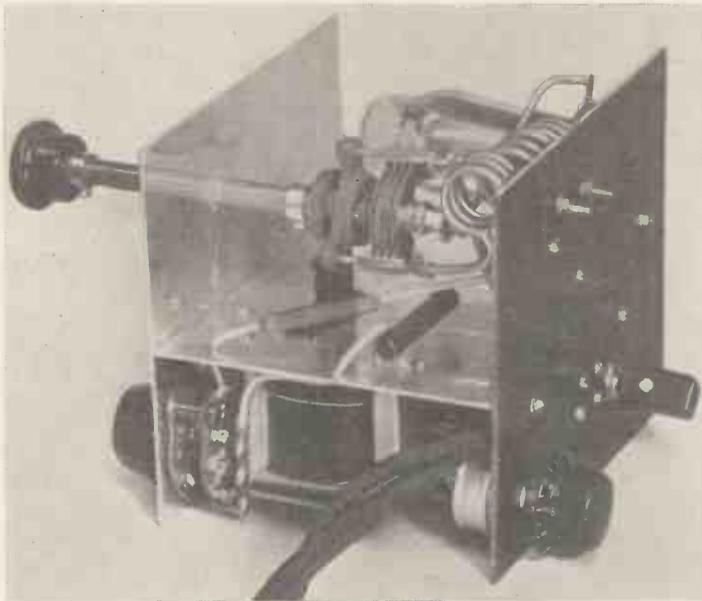
Fig. 3.—The two terminals at the top of the panel are for the aerial connections.
