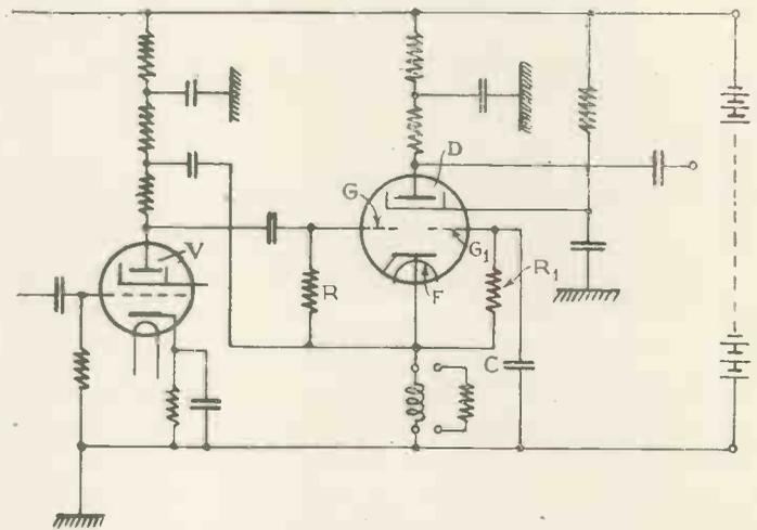
A.C. components are concerned, through a condenser C. The cathode F. is connected to the mid-point of two equal resistances R, R<sub>1</sub> in order
