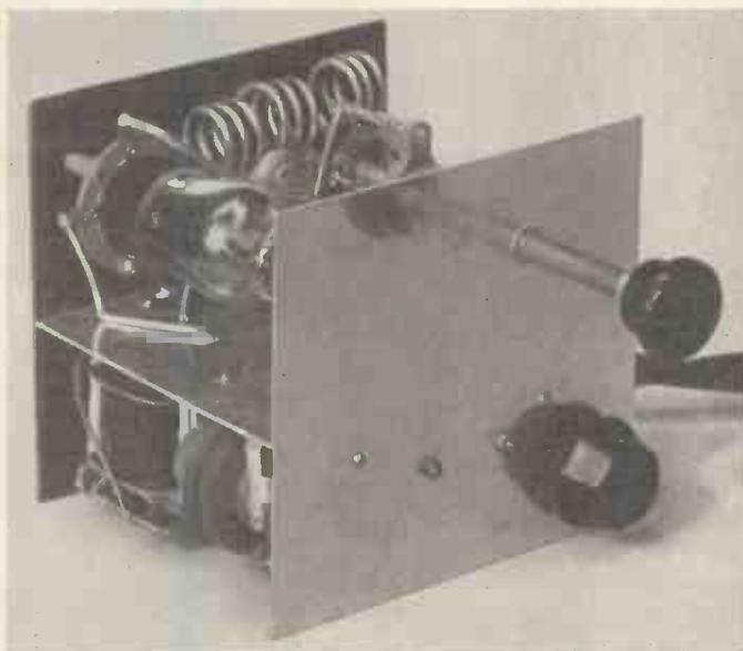
Fig. 2.—To make the unit more compact the master tuner can be made pre-set.
