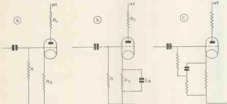
Fig. 1.—Automatic grid bias is derived from the voltage drop across  $R_2$ , but amplification is impaired.
