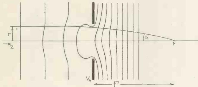
Fig. 1. Electron lens formed by a single aperture in a plate.
