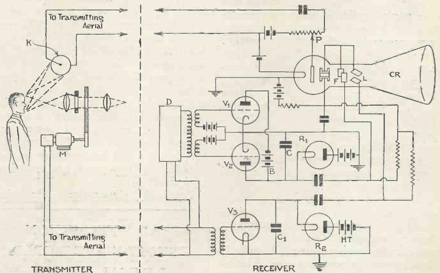
Fig. 2.—Time-base circuit for new method of interlaced scanning.
