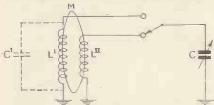
Fig. 2.—Absorption due to coupling by mutual inductance.
