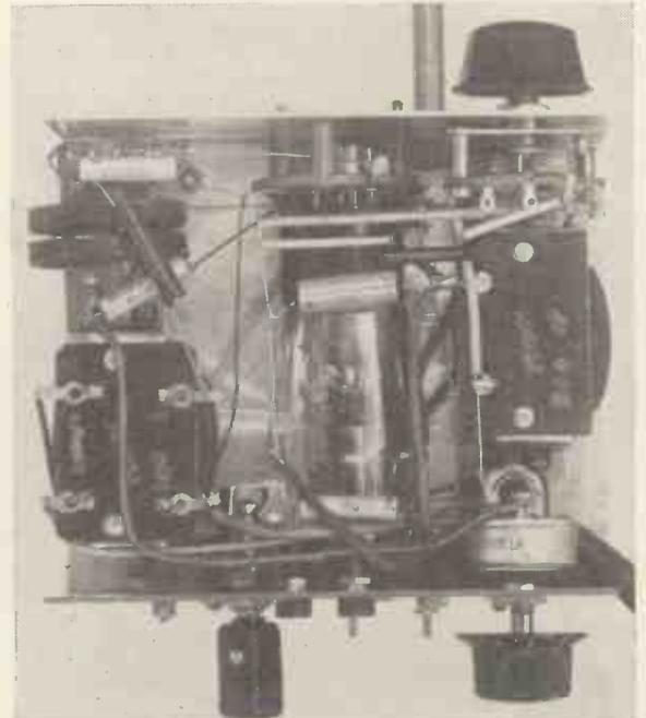
Fig. 4.—Some idea as to the layout can be seen from this view. The pentode modulator is in the centre of the chassis.
