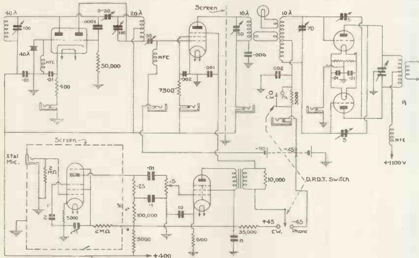
Fig. 4. The ten-metre band has proved its use this year. Here is a straightforward circuit that can be adapted for English valves.
