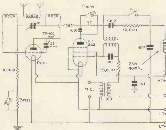
Fig. 5.—A microphone battery has to be connected up externally, but this can be part of the low-tension to save weight. For a microphone we suggest the use of a small carbon type which can be obtained very cheaply. This type of microphone also gives a high output.
