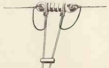
Fig. 7.—This is the way the feeders should be connected to the insulator in the centre.
