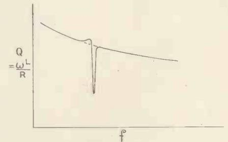
Fig. 4.—Sudden variation in  $Q$  of coil due to coupling with nearby coil.
