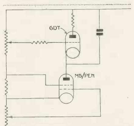
Fig. 3.—Another successful method of providing a continuous variation of sweep.
