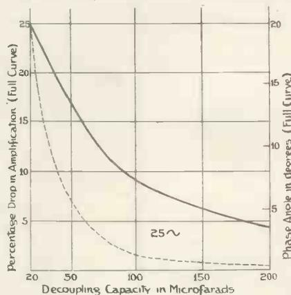
Fig. 6.—Second method, using screen grid valve (same as in Fig. 4):  $R_v = 500,000$ ,  $R_1 = 20,000$ ,  $R_3 = 100,000$ ,  $R_2 = 500$ ,  $\mu = 1,000$ .
