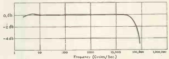
Fig. 34. Frequency response curve of Marconi television amplifier.
