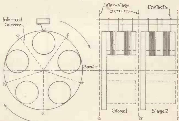
Fig. 5.—Turret principle of coil changing.
