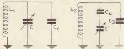
Fig. 1.—A signal frequency circuit and a conventional oscillator circuit.
