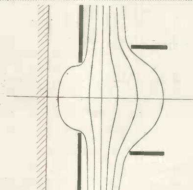
Fig. 2. Electron lens consisting of aperture and cylinder.
