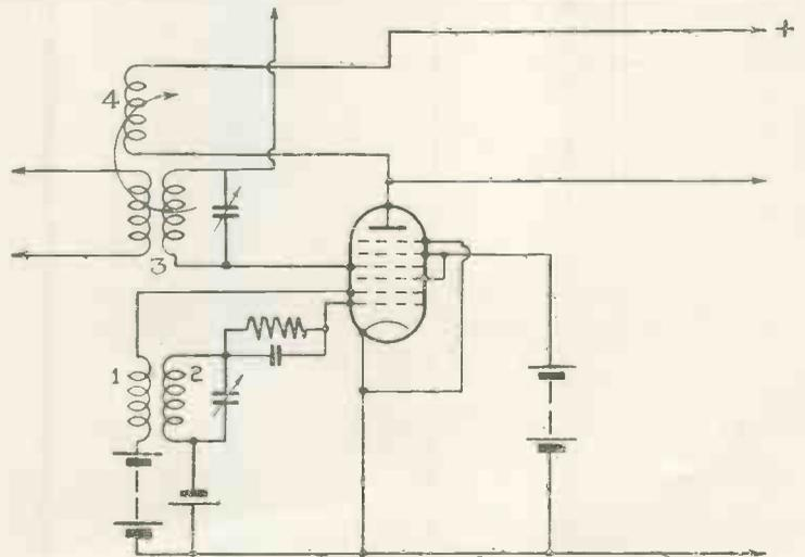
and fifth grids are connected together. A virtual cathode is formed near the third grid, and supplies electrons to the upper part of the valve
