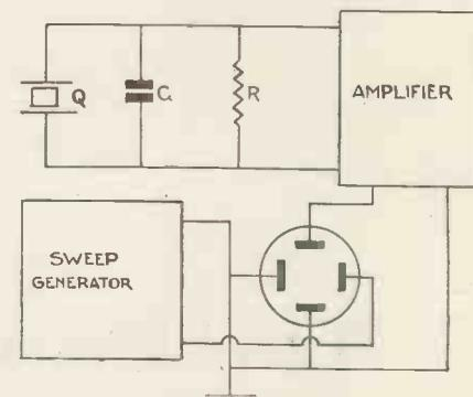
*A simple circuit for using the tube as an engine indicator.*
