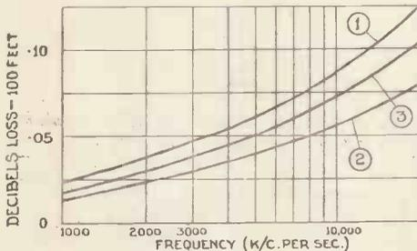
Fig. 1.—This curve shows Loss versus Frequency. (1) for 12-gauge copper wire at 600 ohms. (2) for 1/4-in. copper tube at 300 ohms. and (3) 1/4-in. aluminium tube at 300 ohms.
