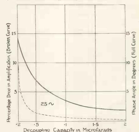
Fig. 3.—Showing effect on amplification and phase angle of different values of decoupling capacity for typical circuit with following constants:  $R_v = 10,000$ ,  $R_1 = 20,000$ ,  $R_2 = 1,000$ ,  $\mu = 30$ .
