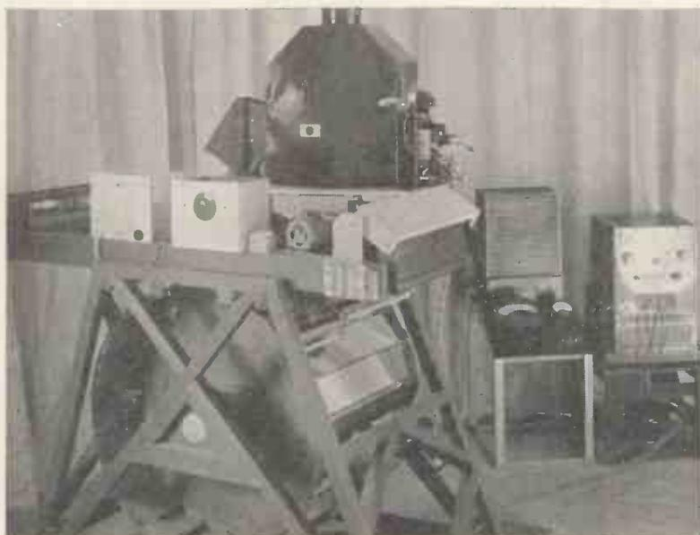
The big screen television projection apparatus. This apparatus is capable of projecting a 240-line picture on to the 13 ft. by 10 ft. screen, with adequate brilliance and can be focused to a still larger picture.
