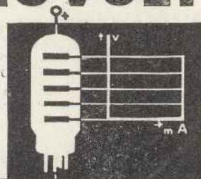
The Stabilovolt tube is a voltage-dividing potentiometer and voltage regulator. The voltages tapped are independent to a precision of about .1% from the supply voltage variations, 1-2% from the varying current intensities tapped, .01% from one another. Currents up to 200 mA, voltages of unlimited values subdivided into parts of 70 volts each. Light in weight, small in size, simple and safe in operation.
