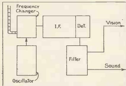
*With this circuit the frequency changer, oscillator, I.F. amplifiers and second detectors are all used both for reception of vision and sound. The filter after the second detector splits the vision and sound signals and feeds them into separate L.F. amplifiers*
