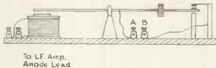
Fig. 2.—The relay may be home constructed on these lines.
