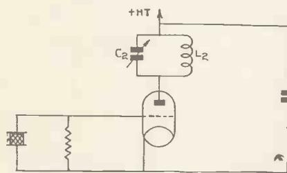
Fig. 2.—A simple crystal control circuit.
