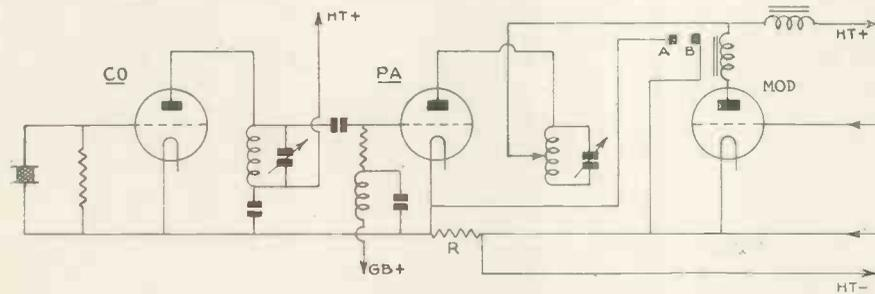
Fig. 1.—This is a typical transmitter showing just how the relay is connected as described by the author. We can recommend this arrangement for all types of transmitters up to 10 watts input.
