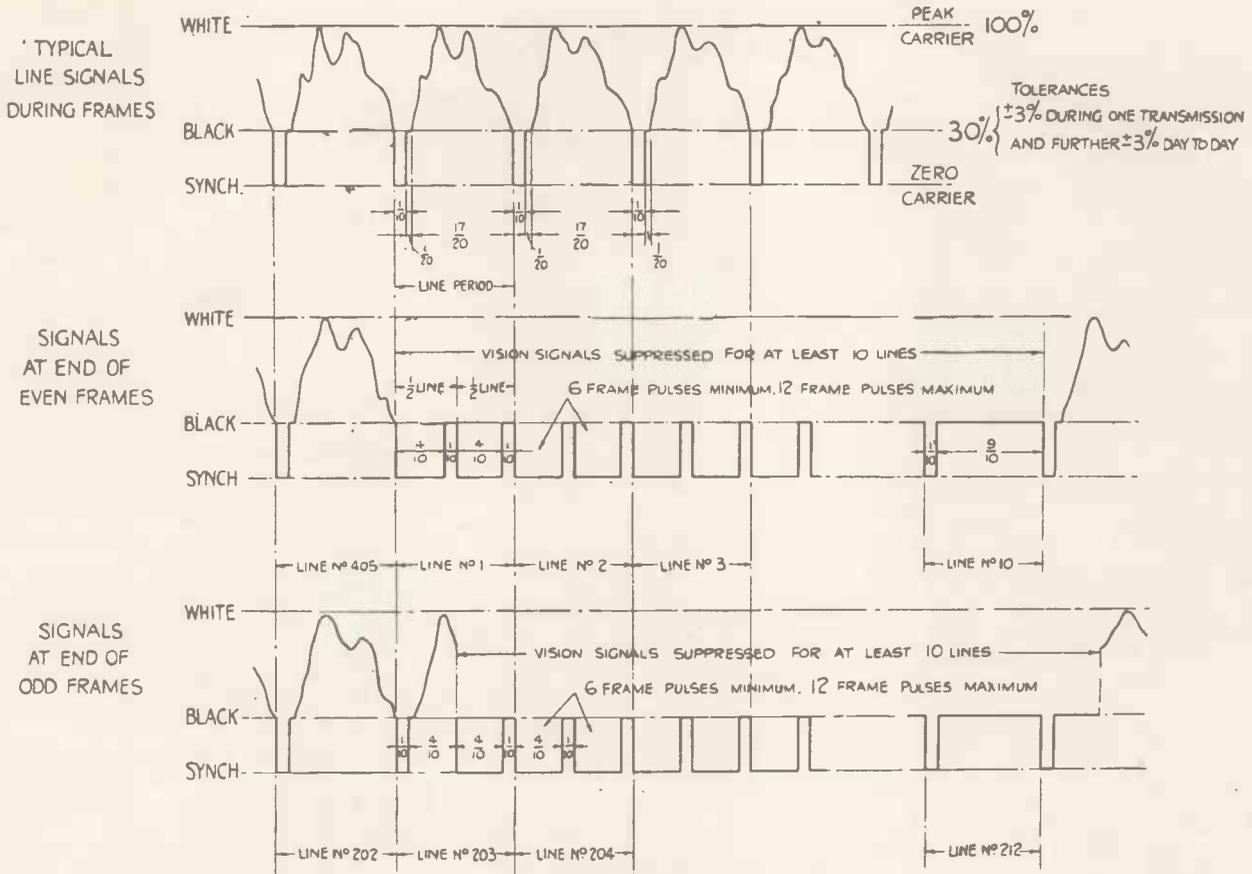
Fig. 4.—The E.M.I. waveform.
