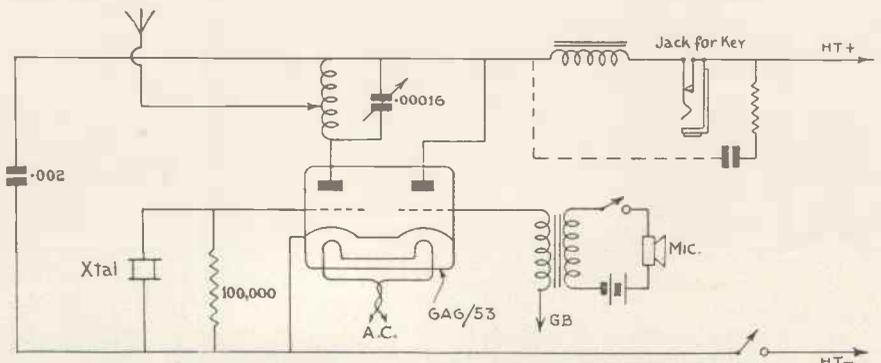
Either a 6A6 or a 53 type valve can be used. Full modulation cannot be obtained unless the microphone is of the carbon type giving a high output. There must be at least 4 volts across the secondary of the microphone transformer.
