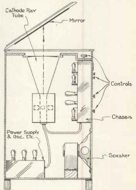
Diagram showing the general scheme of the R.C.A. receiver.
