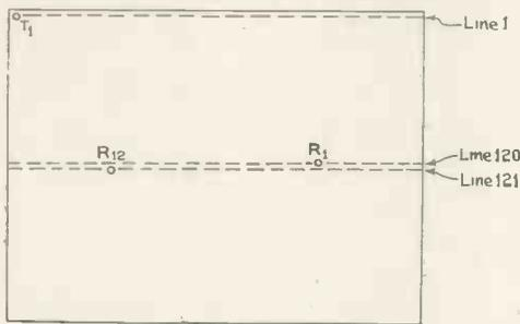
Fig. 2.—Showing the relative positions of spot and synchronising impulse.
