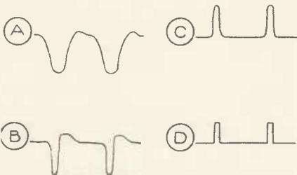
Method of producing synchronising impulses. Patent No. 443,032.
