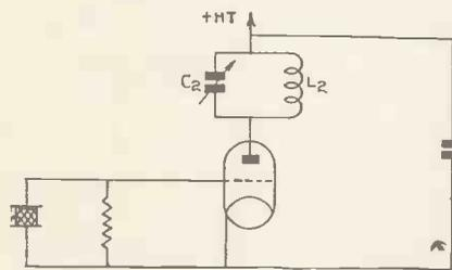
Fig. 2.—A simple crystal control circuit.
