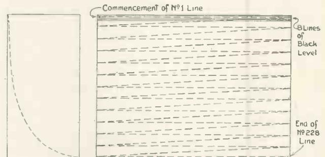
Fig. 3.—Fly-back of Baird's old 30-line system (left) compared with that of their modern 240-line system. No attempt has been made to draw any line scanning line. It must not be overlooked that the old system was designed for mechanical receivers.
