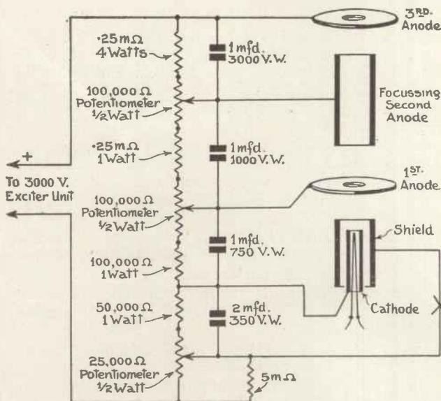
Resistance and condenser network for cathode-ray tube.
