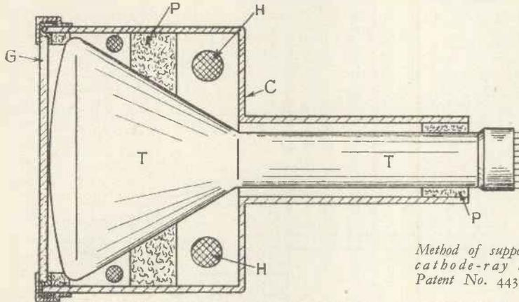
Method of supporting cathode-ray tube Patent No. 443,484.
