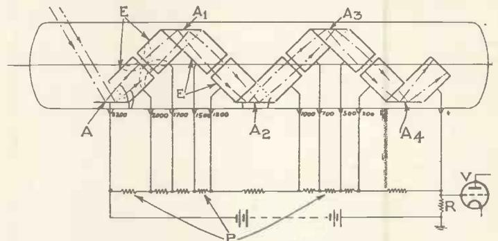
An electron multiplier system. Patent No. 443,777.
