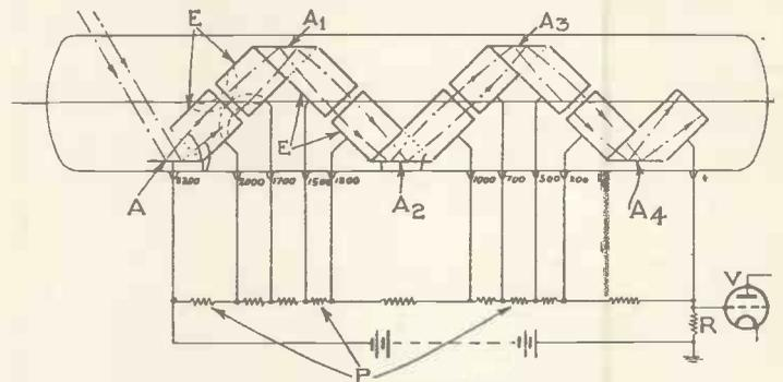
An electron multiplier system. Patent No. 443,777.
