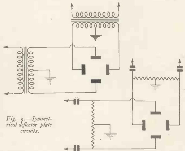
Fig. 3.—Symmetrical deflector plate circuits.
