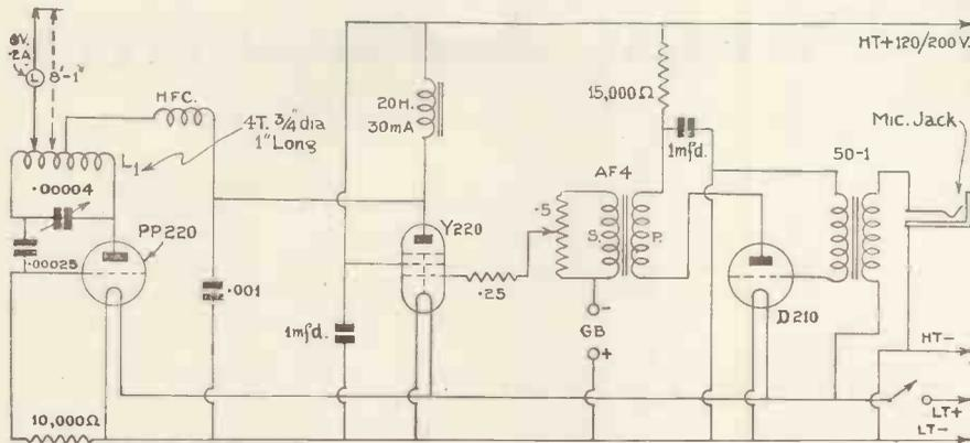
Only three valves are used, two in the modulator-speech amplifier section and one as an ultra audio oscillator.
