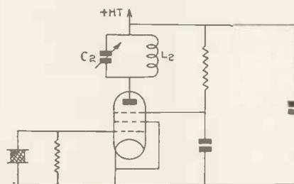
Fig. 3.—A pentode oscillator gives greater output.
