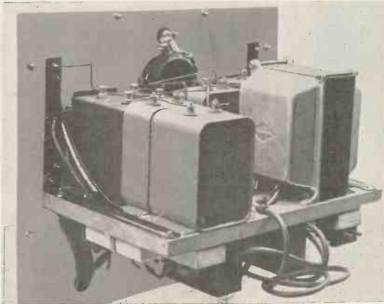
*The large condensers and mains transformer are mounted on a solid wooden baseboard. Under the baseboard are the smoothing chokes, power resistances and fuse plug.*
