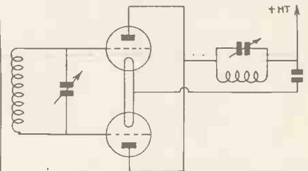
Fig. 4.—Push-pull oscillators have the anodes strapped in this way.
