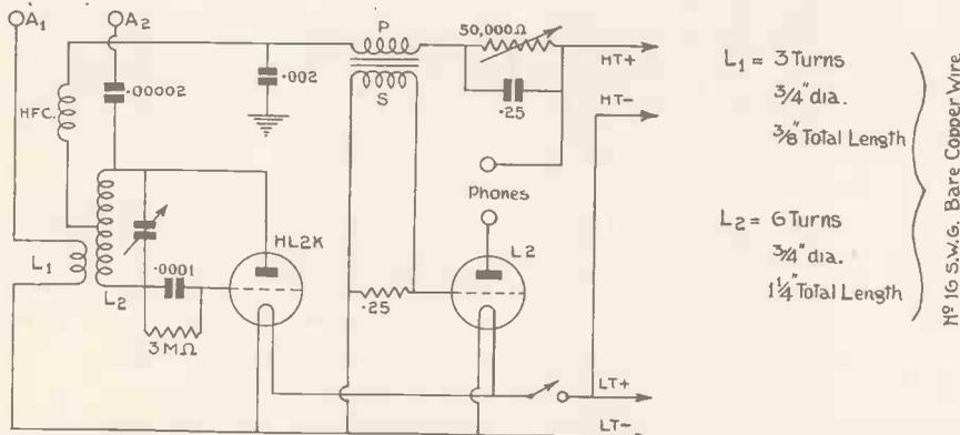
By connecting the grid return to a point at high potential the efficiency is increased and noise reduced by at least 25 per cent.
