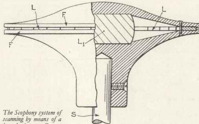
The Scophony system of scanning by means of a lensed ring. Patent No. 443,393.
