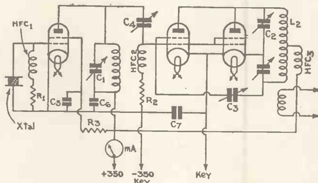
Adjustments should be made in the following manner. Tune C<sub>2</sub> for minimum plate current after first adjusting C<sub>1</sub> for maximum grid current with the anode voltage off. Then couple the aerial inductively to L<sub>2</sub> and load up as much as possible without the HF300 showing any suggestion of colour during keying. Primary keying was used
