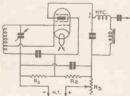
Fig. 3.—Regeneration is very important in straight receivers. Try this arrangement for it is smooth and does not introduce modulation hum.
