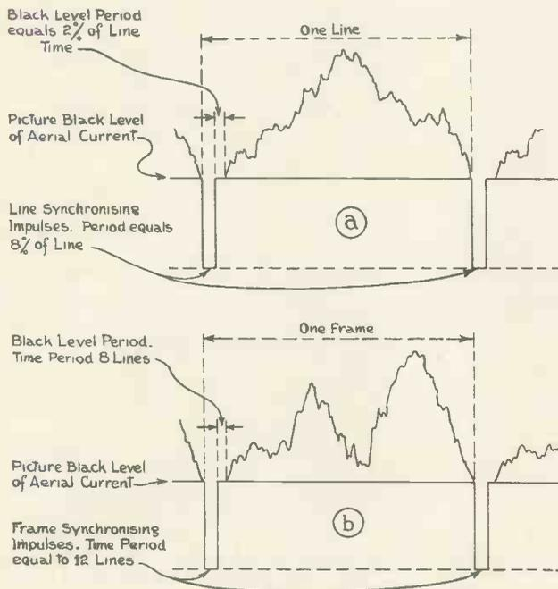
Fig. 1.—Details of waveform used in the Baird system.
