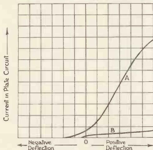
Fig. 4.—Graphs showing effect of input impedance to deflector plates.
