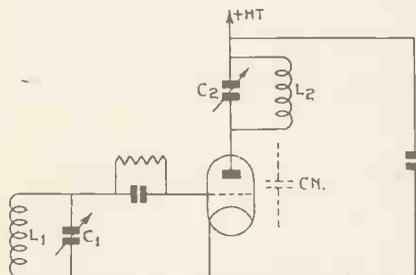
Fig. 1.—The tuned-grid tuned plate circuit.
