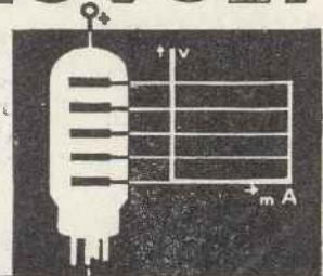
The Stabilovolt tube is a voltage-dividing potentiometer and voltage regulator. The voltages tapped are independent to a precision of about .1% from the supply voltage variations, 1-2% from the varying current intensities tapped, .01% from one another. Currents up to 200 mA, voltages of unlimited values subdivided into parts of 70 volts each. Light in weight, small in size, simple and safe in operation.
