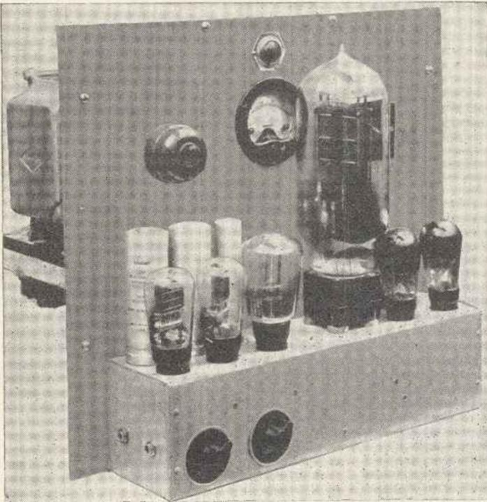
*All of the small components in the amplifier are mounted within the valve rack. In this way connections are kept short and hum pick-up reduced to a minimum.*
