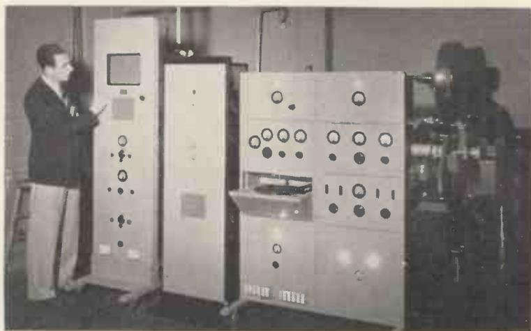
*One of the 240-line film transmitters in operation. Mr. J. Sieger is at the controls of the control receiver. This receiver projects a picture of 240-lines definition on a flat screen 10 in. by 8 in. using only a talkie exciter lamp as light source. The brightness is sufficient to see the picture with all the lights on in the transmitter room.*
