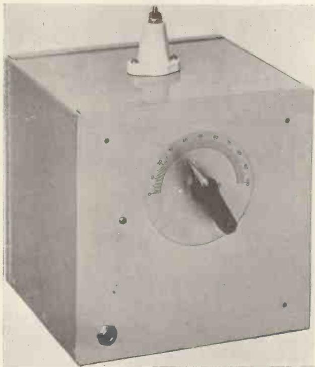
*The plug in the left-hand corner is for the microphone while the stand-off insulator is connected to the coil in anode circuit of the 6A6. Unless the correct tapping point on the coil is obtained efficiency will be greatly decreased.*
