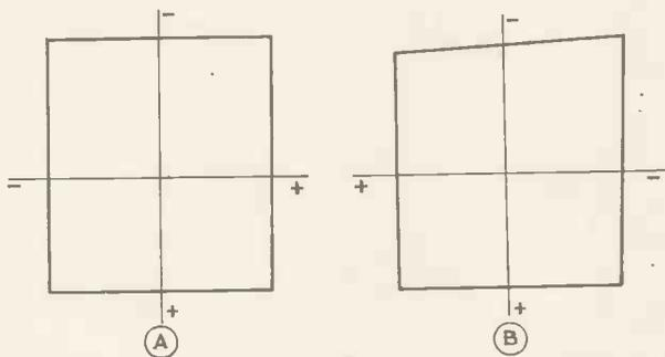
Fig. 2.—Distortion due to variations of sensitivity. A—one pair of plates. B—Two pairs of plates.
