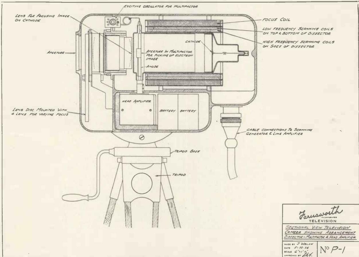
*This is a reproduction of the working drawing of the camera produced in the Farnsworth laboratories.*
