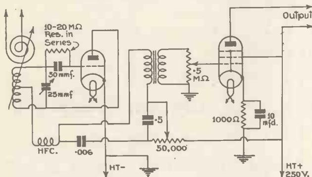
Fig. 1.—A super-regenerative type of receiver of this kind is claimed to be very free from background noise.
