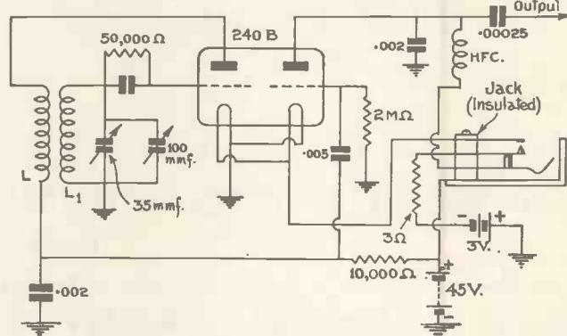
Fig. 2.—The 240B valve is most suitable for this circuit as it oscillates very freely.
