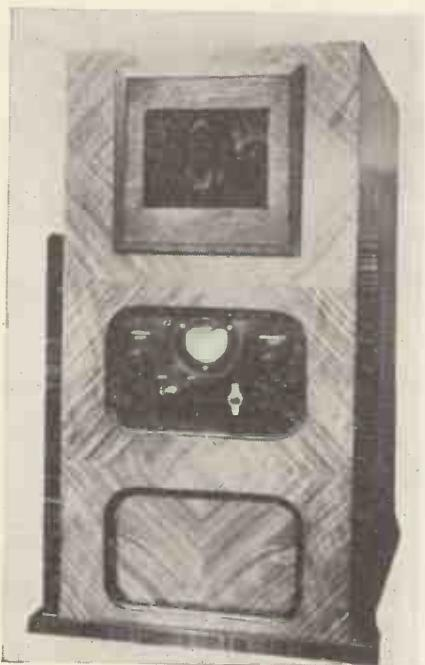
*An experimental cathode-ray receiver designed in the Furzebill Laboratories.*
