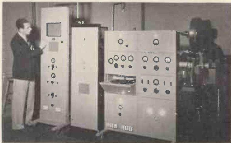
*One of the 240-line film transmitters in operation. Mr. J. Sieger is at the controls of the control receiver. This receiver projects a picture of 240-lines definition on a flat screen 10 in. by 8 in. using only a talkie exciter lamp as light source. The brightness is sufficient to see the picture with all the lights on in the transmitter room.*
