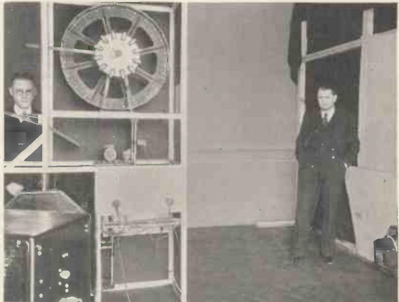
*The Medium-screen Demonstration Receiver on the left, showing the low-speed scanner. This apparatus projects a picture 5 ft. by 4 ft. on to the screen, part of which is shown on the right. Mr. G. Wickenhauser, is standing next to the screen.*
