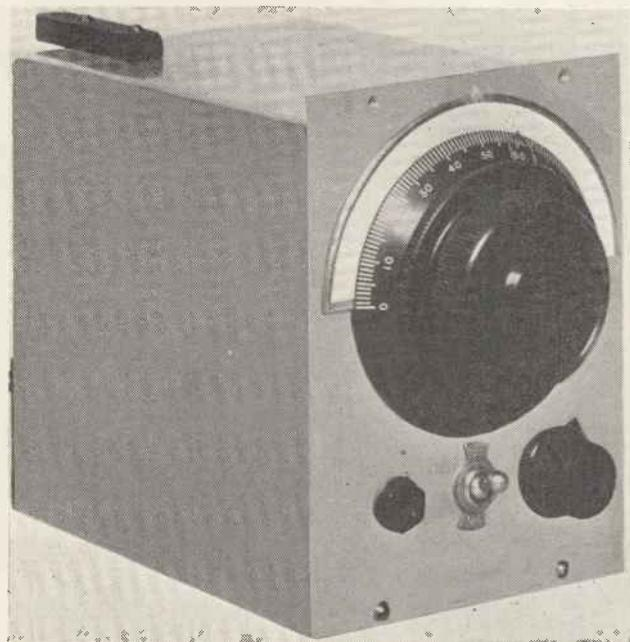
*The controls are; left, phone jack; centre, on/off switch; right, volume control. The tuning dial in the receiver is one of the original Burndept type which can still be obtained but any dial with a good smooth drive can be used.*
