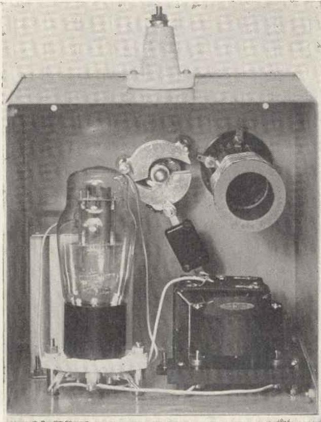
The lay-out of this transmitter can be seen from this illustration. In the foreground is the special Brookes 20 metre crystal. Insulate the tuning condenser from the metal case by means of a large square section of ebonite.
