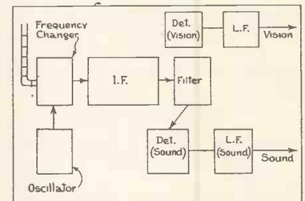
*By having separate second detectors the sound and vision signals can be more accurately separated and amplified to the required amount by entirely separate L.F. amplifiers.*
