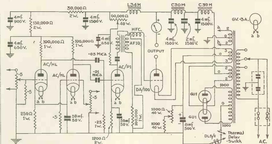
*A useful feature is the inclusion of a split-grid input circuit so that a microphone and pick-up can be used together. One circuit has been arranged to give better response for pick-up work.*
