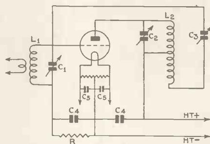
Fig. 5.—This power doubler uses the H.F. 300 but it can be adapted to use other valves of lower wattage if the input capacity is low. We suggest the Ediswan E.S.W.501.
