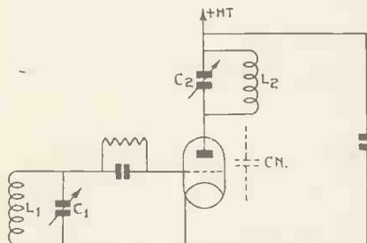
Fig. 1.—The tuned-grid tuned plate circuit.
