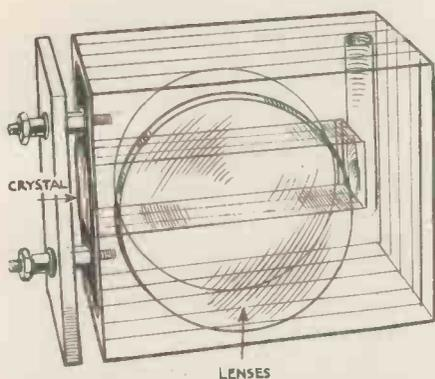
Fig. 7 (above) The supersonic light modulating cell merely consists of a glass sided box capable of holding a liquid with a crystal at one end to which the input from the receiver is applied. The owners of the patent for this type of cell are Scopony Ltd. and it is only permissible to use it experimentally.
