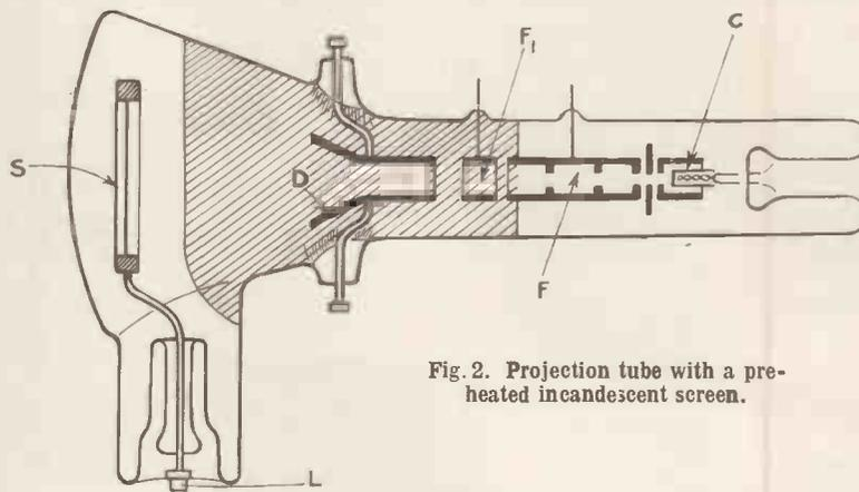
Fig. 2. Projection tube with a pre-heated incandescent screen.
