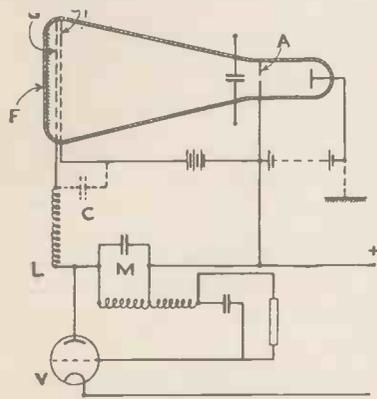
Low-voltage cathode-ray tube. Patent No. 481,917.
