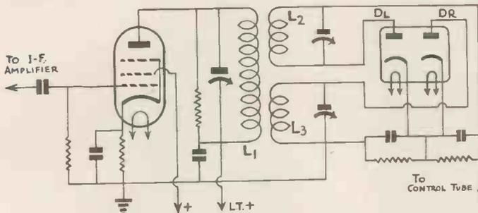
Fig. 1. A frequency discriminator of the simplest type.
