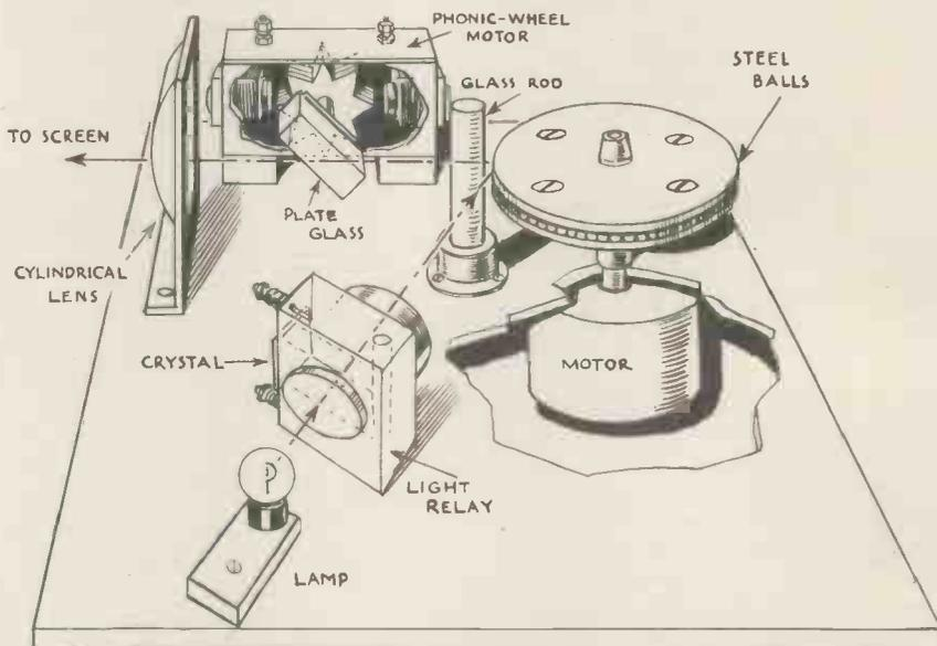
The drawing above shows the complete lay-out of a very simple scanning arrangement shown by the photograph on an earlier page.
