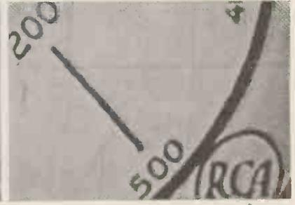
Figs. 2, 3 and 4. Section of the cathode-ray tube screen to illustrate the effect of various receiving aerials on reproduction. The receiver was operated with reduced contrast for best photographic results.
