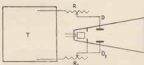
Scheme for adjusting the picture. Patent No. 479,149.
