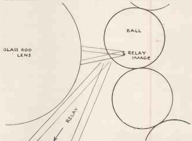
Fig. 8. This drawing shows the incidence of the modulated light on one of the ball units of the scanner.
