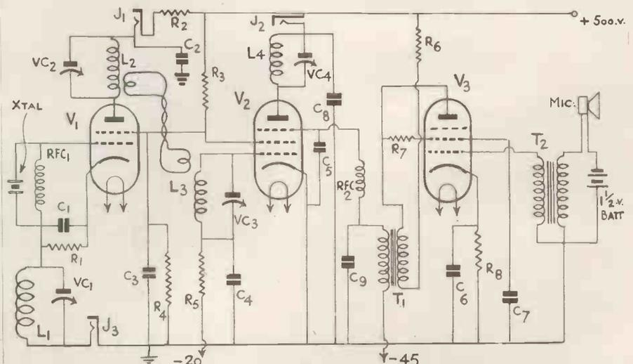
This is the complete circuit of the transmitter complete with single valve modulator. A high percentage of modulation can be obtained providing a carbon microphone is used.
