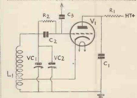
This is the circuit for the complete B.F.O. unit which can be mounted in a metal container or on a breadboard if it is more convenient.
