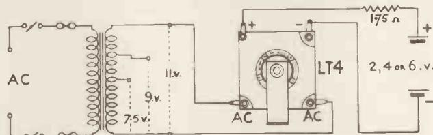
A single or a number of cells can be charged with this unit as fully explained in the text.
