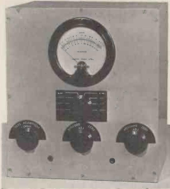
A direct reading meter is used while the various ranges are brought into circuit by means of a multi contact switch.
