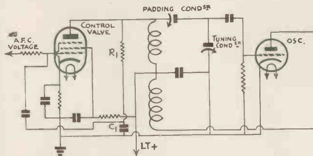
Fig. 3. The out-of-phase voltage in this arrangement is obtained from the condenser  $C_1$ .
