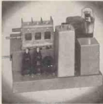
This illustration gives a very good idea as to the construction of the R.M.E. frequency expander. It is similar in appearance to the DB-20 but includes four valves.
