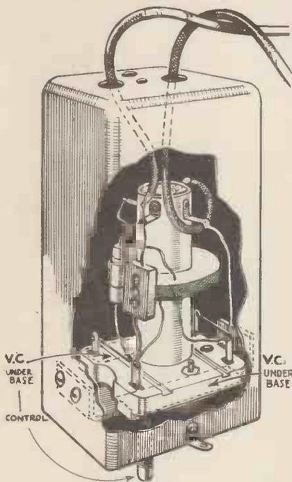
The tuning circuit with its associated condensers and resistors are mounted in a can as shown in this illustration.
