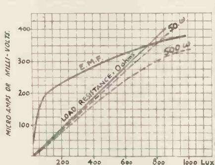
Fig. 4.—Characteristic curve of barrier-layer cell.
