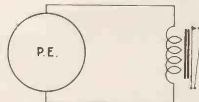
Fig. 7.—A simple light-operated relay.
