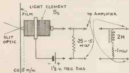
Fig. 8.—Circuit connections of cell used for sound head.
