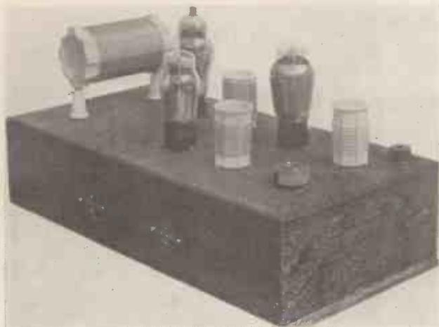
Two valve holders mounted on the back of the chassis are for the high and low voltage supplies. The crystal is mounted in a standard five pin valve holder. In addition, the coil holders with the exception of the final stage are not ceramic but of special hard bakelite.
