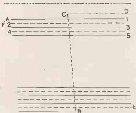
Fig. 1. Diagram explaining the Marconi-E.M.I. system of interlacing.
