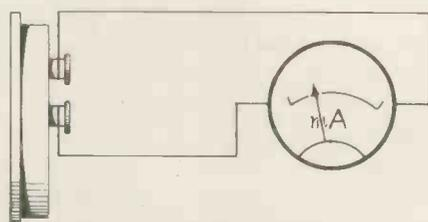
Fig. 5.—Diagram showing construction of photometer.
