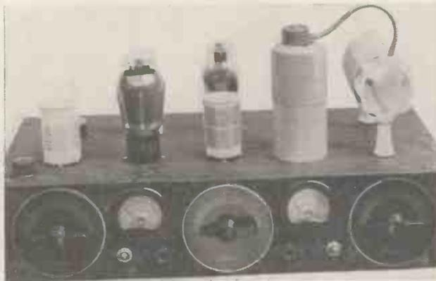
The meters shown are optional for if constructors wish to save expense one meter can be made to monitor the whole transmitter. The 802 valve is completely screened.
