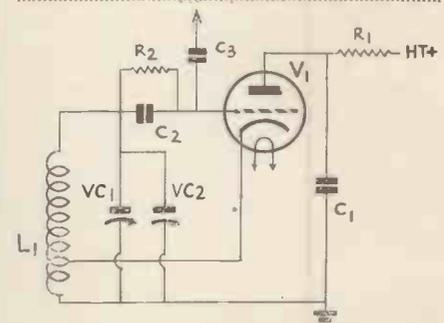
This is the circuit for the complete B.F.O. unit which can be mounted in a metal container or on a breadboard if it is more convenient.
