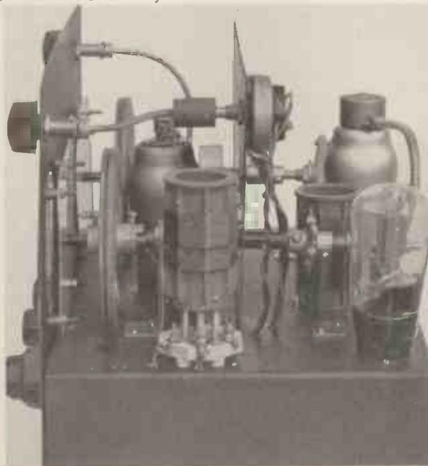
A good idea as to the general construction is obtainable from this view, which shows the aerial coil and output pentode valve.
