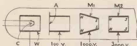
Tube with permanent magnet focusing electrodes. Patent No. 478,410.
