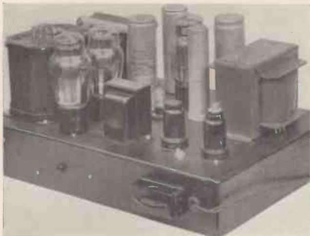
*This simple modulator uses the low voltage high current circuit, so reducing the cost of the components. It gives high quality reproduction and has been designed by G18TS for use at his station.*
