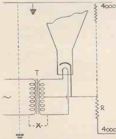
The voltage existing across X is 4,000. With the 6-way plug withdrawn this circuit is removed.
