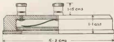
Fig. 1.—Type of cell as used for photometers.
