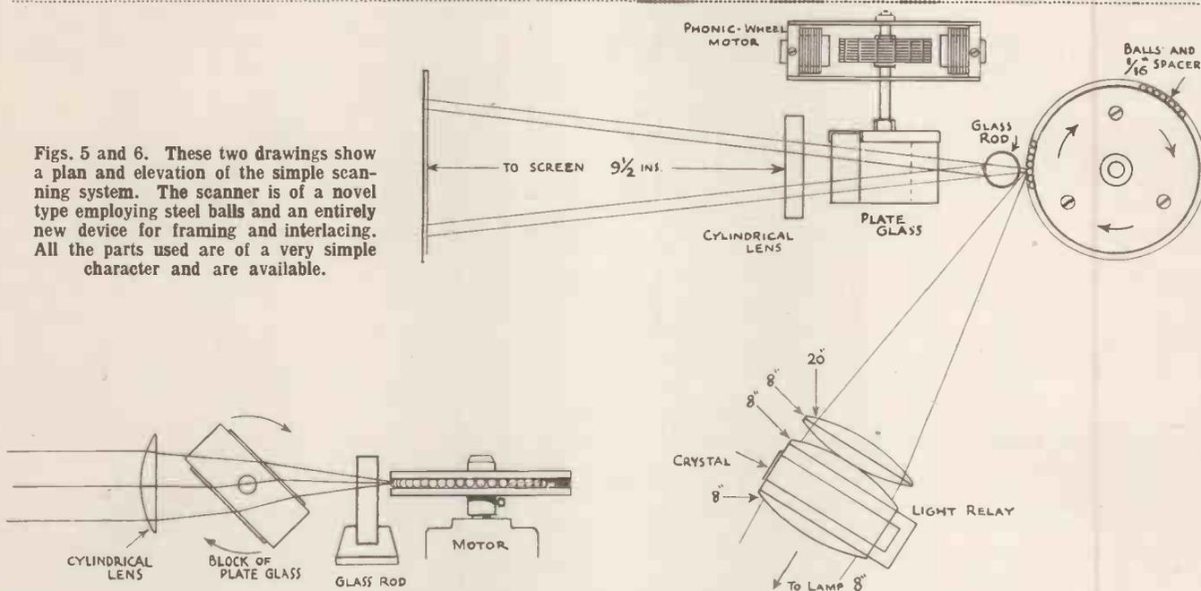
them carry round the image of a train of modulated light details produced in a supersonic wave light relay, we get the basis of an arrangement that can handle a reasonable amount of light.
