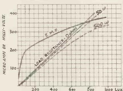
Fig. 4.—Characteristic curve of barrier-layer cell.
