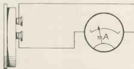
Fig. 5.—Diagram showing construction of photometer.
