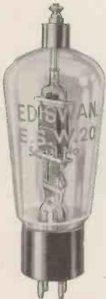
Believing that the British Amateur Transmitter would prefer to use valves of home origin the Ediswan Co. have produced the first medium power transmitting valve at a price within the reach of all pockets.
