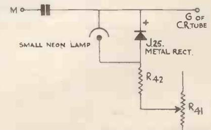
Using a metal rectifier to restore the D.C. component.
