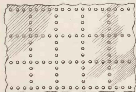
Fig. 1. Incandescent screen with perforations to localise the heat.
