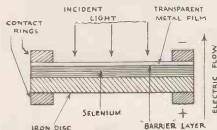
Fig. 3.—Diagram showing construction of barrier-layer cell.
