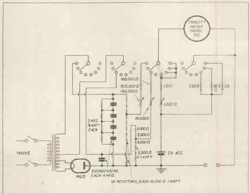
Here is the circuit diagram of the continuity tester with the majority of the component values. A 0-1 mA meter can be used in place of the meter less suggested as explained in the text.
