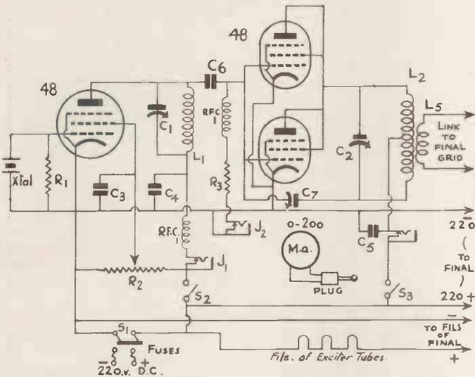
Fig. 4. This interesting D.C. transmitter circuit is suitable for an input of 50 watts.
