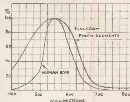
Fig. 9.—Colour sensitivity curve.
