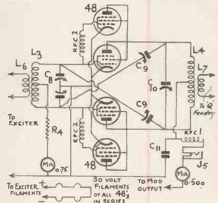
Fig. 5. This type of output circuit is quite easy to operate if precautions are taken as explained in the text.
