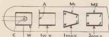
Tube with permanent magnet focusing electrodes. Patent No. 478,410.
