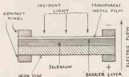
Fig. 3.—Diagram showing construction of barrier-layer cell.
