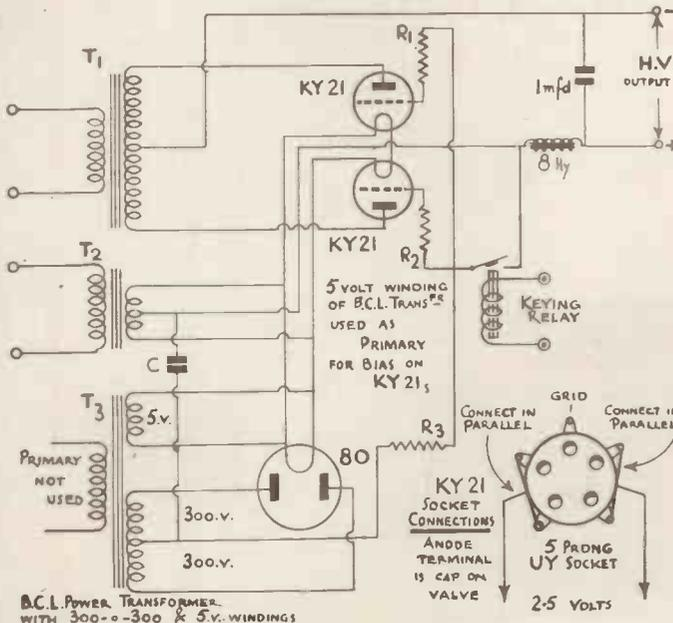
For the C.W. man the keying rectifier offers a new system of clickless keying which has great possibilities. The valves and other equipment needed are now available in this country.
