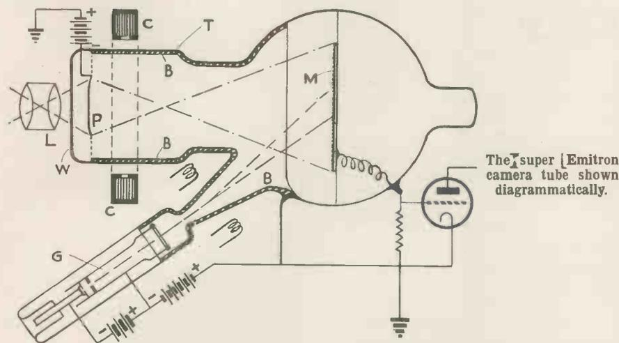
The super Emitron camera tube shown diagrammatically.
