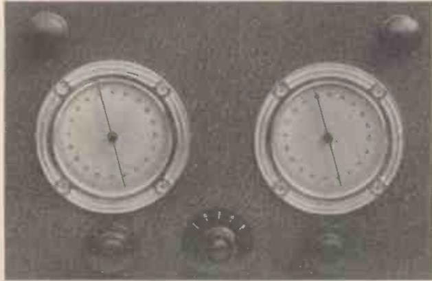
The appearance of this receiver is exceedingly good, while the tuning dials used have a very smooth slow-motion drive arrangement. The switch in the centre is for the wave trap circuit.
