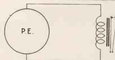
Fig. 7.—A simple light-operated relay.
