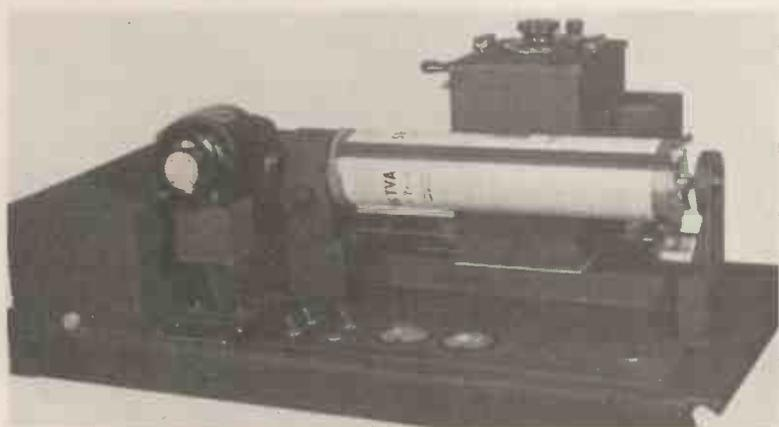
The facsimile transmitter scanner. Pictures, text or drawings are placed directly on the roller drum, the speed of which is synchronised with the receiver-printer in the home.
