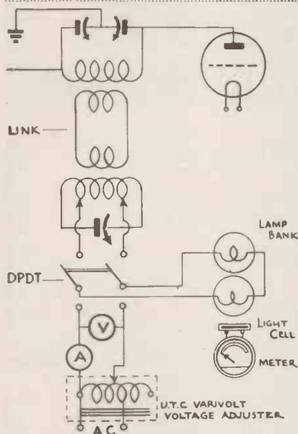
This comparative method of checking R.F. power is a simple method that is most useful to the amateur.
