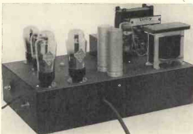
This method of construction allows the experimenter to build an amplifier having quite a professional appearance. The output valves are of a special type with high heater currents in order to minimise hum level.
