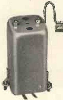
S.W. AIR TRIMMER. A compact trimmer condenser with capacity variation of 1-30 mmfd. Finely graded control and constant setting. No. 1100, 1/3d.
