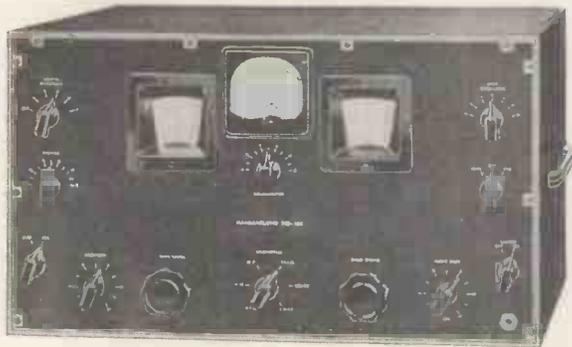
This HQ-120 is the latest receiver to be offered to amateurs by the Hammarlund Company. It includes a very special calibrated R meter and 12 valves.
