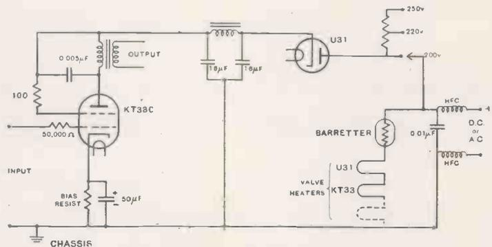
Typical circuit for KT33C in output stage of DC/AC receiver or amplifier, showing heater connections.
