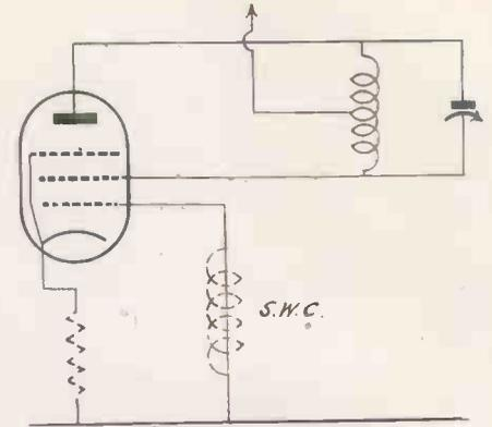
Fig. 4.—Hartley resonant circuit.
