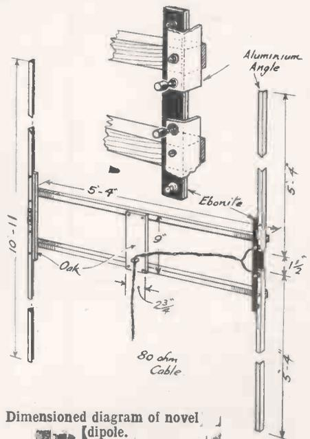
Dimensioned diagram of novel dipole.
