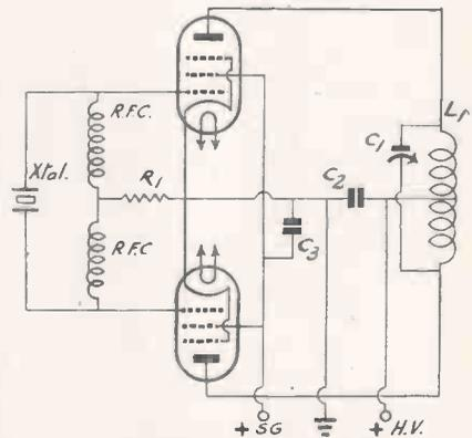
Fig. 3. Push-pull pentode oscillator.
