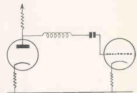
Fig. 8.—Series correcting inductance.
