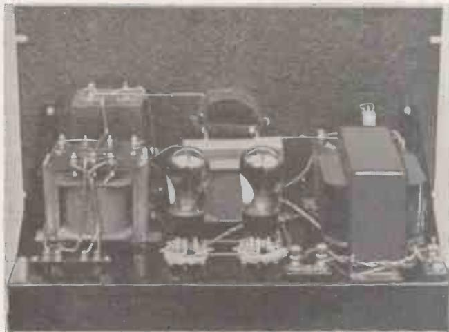
The power unit uses two GU1's and provides 1,000 volts D.C. For lower inputs a 500-volt transformer would be satisfactory with a type 83 full-wave rectifying valve.
