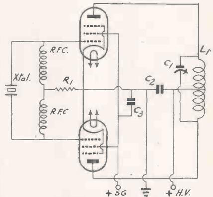
Fig. 3. Push-pull pentode oscillator.
