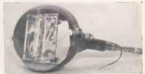
Fig. 11. (right) Camera pick-up tube.
