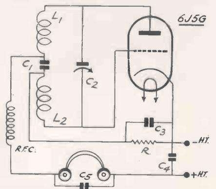
Fig. 3.—The receiver need be only made up of one valve in this way.
