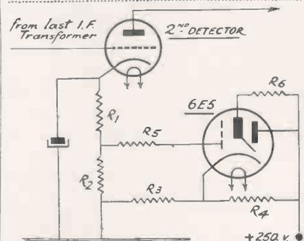
Fig. 2. The tuning indicator with triode detector.
