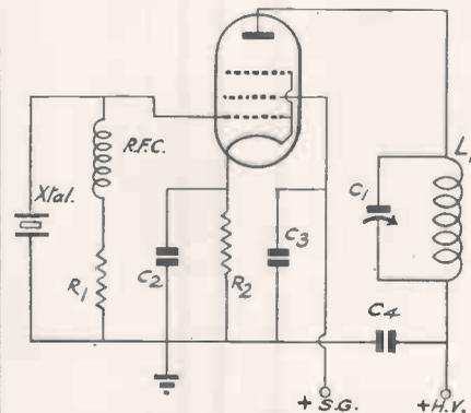
Fig. 2. Standard pentode crystal oscillator.
