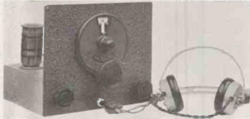
The left-hand control is the band-set condenser, and the right-hand control a 50,000-ohm potentiometer in the reaction circuit.
