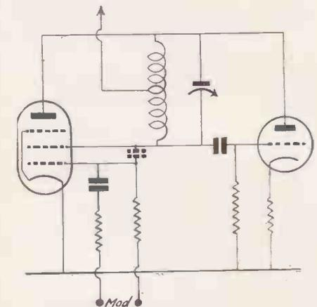
Fig. 5.—Modulated oscillator with sustaining valve.
