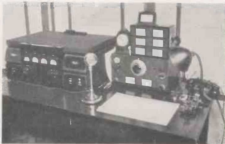
**W9DXX** has invested in one of the new Hallcrafters HT1 transmitters, which gives 75 watts on telephony and over 100 watts on C.W.
