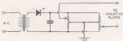
Fig. 1 (left). Half-wave rectifier for picture shift circuit.
