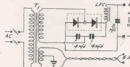
A metal rectifier is used in the power unit and here is the circuit.
