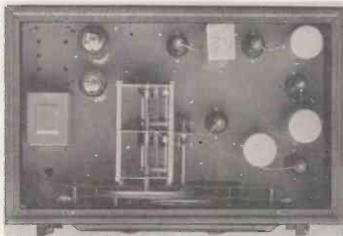
Most of the small components are underneath the chassis so leaving the receiver clean in appearance. Notice the small two gang band spreading condenser alongside the main unit.
