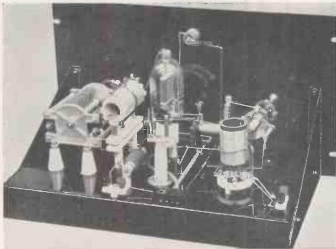
This illustration gives a very good idea as to the layout of the components. Notice how the tank condenser and coil are mounted well away from the chassis.
