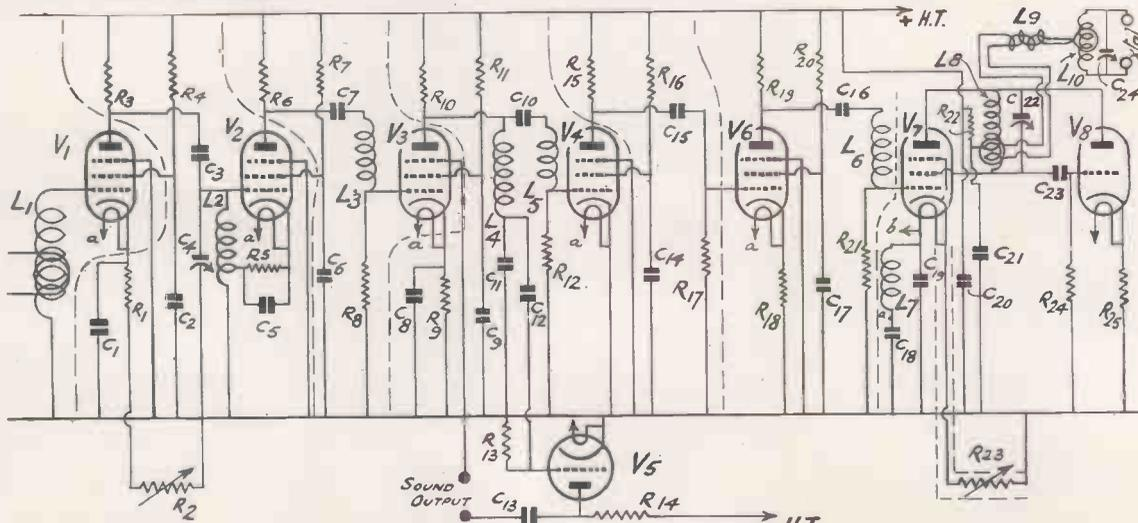
The complete circuit of the radio receiver for mechanical television.
