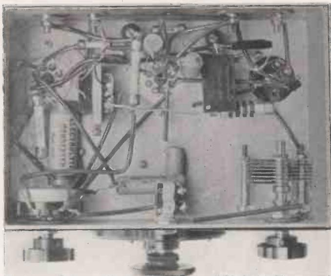
Most of the small components are connected under the chassis as shown in this illustration. Notice the midjet inter-valve transformer.
