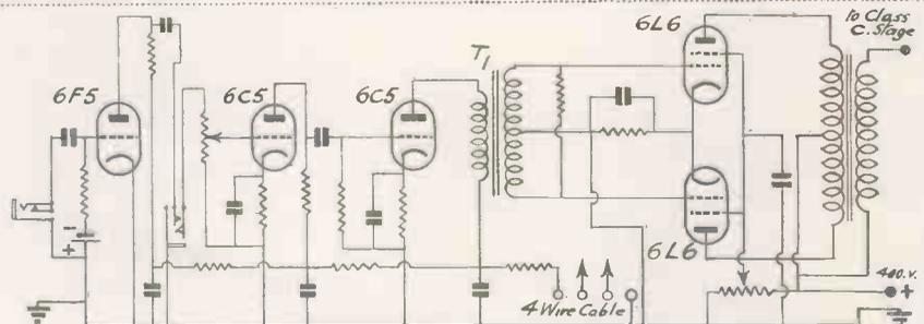
Fig. 5. Over 20 watts of audio are obtainable from this modulator.
