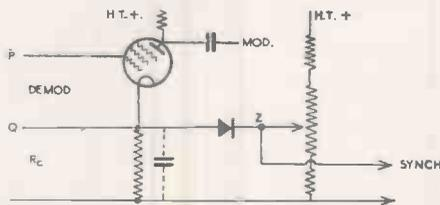
Fig. 4. Typical synchronising filter circuit in which it is necessary to insulate both sides of the input from earth.
