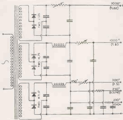
Fig. 3 (left). Complete high-tension power pack for combined vision-sound receiver, time base, cathode-ray tube and picture-shift.
