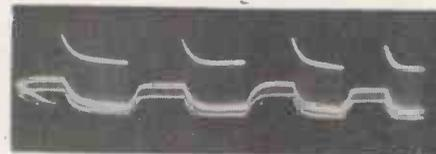
Oscillogram taken at grid of C.R. tube of the same 50-cycle signal. This illustrates a faulty D.C. restoration circuit. If this section is functioning correctly the trace should appear as on the left.
