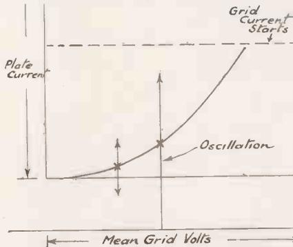
Fig. 3a.—Grid modulation of oscillator.
