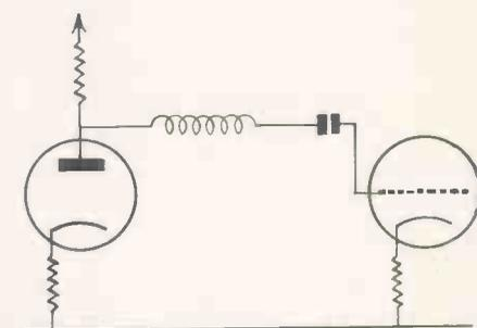
Fig. 8.—Series correcting inductance.
