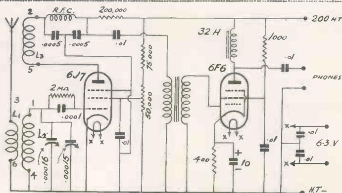
The coils have been numbered in order that constructors will connect them the correct way round in order to obtain maximum gain and reaction.
