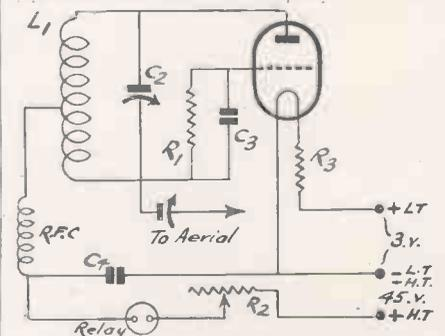
Fig. 3. Remote control circuit with gas-filled triode.
