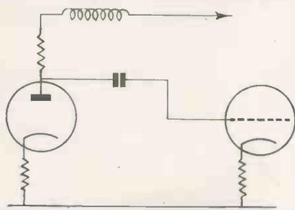
Fig. 7.—Conventional correcting inductance.
