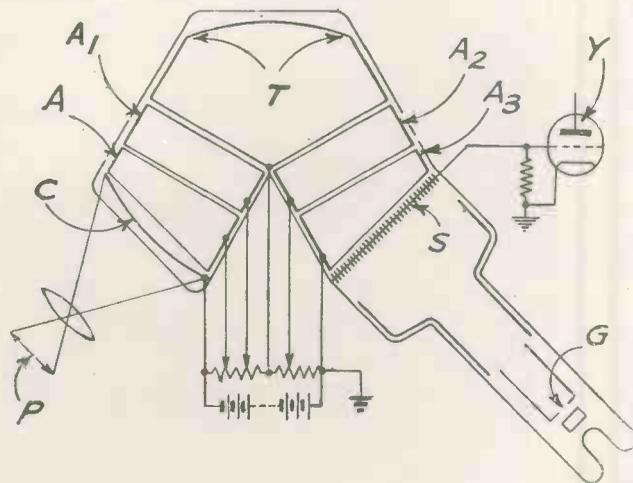
Electron multiplier transmitter tube. Patent No. 497,406.
