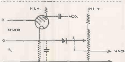
Fig. 4. Typical synchronising filter circuit in which it is necessary to insulate both sides of the input from earth.
