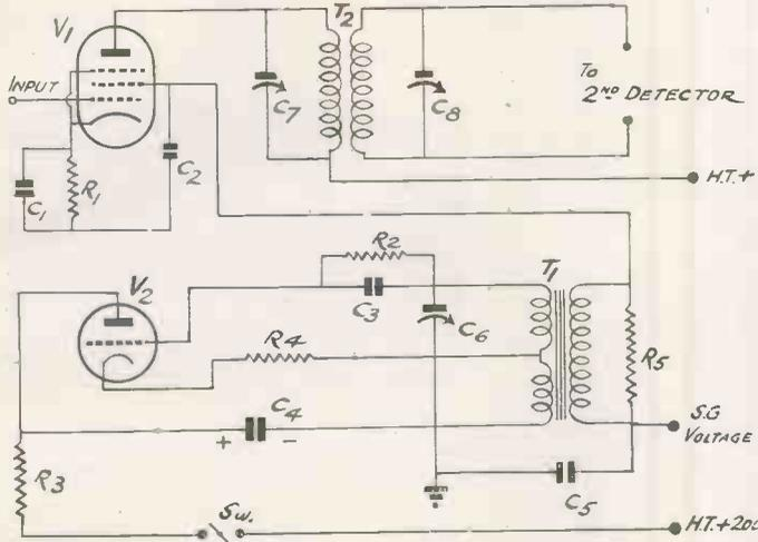
A circuit of an audio oscillator suitable for heterotone reception is quite simple. It must be appreciated that the beat-frequency oscillator must also be retained but the only modification to an existing set is to break the screen lead as shown.
