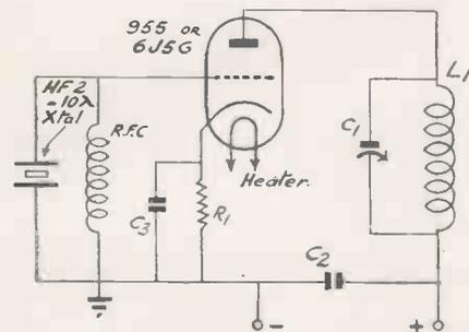
Fig. 1. Triode crystal oscillator, primarily intended for 28 mega-cycles.
