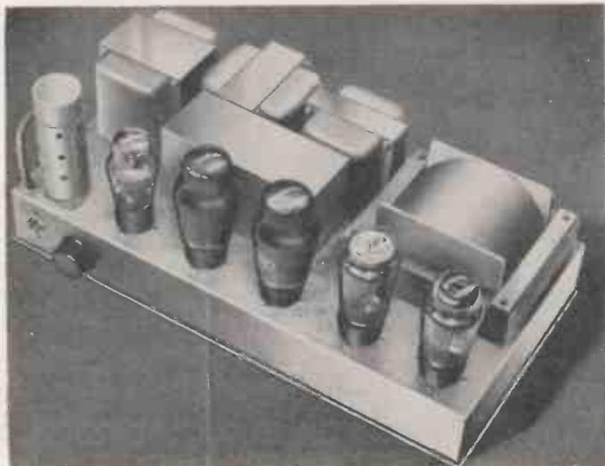
The new Savage high-fidelity amplifier has a gain of 96 DB and a noise level of -60 DB. A commendable feature is that the frequency response is within 2 DB from 50 to 10,000 cycles.
