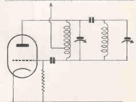
Fig. 2.—Band pass Oscillation Circuit.
