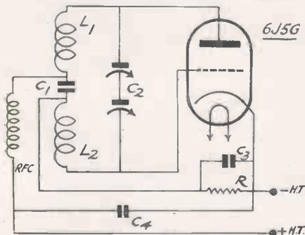
Fig. 1.—A straightforward single valve circuit using the new low capacity triode.
