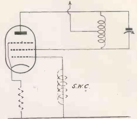
Fig. 4.—Hartley resonant circuit.
