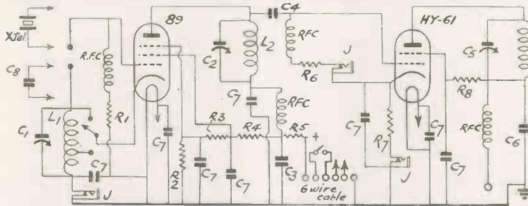
Fig. 4. The input to this transmitter can be increased to 30 watts at 5 metres.
