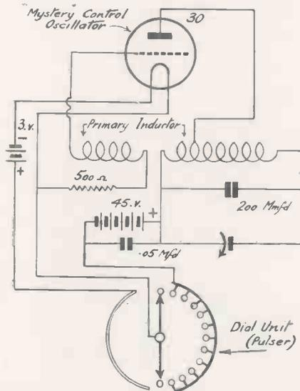
Fig. 1. The Philco remote control arrangement.
