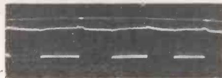
Oscillogram of black cross signal using 50-cycle time base; taken at anode of video stage. A similar trace can be obtained at the detector.
