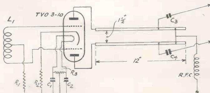
Notice that no condensers are needed in the grid or cathode circuits. It is suggested that the aerial be coupled directly to the tank inductance.
