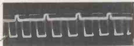
Input. Showing complete line signal on black cross. Signal phase reversed.
