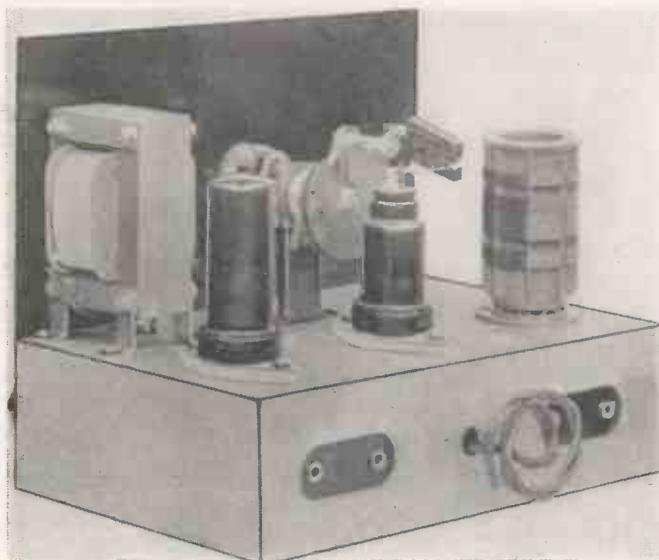
This view of the chassis indicates just how the major components are laid out and shows the sockets for H.T. supply and aerial and earth in addition to the two leads for the heaters.
