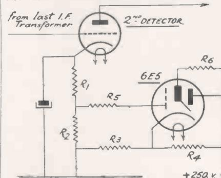
Fig. 2. The tuning indicator with triode detector.
