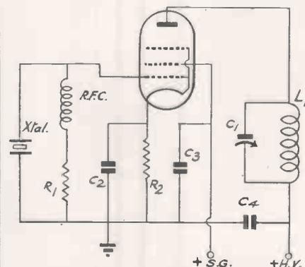
Fig. 2. Standard pentode crystal oscillator.
