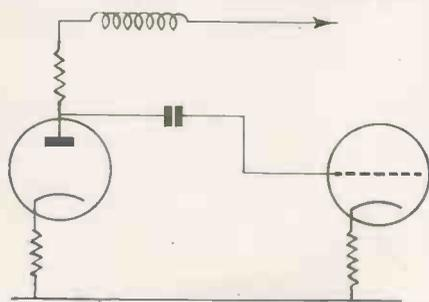
Fig. 7.—Conventional correcting inductance.
