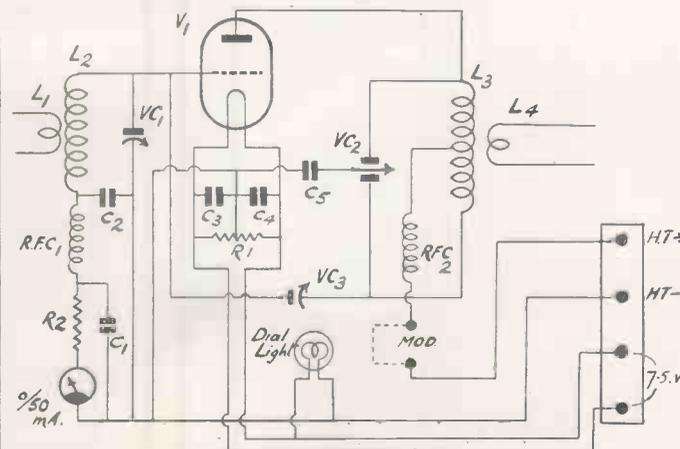
The circuit is a straightforward one but in order to obtain maximum R.F. output the component values should be strictly adhered to. Grid bias is obtained automatically.
