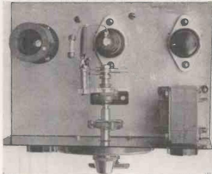
The grid condenser and leak are connected between the grid of the 6J7 and the band-spread condenser.
