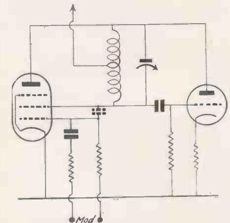
Fig. 5.—Modulated oscillator with sustaining valve.
