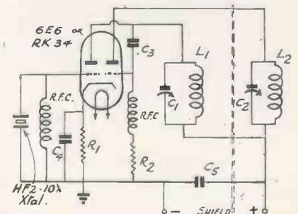
Fig. 8. Double-triode, oscillator-doubler for 5-metre output.
