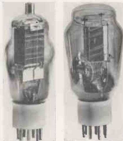
**On the left is the Tungram OS12/500 a valve similar to the 837. An interesting valve is shown on the right—the Tungram 015/600 specially made for 5 metre operation.**
