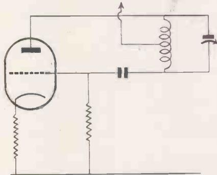
Fig. 3.—Grid modulation oscillator circuit.
