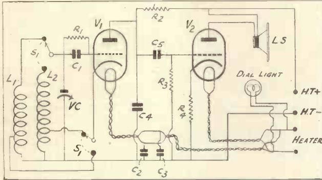
Fig. 2. A suggested two-valve C.W. monitor suitable for feeding a loudspeaker.
