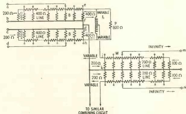
Fig. 7 (above.) Basic mixing circuit.
