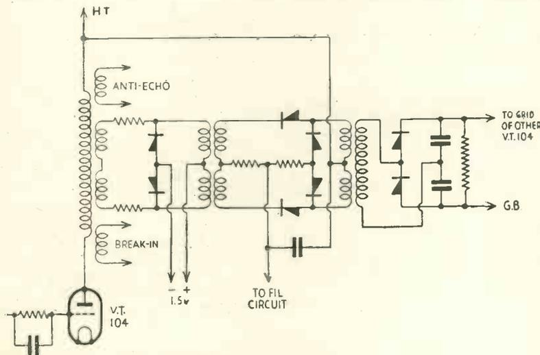
Fig. 3. Section of Post Office stabilised repeater showing three uses of metal rectifiers.
