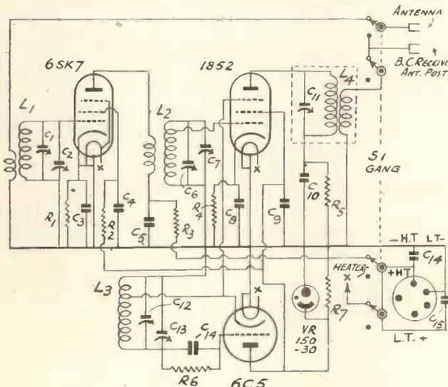
Fig. 4. Two of the latest valves are used in this convertor designed to provide high efficiency on the U.H.F. bands up to about 80 megacycles. Notice also the voltage stabiliser in the oscillator circuit which accounts in a certain degree to lack of frequency drift. A special type of output transformer is also employed.
