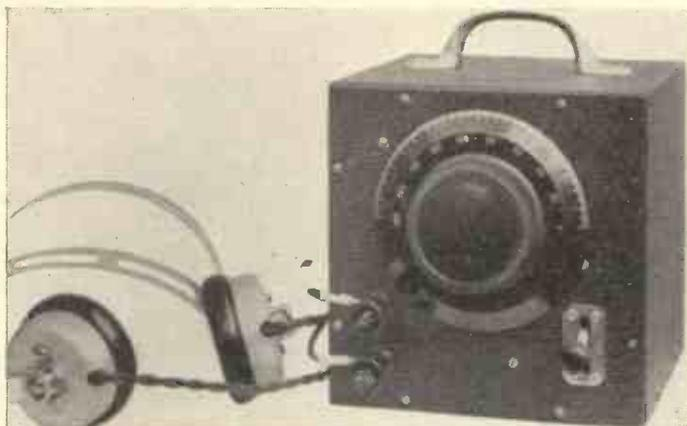
This is the C.W. monitor built in a special Peto-Scott metal cabinet which is only 6 ins. cube.
