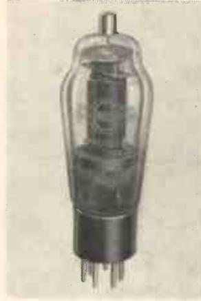
the output is approximately 38 watts. The anode-grid capacity is only 0.1 mmfd. while the total cathode-grid capacity is approximately 16.4 mmfd. This valve is provided with a 6.3 volt heater at which the current is approximately 1.3 amperes. A total emission of 800 mA. is claimed.
