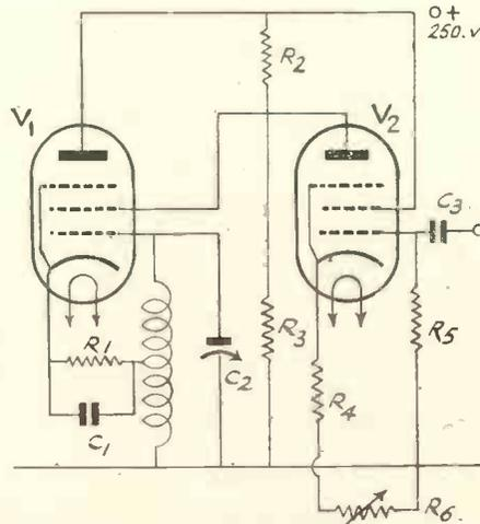
Circuit diagram of modulated oscillator.
