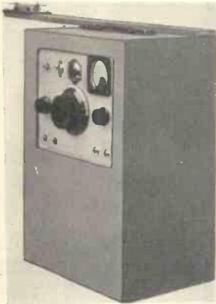
A compass is mounted on the end of a piece of wood so as to keep it well away from the receiver, particularly the moving coil meter, the magnet of which would affect the reading.
