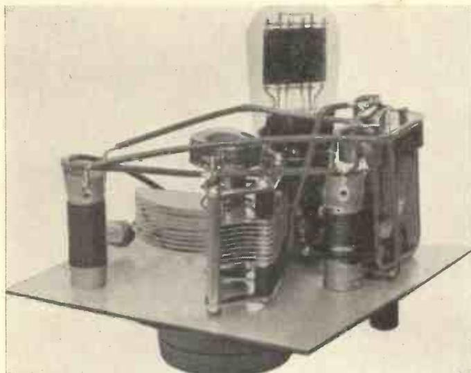
All the components in the C.W. monitor are mounted on the panel. On the left-hand side is the high wavelength coil and on the right-hand side the low wavelength coil. Wiring should be very rigid.
