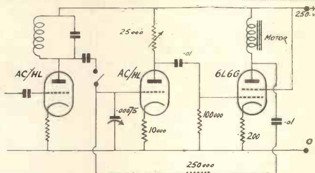
vided from the driver valve plate to the preceding triode grid, and the latter is shunted to earth through a variable condenser. As a result, the pair of valves form, when the motor is connected in circuit, an oscillator of which frequency can be varied over a range of about 1,000 to 10,000 c.p.s. by varying the condenser. The running speed of the motor is 22,500 r.p.m., with 10,125 c.p.s. current, but when fed with, say, 1,000 c.p.s. it
