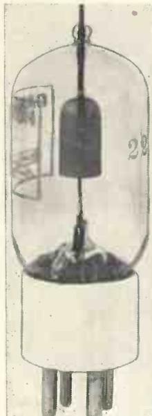
A valve which before very long will be used by most amateurs is the new HK24, a new high-slope triode suitable for U.H.F. working. It has an anode which completely encloses the grid and filament. The heater is 6.3 volts.
