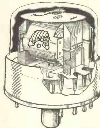
The electrode system is mounted horizontally with a cylindrical grid and anode in this manner.
