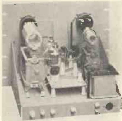
A good example of modern transmitter design is this P.A. stage using a pair of Taylor T-55's in push-pull. It was built for Colonial use and the station is receiving excellent reports from all over the world.
