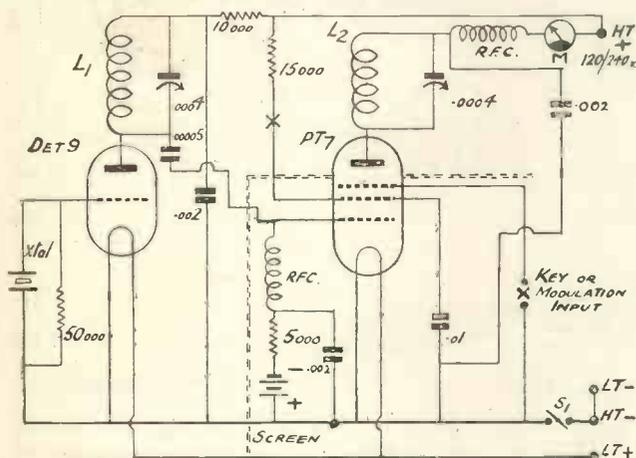
Fig. 1. Battery operated transmitter uses the latest type of Osram two-volt transmitting valve, and the input is restricted to about 3 watts.
