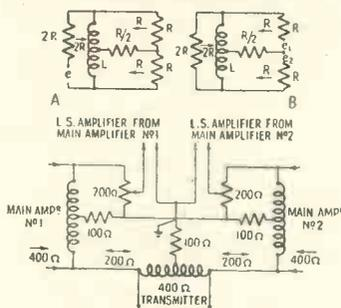
Fig. 9. Basic circuit of output distribution networks.
