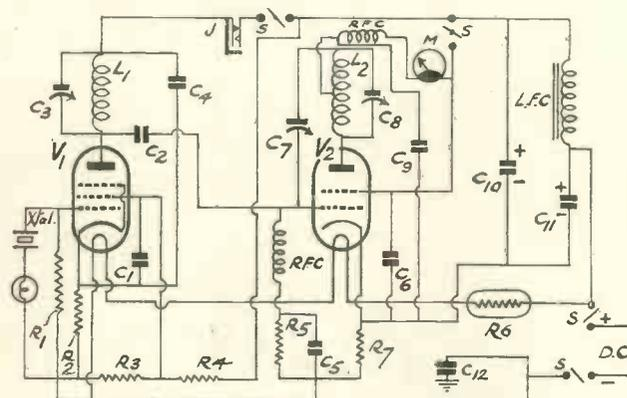
Fig. 5. For those who are limited to operation from D.C. mains this transmitter should prove very serviceable. The output is low but no additional batteries are needed.
