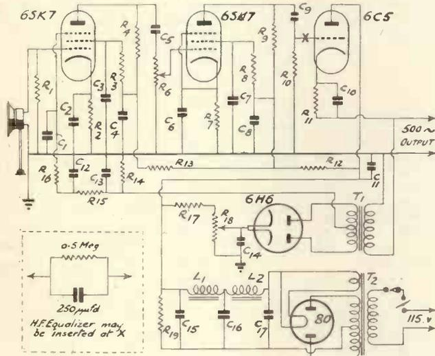
Fig. 3. In the heart of this amplifier is the simple volume compressor built around the 6H6 double diode. It requires a positive voltage of between zero and 30 to give complete variable compression.
