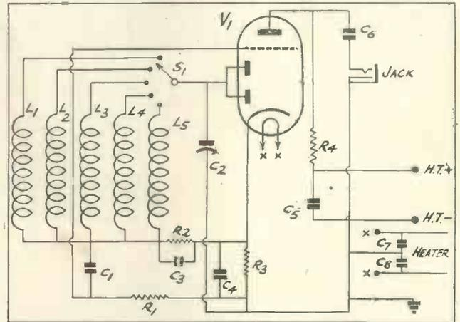
Fig. 3. On the right is the diode-triode phone monitor circuit.
