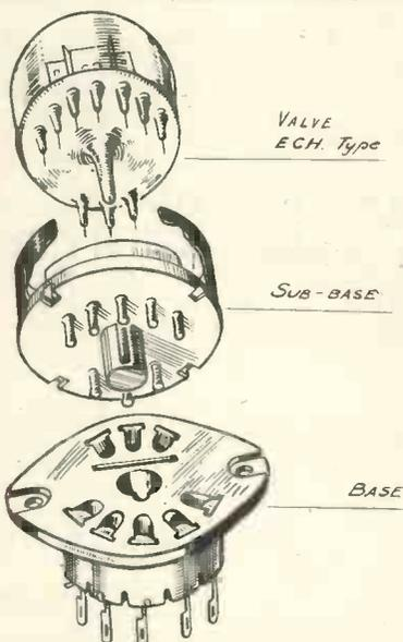
This special drawing shows the glass bulb and lead out wires underneath which is the sub-base and finally the new type of valve holder.
