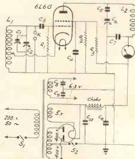
This is the circuit of the single valve transmitter with which contacts have been made in America Canada and South America.
