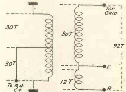
How the coil is wired.
