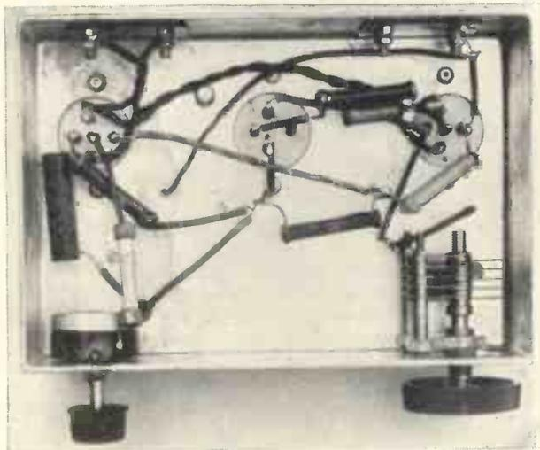
Under-chassis view of modulated oscillator.
