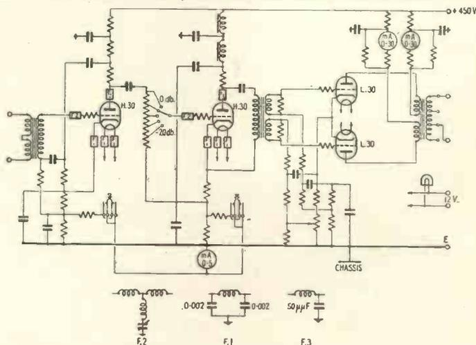
Fig. 6. Circuit of main amplifier.
