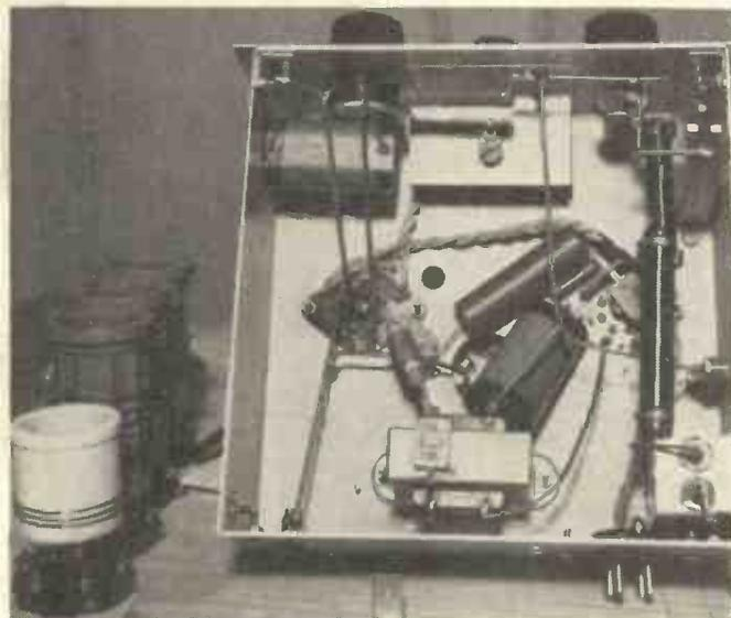
As can be seen from this sub-chassis view the very minimum of components are required while coils cover all amateur wavebands. It is recommended that the U.H.F. coil be wound on ceramic.
