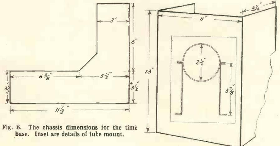
Fig. 8. The chassis dimensions for the time base. Inset are details of tube mount.
