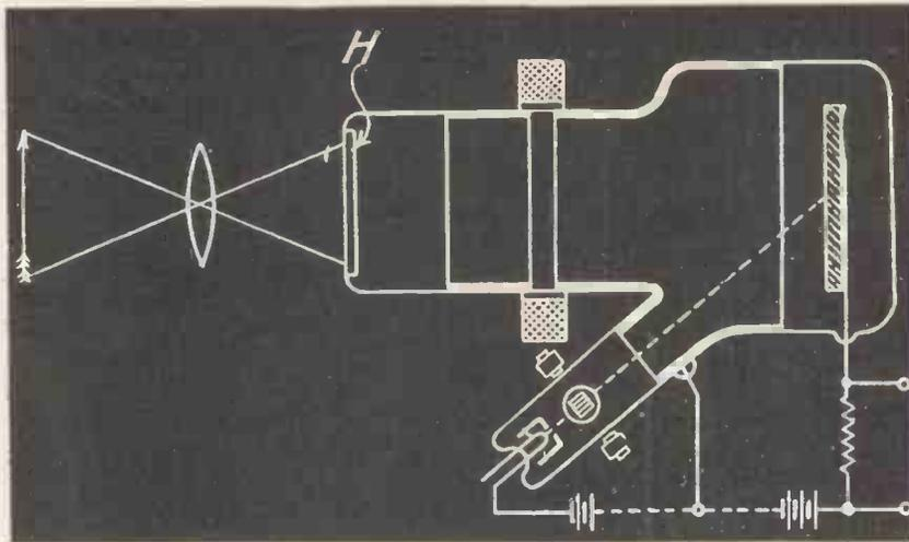
Fig. 3. An alternative method of using the principle employing an electron image.
