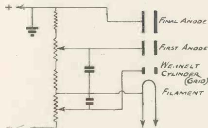
Fig. 2b.—Potentiometer for use with hard tubes.
