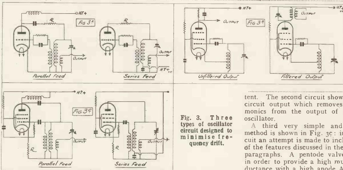
Fig. 3. Three types of oscillator circuit designed to minimise frequency drift.
