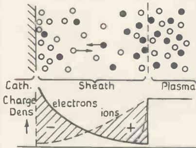
Fig. 16. Space charges in cathode sheath.
