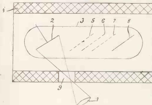
Fig. 2 (right). Modifications of the grid-type electron multiplier.
