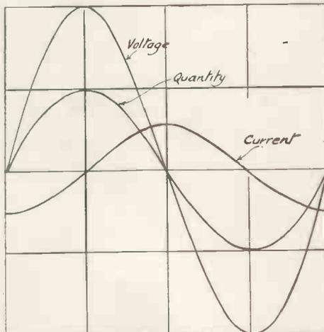
Fig. 1. Showing how the current flowing through a condenser differs in phase by 90° from the applied voltage.
