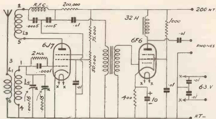
Circuit diagram of the two-valve mains-operated receiver.
