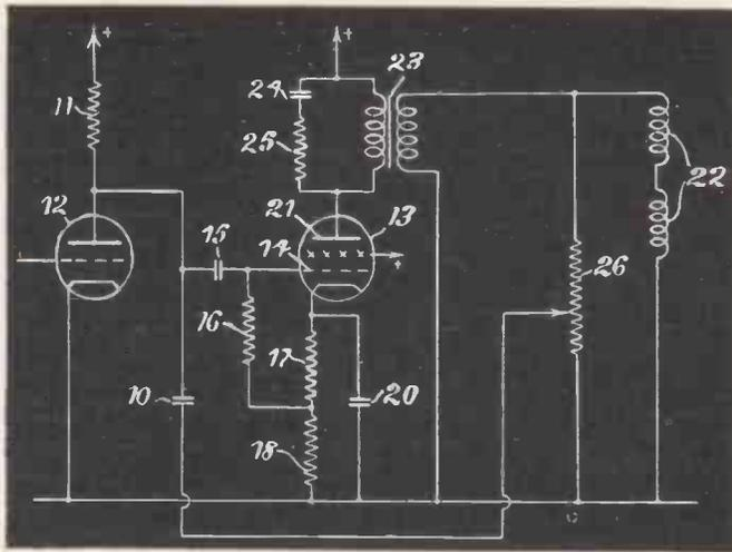
Fig. 1. Circuit diagram of improved scanning oscillator
