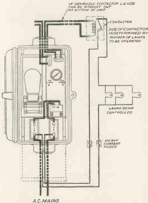
Schematic diagram of control gear for group lighting.
