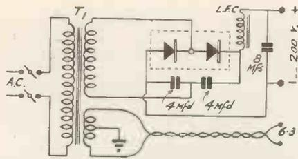
A metal rectifier is used in the power unit. This is the circuit.
