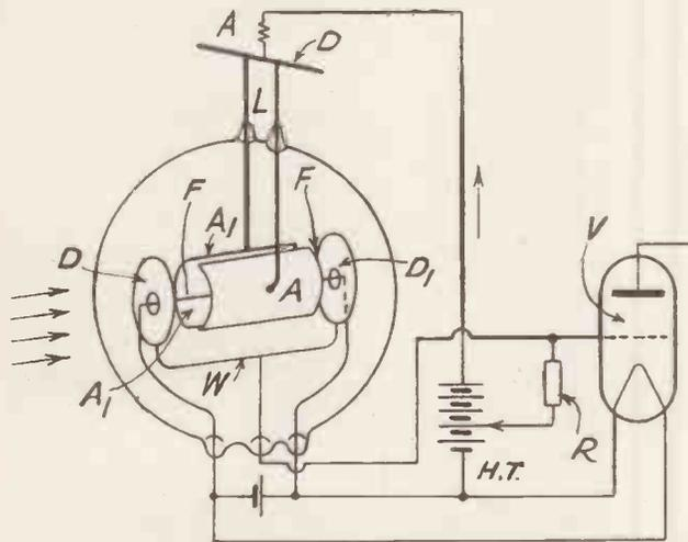
Left: Magnetron circuit for reception of ultra-short waves.
