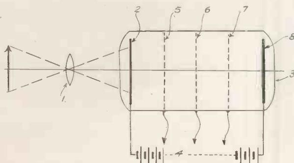
Fig. 1 (left). Diagram of typical grid type electron multiplier.
