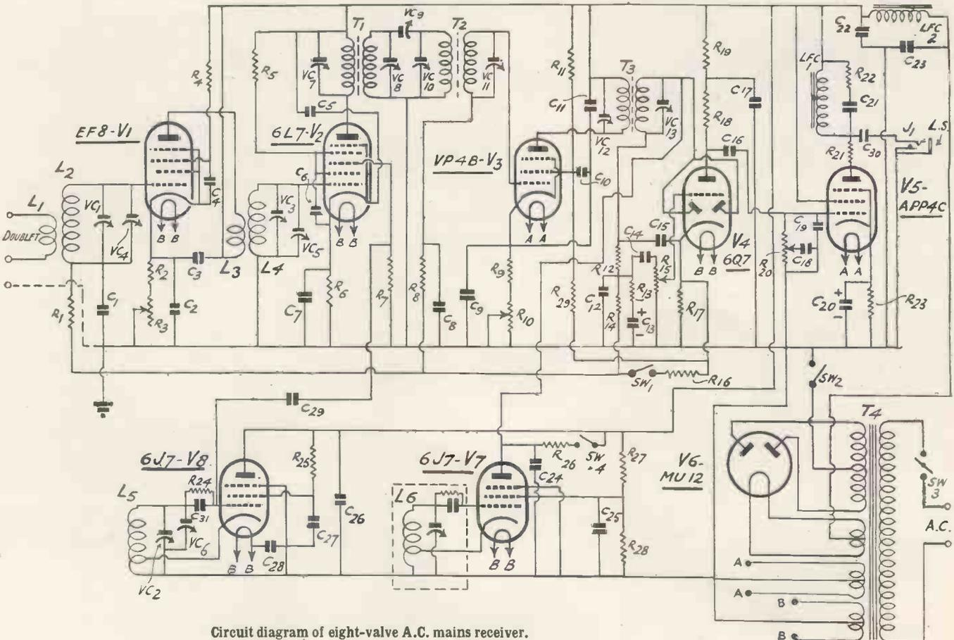
Circuit diagram of eight-valve A.C. mains receiver.
