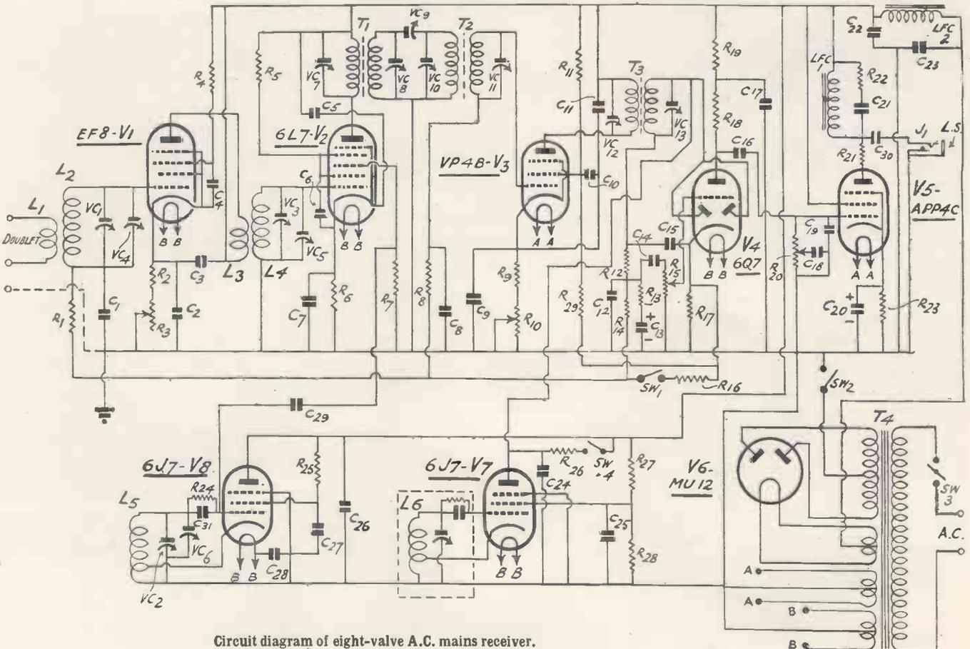
Circuit diagram of eight-valve A.C. mains receiver.
