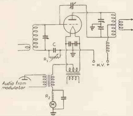
Fig. 1.—The fundamental cathode-modulation circuit. Audio from the modulator unit is introduced in the cathode (centre-tap) circuit of the valve or valves being modulated. The grid-leak resistance  $R_1$  is adjusted for proper modulation characteristics, and  $R_2$  serves to give some original bias to the valve. Condenser C must be large enough to by-pass the modulation frequencies.
