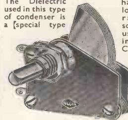
having extremely low losses, even at high radio frequencies so that it may be used with confidence in exacting positions. Capacity, .0005 μF. max., and condenser is provided with ¼ in. shaft with one-hole fixing-bush. The full capacity range is obtained in the 180° swing ± 15 per cent.
