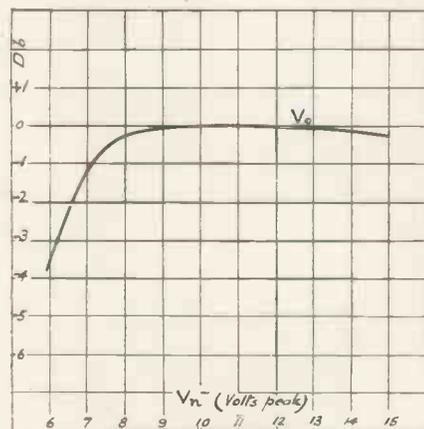
Fig. 4. Variation of beat frequency output  $V_o$  with the output voltage  $V_n$  of the variable oscillator.
