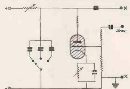
Fig. 3.—Simple form of gas-relay time base.
