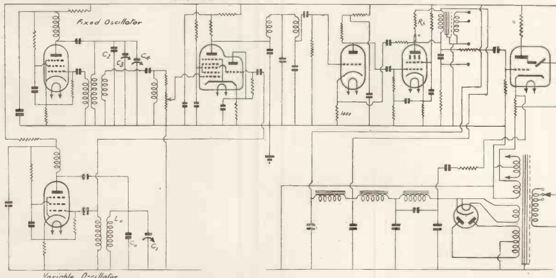
Fig. 6. A suggested circuit for a beat note oscillator embodying the points discussed. A design based on this is being given shortly.
