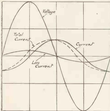
Fig. 2. Where there is loss in the condenser, the current is not at 90°, but at an angle less than 90°.
