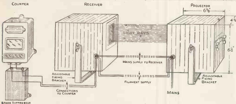
Diagram showing the arrangement of the counting apparatus.
