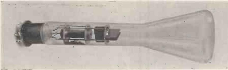
The 4096-AB cathode ray tube, as manufactured by Standard Telephones and Cables Limited, is a high vacuum tube with a 3 in. diameter screen. It employs electrostatic deflection and focusing. The gun is of the two-anode type and its simple construction ensures great accuracy in alignment without complicated manufacturing methods.
