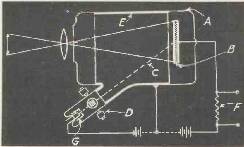
Fig. 1. Schematic diagram of television transmitter employing the new tube.
