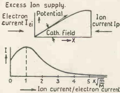
Fig. 18. Effect of ion supply on current.
