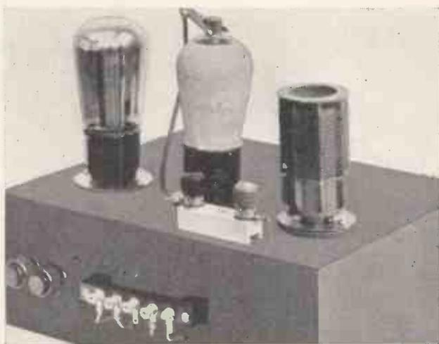
The same chassis is used as for the one-valve receiver.
