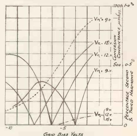
Fig. 5. Variation of 2nd and 3rd harmonic of beat frequency with the amplitude of  $V_n$ . The full line is % 2nd harmonic and the chain dotted line 3rd harmonic. Conversion conductance is shown by the dotted line. ( $V_s$  0.2 v. peak).
