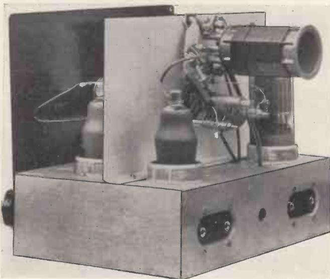
Rear view of three-valve mains receiver.
