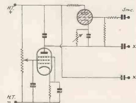
Fig. 4.—Gas-relay time base using pentode charging.
