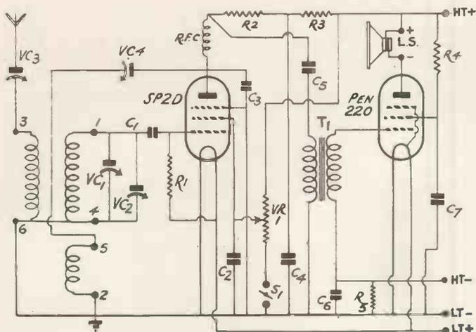
Circuit diagram of the two-valve battery-operated receiver.
