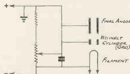
Fig. 2c.—Potentiometer for use with soft tubes, which usually require positive Wehnelt.
