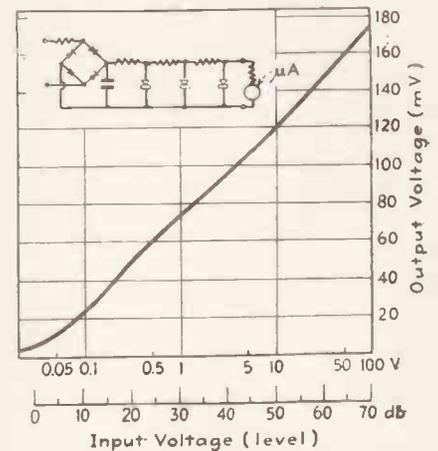
Fig. 3.—Logarithmic characteristics of completed meter with meter connections shown in upper left.
