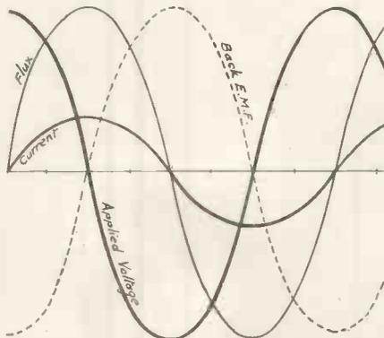
Fig. 3. The curves of voltage and current through an inductance for comparison with those of a condenser (Fig. 1 & 2.)
