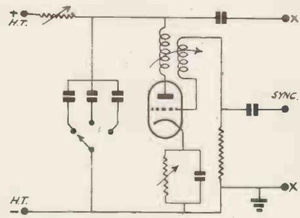
Fig. 5 (left). Simple form of hard valve time base.
