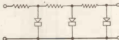
Fig. 2.—Series-parallel arrangement for extending the logarithmic range of the rectifiers.
