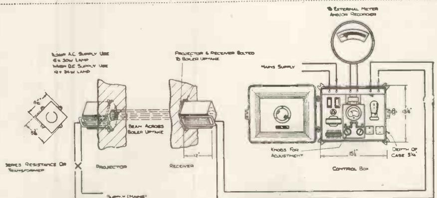
Diagram showing arrangement of smoke indication apparatus for use on smoke stacks.
