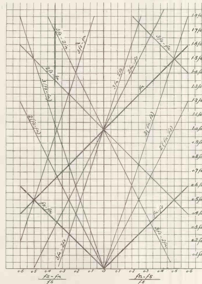
Fig. 2. A chart showing the spurious frequencies present in the output of the detector fed by the two frequencies  $f_s$  and  $f_n$ .
