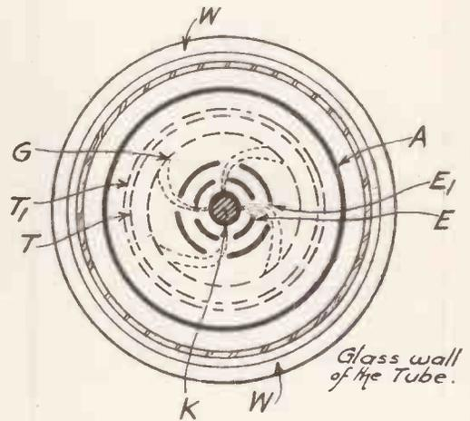
stead of a straight path, and so regulates their time of flight. In general, for maximum output, the wavelength produced by a magnetron valve of this type is inversely proportional to the strength of the field.
