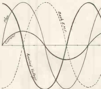
Fig. 3. The curves of voltage and current through an inductance for comparison with those of a condenser (Fig. 1 & 2.)
