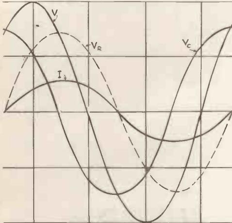
the resistance it will read approximately 200 volts, but when connected across the condenser it will read not 50 v. but 150 volts. These values may not be obtained exactly owing to the tolerances on the component values, but there will always be a sufficient margin to demonstrate that the total applied voltage is not equal to the sum of the two individual voltages.
