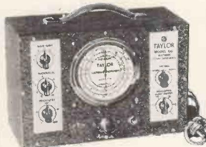
Mains operated, it covers 6.5 to 3,000 metres, 100 kc. to 46 mc. in 6 bands, directly calibrated. Almost constant output, low harmonic content. Up to 50 per cent. variable internal or external modulation. Saves hours of tedious work.
