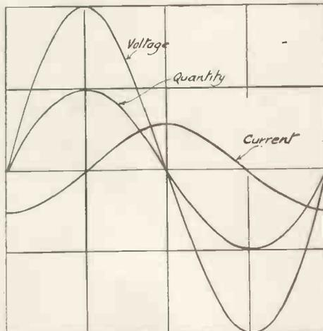
Fig. 1. Showing how the current flowing through a condenser differs in phase by 90° from the applied voltage.
