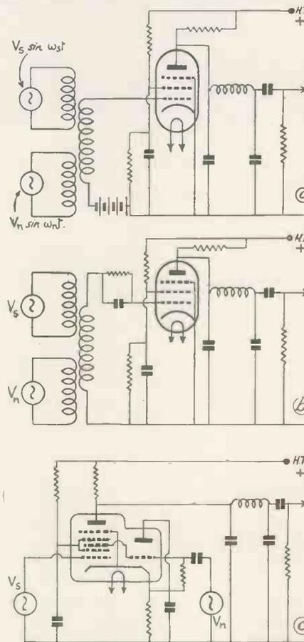
Fig. 1.—Three methods of producing beat frequency. By using a pentode (a & b) and a hexode (c).
