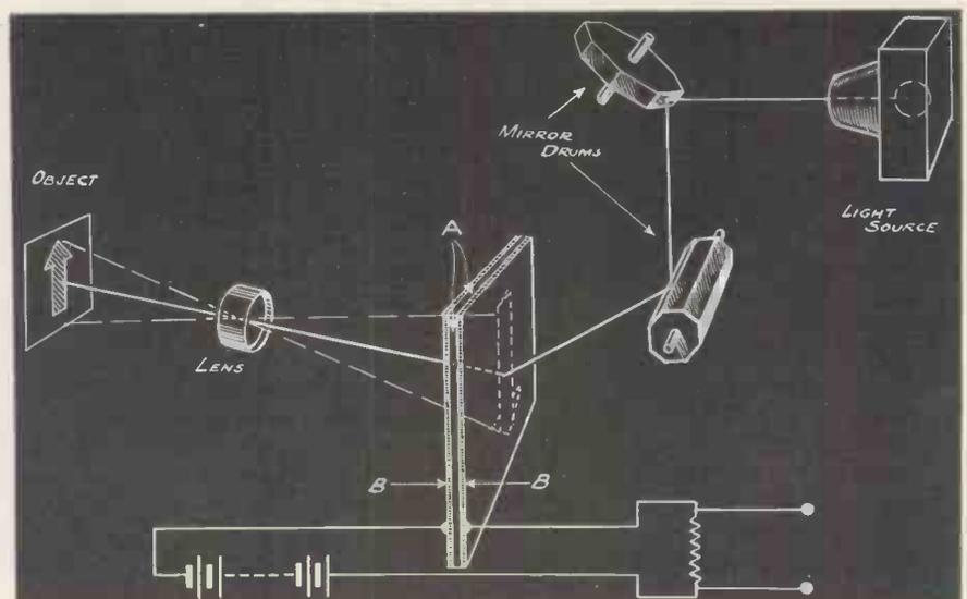
Fig. 4. Scheme for employing light for both image formation and scanning.
