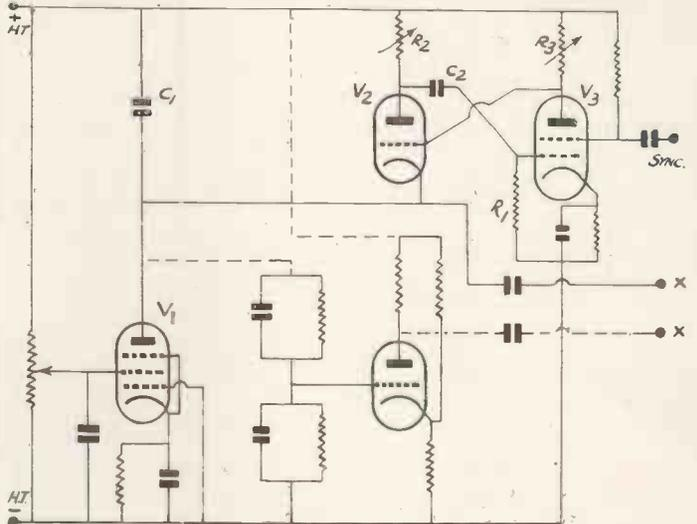
Fig. 6 (right). This figure gives the circuit diagram of a hard valve time base, efficient up to quite high frequencies. Balanced deflection is provided.
