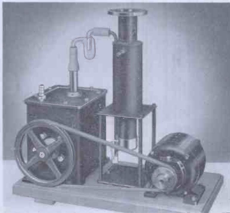
Fig. 8. Mercury-vapour diffusion pump in use in conjunction with mechanical backing pump.
