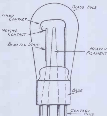
Fig. 4. Vacuum-type thermal delay switch.
