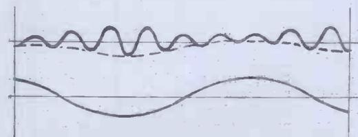
Fig. 4. The modulated beat frequency after detection a second time, leaving the audio frequency component.
