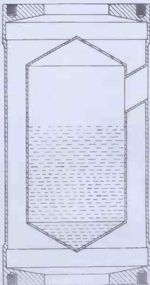
Fig. 7. Diagram showing operating principle of mercury-vapour trap.
