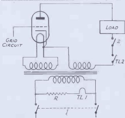
means of the main switch, the anode voltage disappears before the cathode commences to cool down. In the event of sudden voltage failure the process is the same; the timer cooling down again ready to operate upon resumption of the supply.
