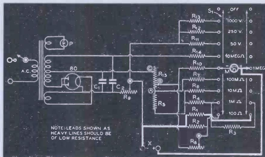
Fig. 2. Circuit diagram of A.C. operated ohmmeter.
