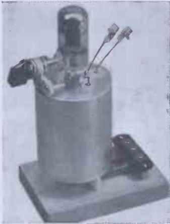
A Peterson "pot" oscillator for 112 Mc. using two shield cans and a copper rod for the tank circuit. The stability is superior to any other form of U.H.F. self-excited oscillator.
