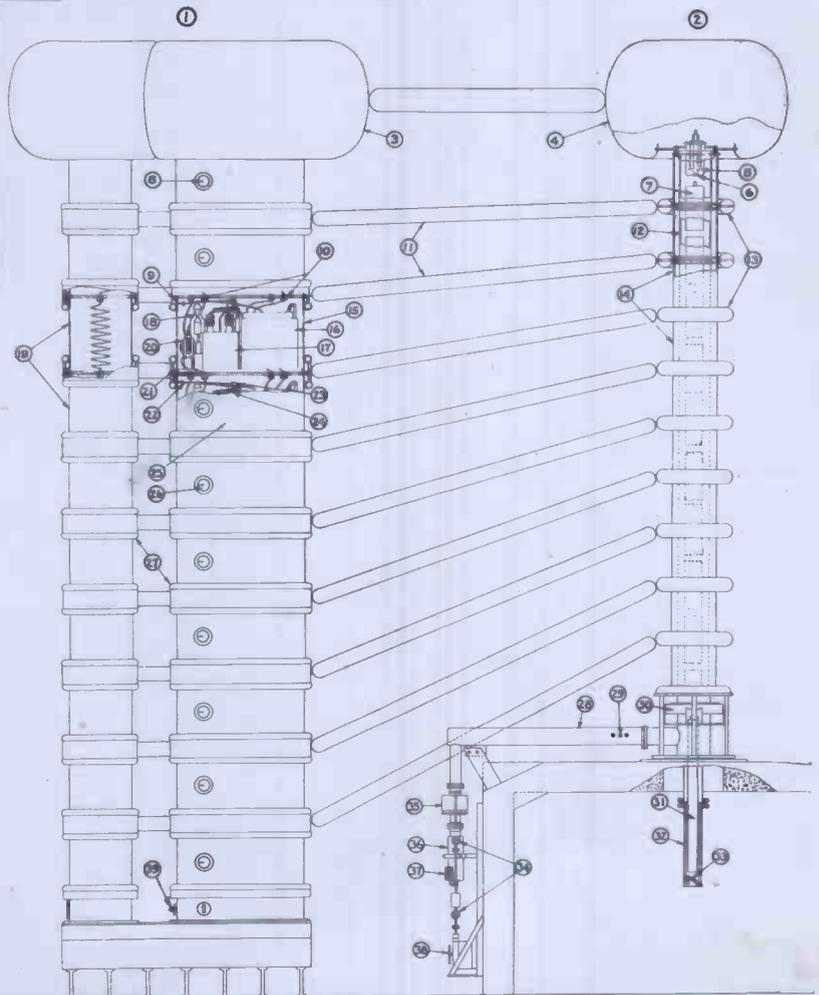
Fig. 1. Assembly of 1,400,000-volt constant-potential X-ray equipment.
