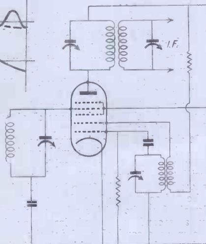
Fig. 6. A valve used as a combined oscillator and detector.
