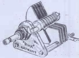
Our standard range of micro-variables are of all-brass construction with heavy gauge vanes and a special device electrically short-circuits the ball-bearing spindle, giving noise-free operation with smooth control and avoiding the troubles inherent with old-fashioned pigtails. Ceramic insulation (RMX) is the latest product of the laboratories. Note how it improves at high frequencies.
