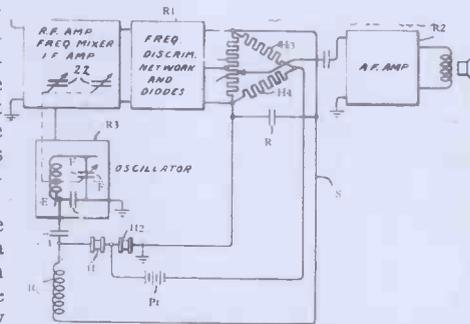
Fig. 3. Another modification using a resistive bridge circuit.
