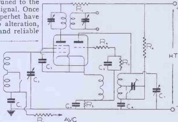
Fig. 7. A heptode valve in which the coupling is by electron stream.
