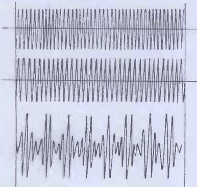
Fig. 1. Showing how two notes of slightly different frequency combine to produce 'beats.'
