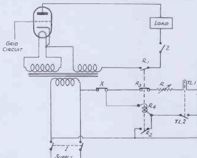
The properly designed thermal timer is compact and reliable. It is available in a wide range of types, covering time lags up to about 2 minutes. For longer periods it is usually necessary to employ more expensive types of apparatus, employing some form of air or oil dashpot, or eddy current retarding device.
