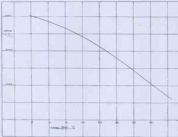
Fig. 9. Curve showing effect of cooling water temperature on speed of diffusion pump.
