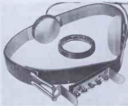
View of headband and electrodes for application of the shock to the skull.
