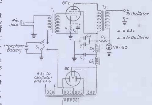
Fig. 2. A modulator and power supply suitable for use with the "pot" oscillator.
