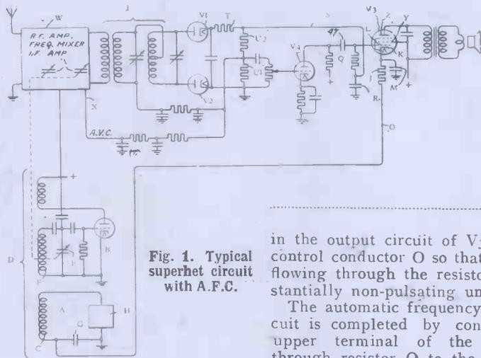
Fig. 1. Typical superhet circuit with A.F.C.
