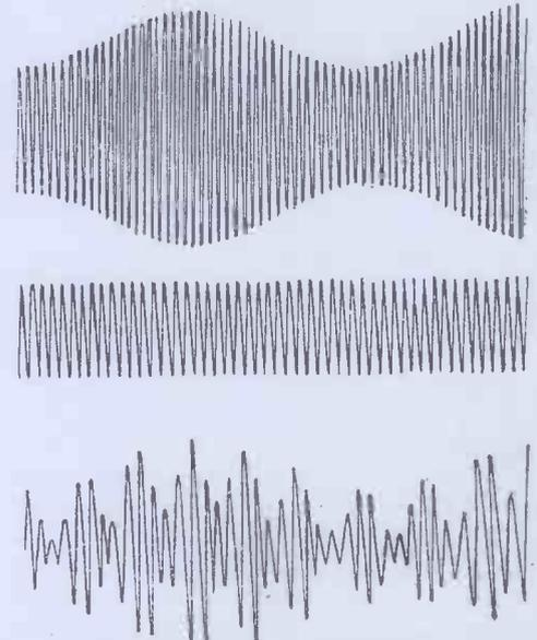
Fig. 2. A modulated carrier wave combined with a local oscillation frequency reproduces the modulation in the beat frequency.
