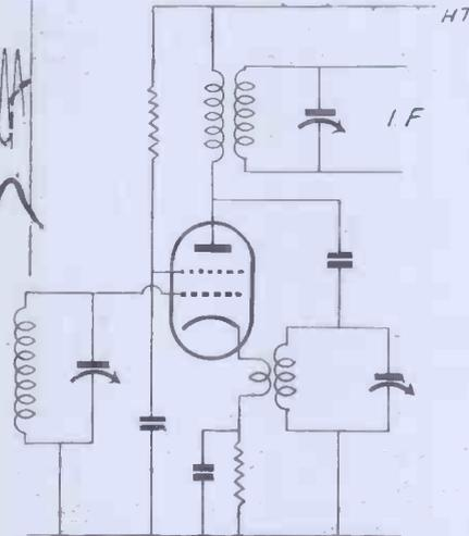
Fig. 5. A simple circuit for injecting an oscillation into the first detector.
