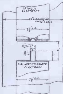
Fig. 8. Cathode section of the X-ray tube.
