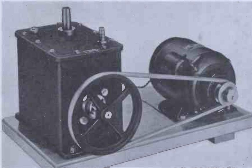
Fig. 2. Complete "Speedivac" mechanical rotary pump.
