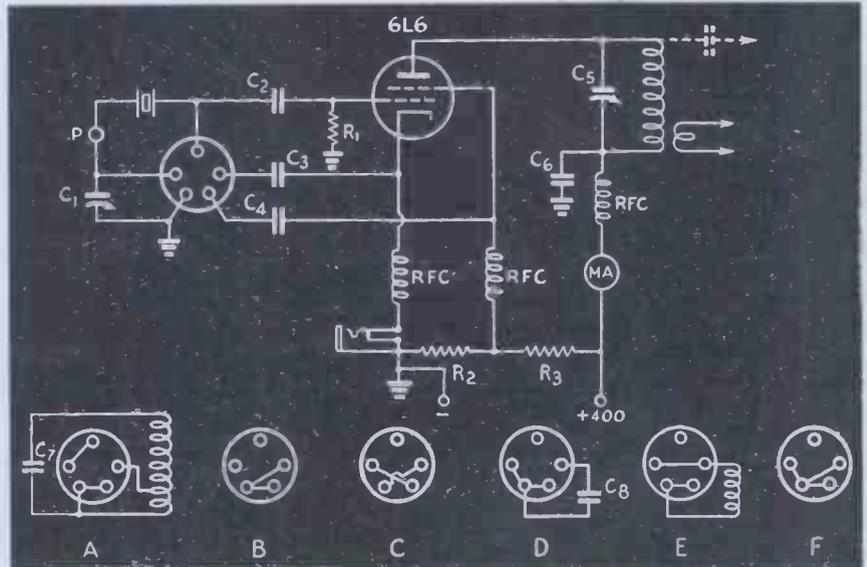
Fig. 1. Circuit diagram of experimental oscillator and details of coil and plug connections.
