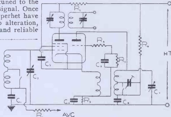
Fig. 7. A heptode valve in which the coupling is by electron stream.
