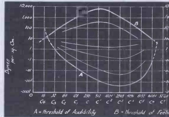
Fig. 1. The aural spectrum curves obtained by the Bell Laboratories in U.S.A.
