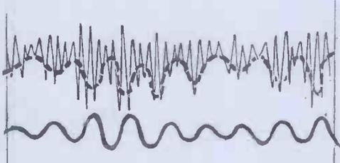
Fig. 3. The modulated beat frequency after rectification showing the anode current fluctuations following the modulation.
