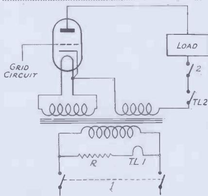
Fig. 2 (left). Simple timing circuit for cathode pre-heating.
