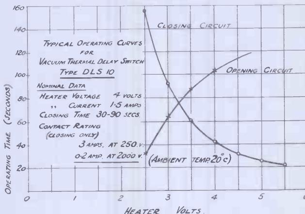
Fig. 5 Characteristics of vacuum-type thermal delay switch.
