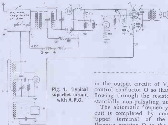
Fig. 1. Typical superhet circuit with A.F.C.
