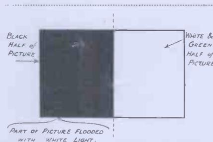
Diagram elucidating the fact that "the colour contrasts are not affected so greatly as are simple black and white contrasts, when the picture is flooded with external light."
