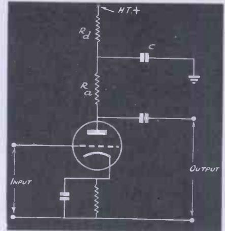
Fig. 3. Conventional resistance-capacity amplifier, showing method of decoupling anode and cathode circuits.
