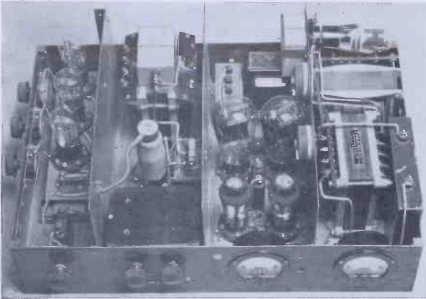
Complete amplifier showing the disposition of the components. The L.H. section shows the three input channels; the second, the tone control stage; the third the paraphrase and output valves, and the fourth the power supply.
