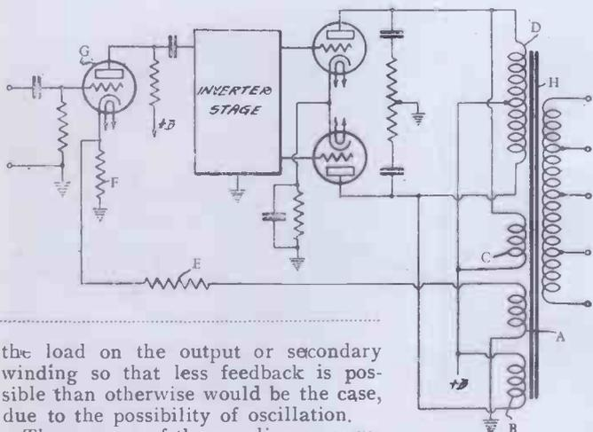
Fig. 1. Circuit arrangement for reduction of phase shift in negative feedback amplifiers.
