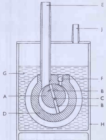
Fig. 1. Diagram showing operating principle of rotary mechanical vacuum pump.
