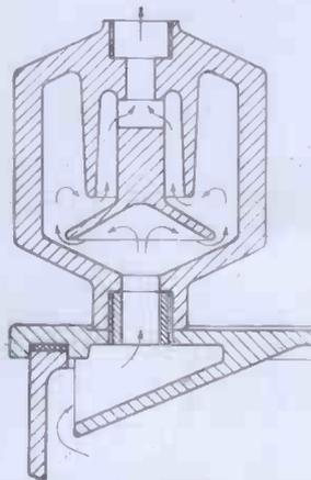
Fig. 4. Diagram of spray arrestor for mechanical rotary pump.
