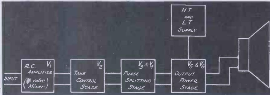
Fig. 2. Schematic diagram of the valve sequence.
