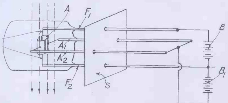
Arrangement of Magnetron valve for generating centimetre waves. Patent No. 526,827.
