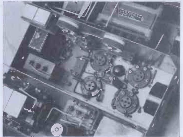
Close-up of the paraphase and output valves showing the close proximity of the components in order to ensure very short connections.
