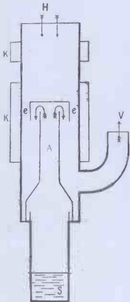
Fig. 5. Diagram showing operating principle of mercury diffusion pump.
