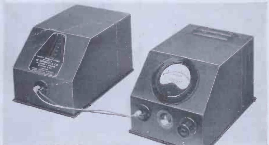
Fig. 13. The Philips direct-reading gauge.
