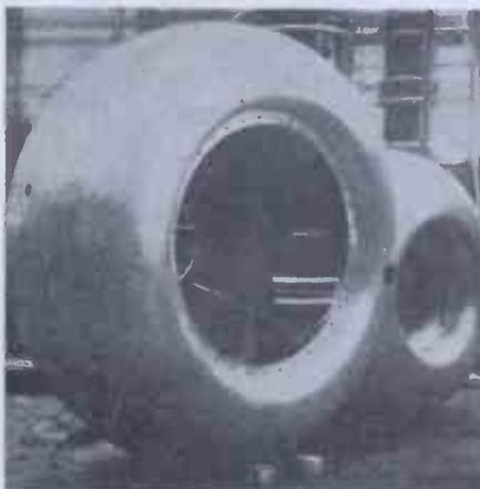
Fig. 6. Corona shield of the high-voltage generator.
