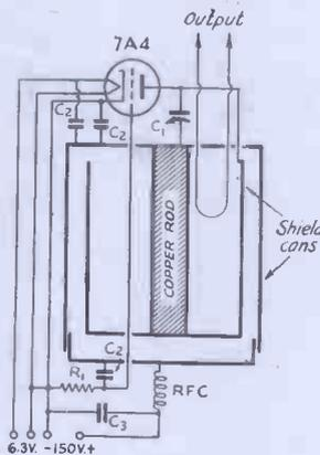
Fig. 1. Circuit diagram of the "pot" oscillator using shield cans for the concentric cylinders.
