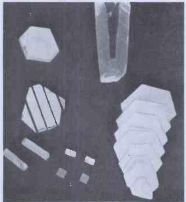
Fig. 3. Quartz crystals in different stages of preparation. Top centre : an uncut mother-quartz crystal. Lower right : a crystal after the first sawing operation. Top left : one of the resulting sections, and beneath it a section after being sawed into bars. Bottom left : bars before and after the final sawing operation, and also four of the resulting radio crystals ready for the various finishing operations.
