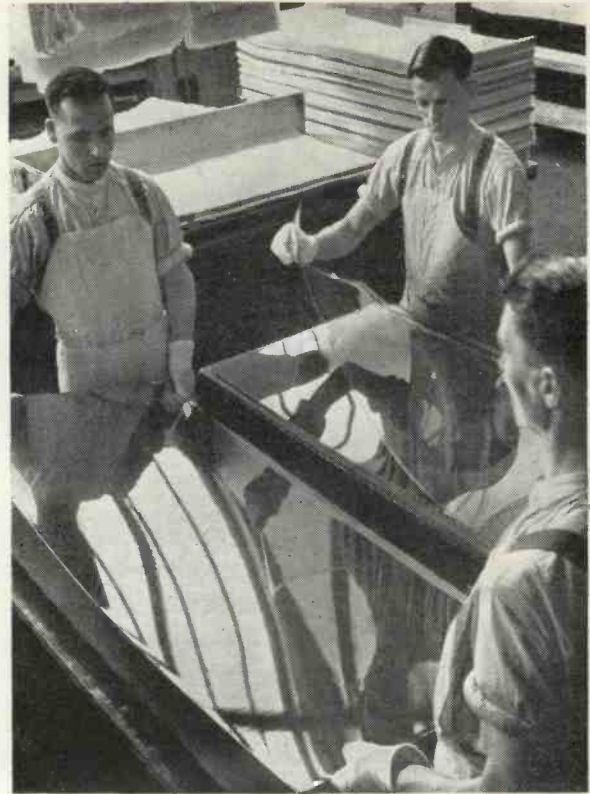
Fig. 2 (right). Removing polished celluloid sheet from polishing "nip."
