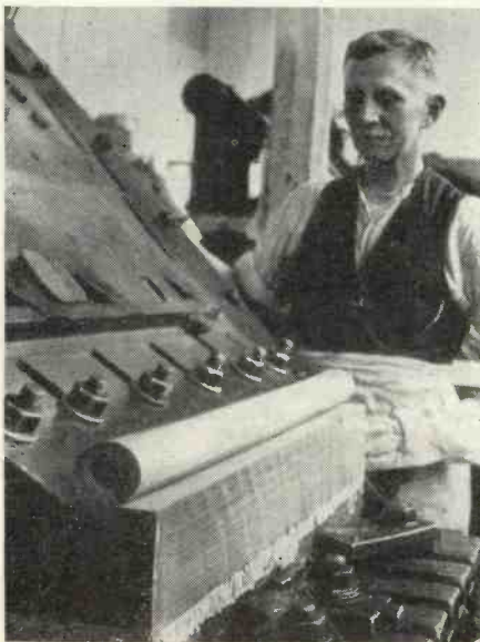
Fig. 1 (left). Slicing celluloid block.
