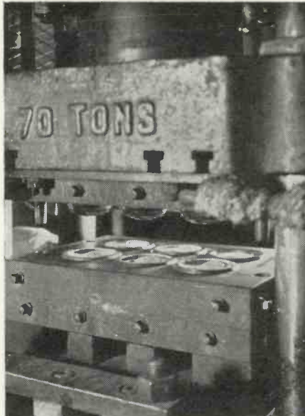
Fig. 8. Moulding of Bakelite (Press closing). Courtesy of Bakelite, Ltd.
