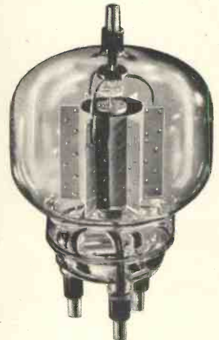
Fig. 12. 4,000 v. 350 w. triode type 357A (Western Electric) with 100% ratings down to 100 Mc/s. The leads are made of solid copper sealed through the glass.
