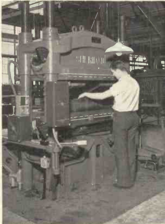
Fig. 1. Electronic safety guard for power press operator. The light beam is interrupted by the shoulder (white rectangle). This press is also fitted with electronic time delay circuits to allow it to remain closed for a predetermined length of time. (Courtesy, Arvey Corporation, Detroit, U.S.A.)
