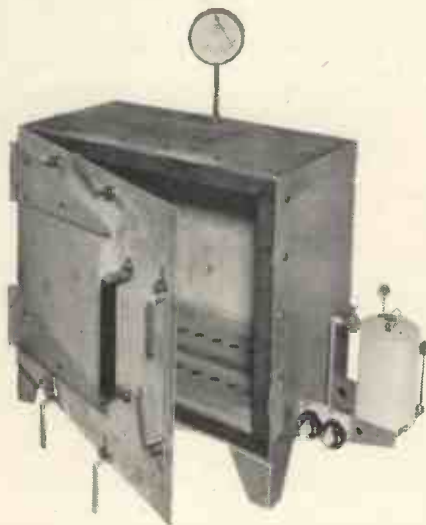
Special humidity chamber for testing export receivers under conditions of heat and damp.
