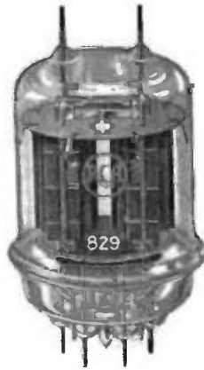
Fig. 19. R.C.A. 829 push-pull beam tetrode, with max. total anode dissipation of 40 w. at 500 v. Ratings are 100 per cent. down to 150 cm. Bulb diameter 2".
