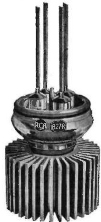
Fig. 20. R.C.A. 827R. A radiation-cooled beam tetrode operating at 3-35 kv. with an anode dissipation of 800 watts. This valve has 100 per cent. ratings down to a wavelength of 90 cm. Max. diameter of radiators: 4.65".
