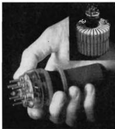
Fig. 16. This illustration shows the remarkably small size of the G.L. 8002, which is a 3000 v. 1200 watt water-cooled triode with 100 per cent. ratings down to 200 cm., at which wavelength it delivers 1800 watts. Inset: GL. 8002R.
