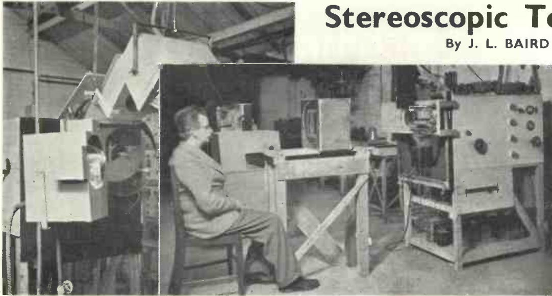
A photograph of Mr. Baird in front of his experimental receiver and (left) a view of the transmitter showing shutter and photocells.
