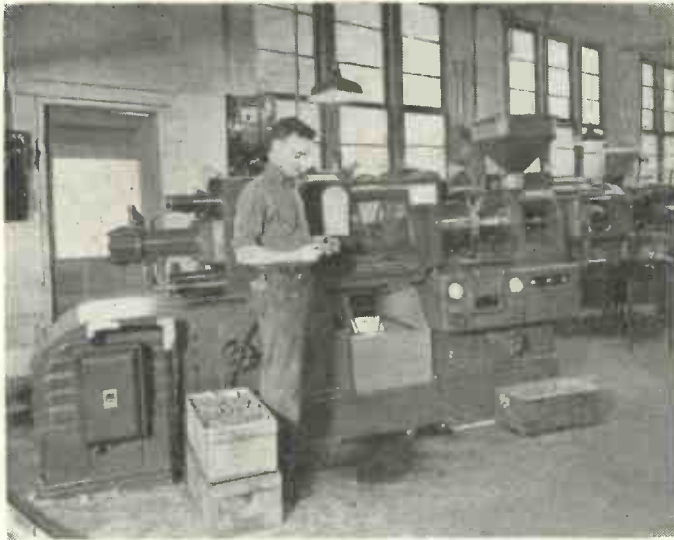
Fig. 1. Automatic machine for mass production of injection mouldings. The operator is holding a set of mouldings which have just been expressed from the machine. (Courtesy of Alfred Herbert, Coventry.)
