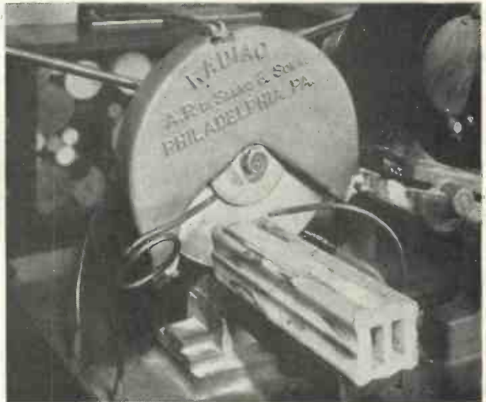
Fig. 4. Cutting sections of cast phenol-formaldehyde resin. (Courtesy of Catalin, Ltd.)
