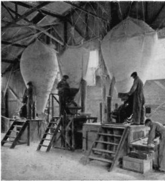
Fig. 1. Grinding mica particles. The fabric bags at the back cover the air outlet from the grinder.
