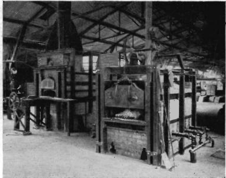
Processes in the manufacture of Mycalex : Fig. 3 (left) Compressing the mica-glass mixture in a hydraulic press before final firing, and Fig. 2 (right), The glass ingredients undergoing preliminary baking before being mixed with mica flour.
