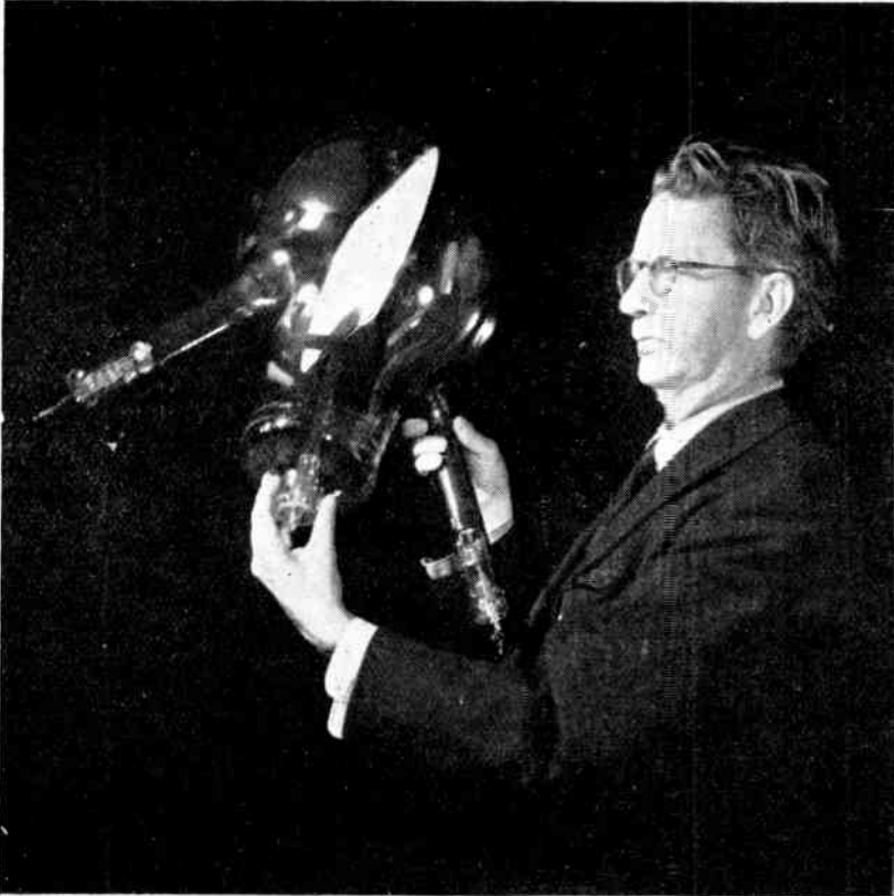
J. L. Baird with his new two-colour Cathode Ray Tube.
