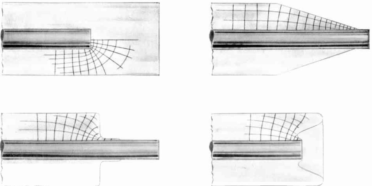
Fig. 2. Lines of principal stress for four "rod" seals.
