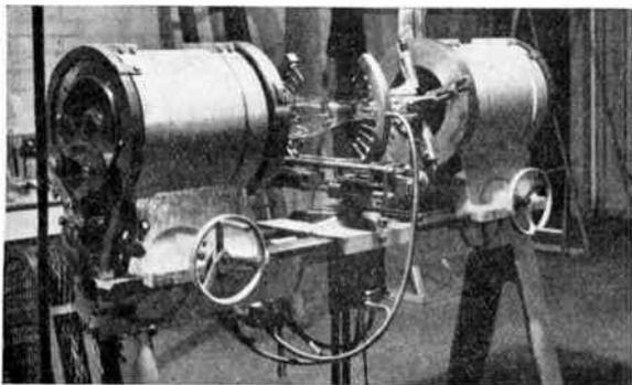
Fig. 9. Large sealing lathe for tubes.
