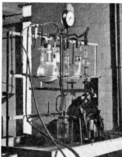
Fig. 3. Oil filling plant for tubes.
