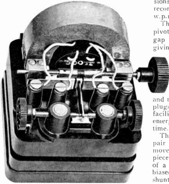
**A** HIGH speed relay developed by the Automatic Telegraph and Radio Transceiver Co., Ltd., combines small overall dimensions with a high sensitivity and a recorded working speed of 1,000 w.p.m.
