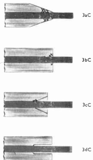
Fig. 3. Crack systems for "rod" seals loaded mechanically so that the free end of the rod is bent downwards.
