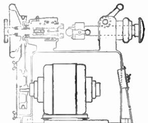
*A cross-section of the Plug Maintenance Machine shows how a S.E.M.  $\frac{1}{4}$ -h.p. motor drives the head-stock by means of a V-shaped endless belt*
