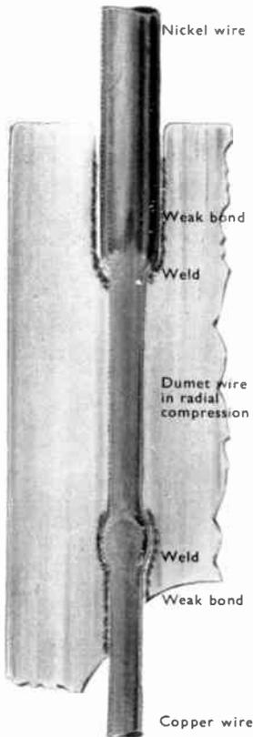
Fig. 6. Rod seal of copper-Dumet-nickel through C.12 glass.
