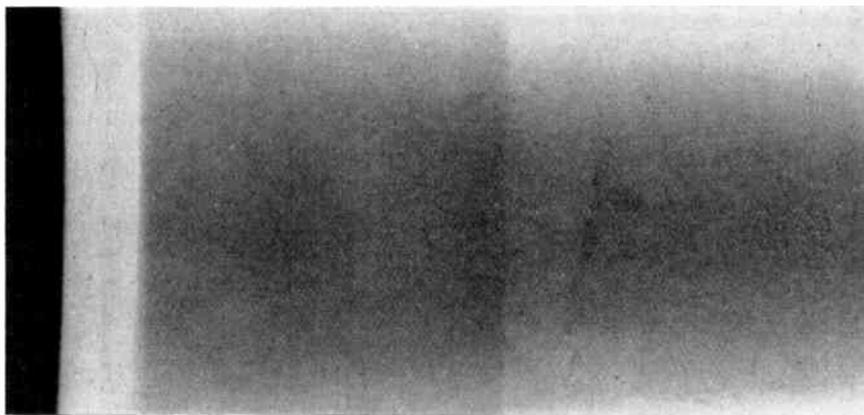
Fig. 2. Radiograph of portion of a porcelain high-tension insulator showing porous region and crack.
