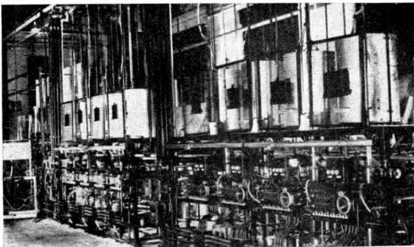
Fig. 4. Exhaust benches for H.T. rectifiers showing baking ovens in place.
