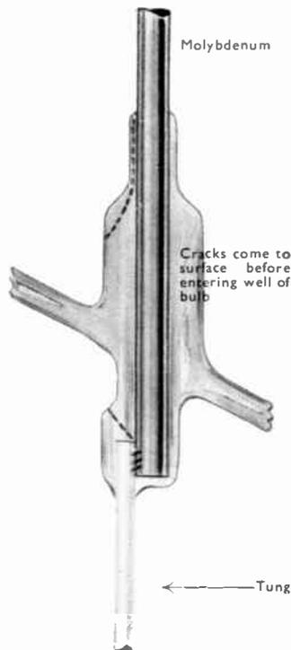
Fig. 4. Rod seal of molybdenum through C.14 glass.
