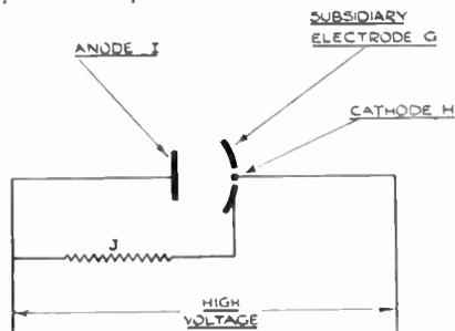
Fig. 4. Diagram illustrating electrode assembly in X-ray tube for high speed radiography.
