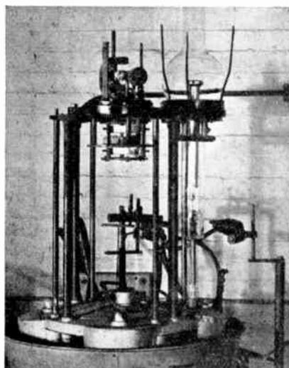
Fig. 7. Four-head drop sealing machine.
