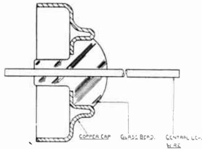
Fig. 1. Sectional drawing of glass-metal seal.
