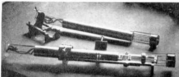
Fig. 2. Assembly jigs for H.T. Rectifier electrodes.
