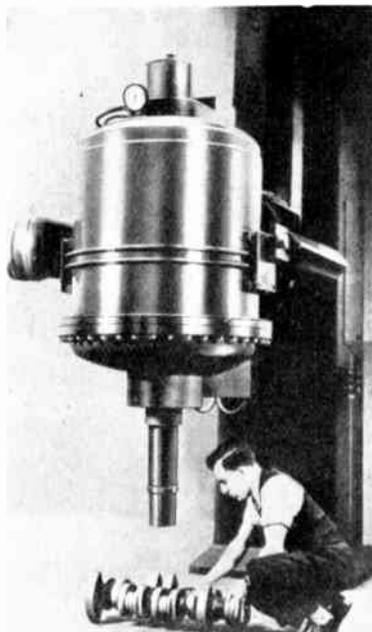
Fig. 3. The General Electric 1,000 kV X-ray tube. (Courtesy of the Victor X-ray Corporation, Ltd.)
