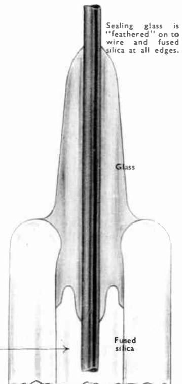
Fig. 5. Rod seal of tungsten into glass into fused silica.
