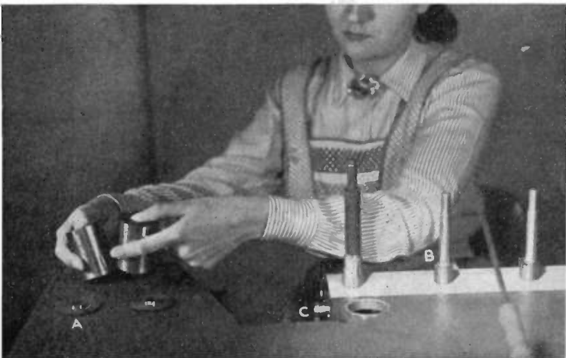
Figs. 4 (top), 5 (centre) and 6 (bottom).—Three stages in the assembly of carbon rings for grinding.
