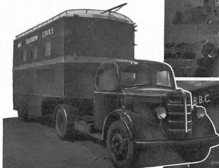
The photograph above shows the new mobile control room, manufactured by Pye Ltd., to the B.B.C.'s specification for television outside broadcasts. On arrival at the O.B. Point, the motor is usually detached from the trailer.
