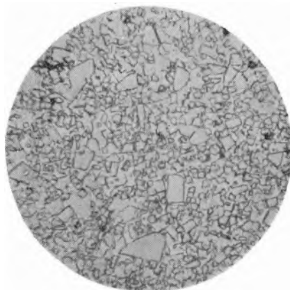
Fig. 1c. Hard Metal, 6 per cent cobalt (etched with alkaline potassium ferricyanide)
