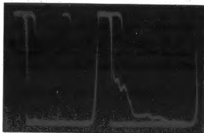
Fig. 18. Pattern obtained with razor blade tester, showing a number of defective blades, compared with the edges of good blades
