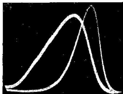
Fig. 21b. Light distribution in image showing chromatic aberration. Pattern at left, at centre of image; at right, at edge of image
