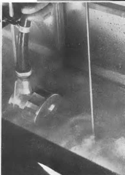
The new Mullard Ultrasonic Generator with covers removed with transducer head in foreground
