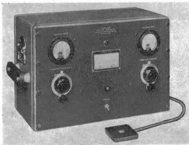
Model U.500 Ultrason, capable of giving a maximum of 6 watts output power
