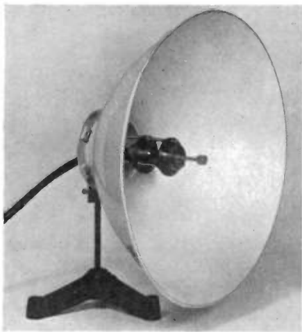
Fig. 7. Hartmann whistle mounted in reflector
