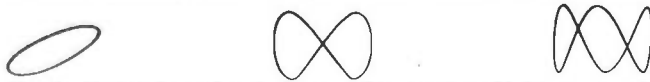
Fig. 8. Typical traces for electro-magnetic generator. First, second and third order Lissajous figures representing speeds of 600, 1,200 and 1,800 r.p.m.
