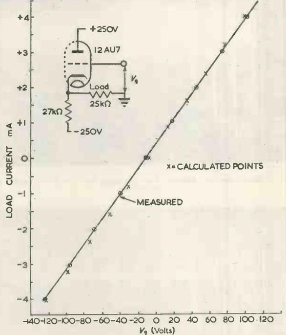
Fig. 5. Measured and calculated performance
