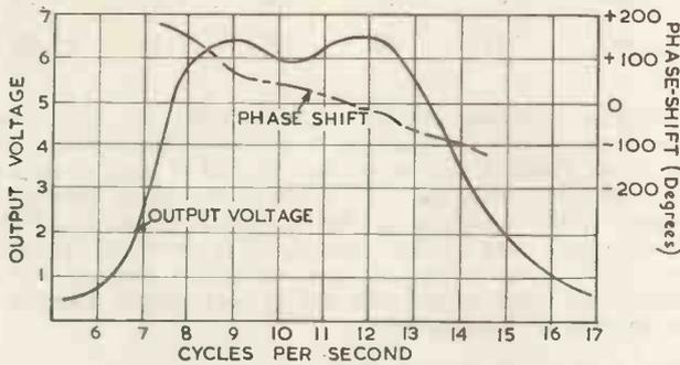
Fig. 6. Response of filter unit combining five resonant circuits of the type shown in Fig. 3(b)
