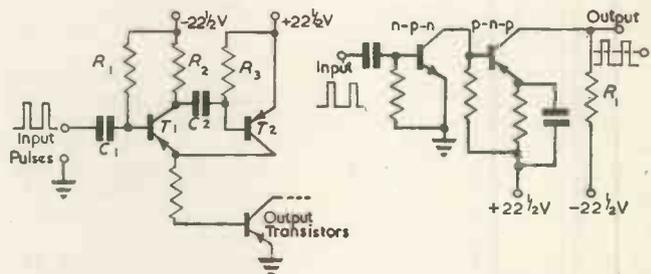
Fig. 24. "Totem pole" circuit Fig. 25. Direct-coupled pulse amplifier
