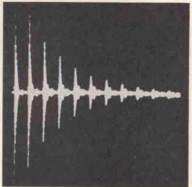
Fig. 1, where the exposure time was chosen to suit the brightness of the largest amplitude signal. Fig 2 shows that if the exposure time is correct for the smaller amplitude signals, the larger amplitude signals are underexposed.
