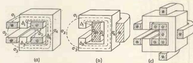
Fig. 2. Winding arrangements
