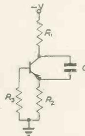
Fig. 20. Vertical oscillator
