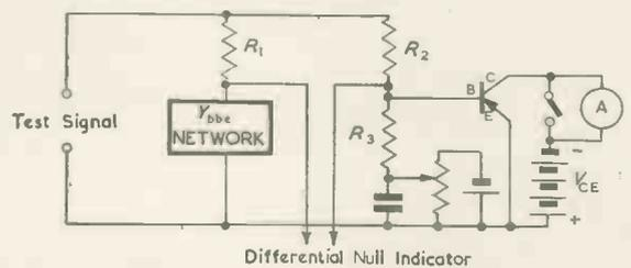
Fig. 3. Common-emitter input admittance bridge test set
