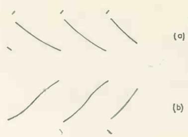
Fig. 21. Waveforms of (a) vertical oscillator output; (b) vertical yoke voltage
