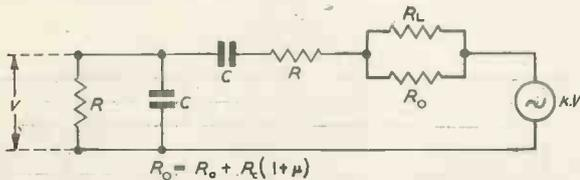
Fig. 9. Equivalent circuit of two-stage filter
