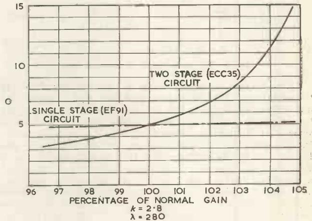
Fig. 8. Variation of circuit Q with stage gain
