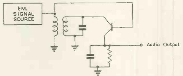
Fig. 18. Transistor FM detector
