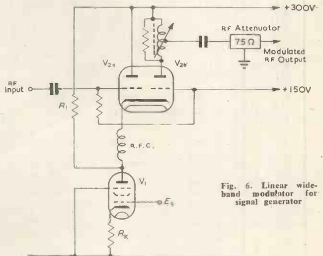
Fig. 6. Linear wideband modulator for signal generator
