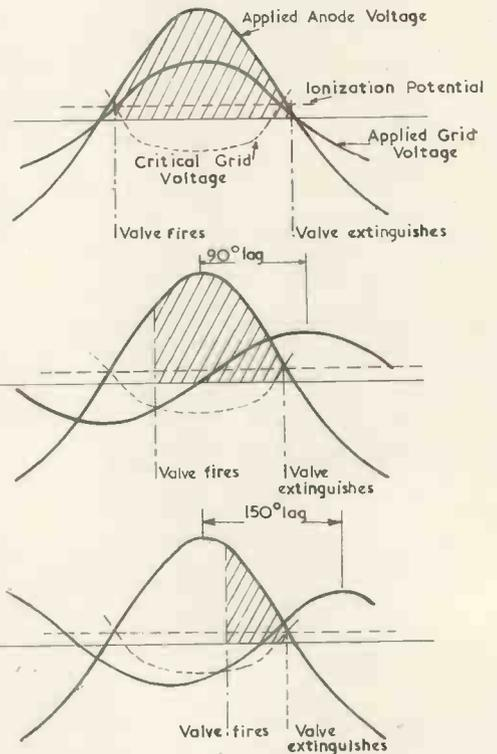
Fig. 3. Control of thyatron firing point using A.C.
