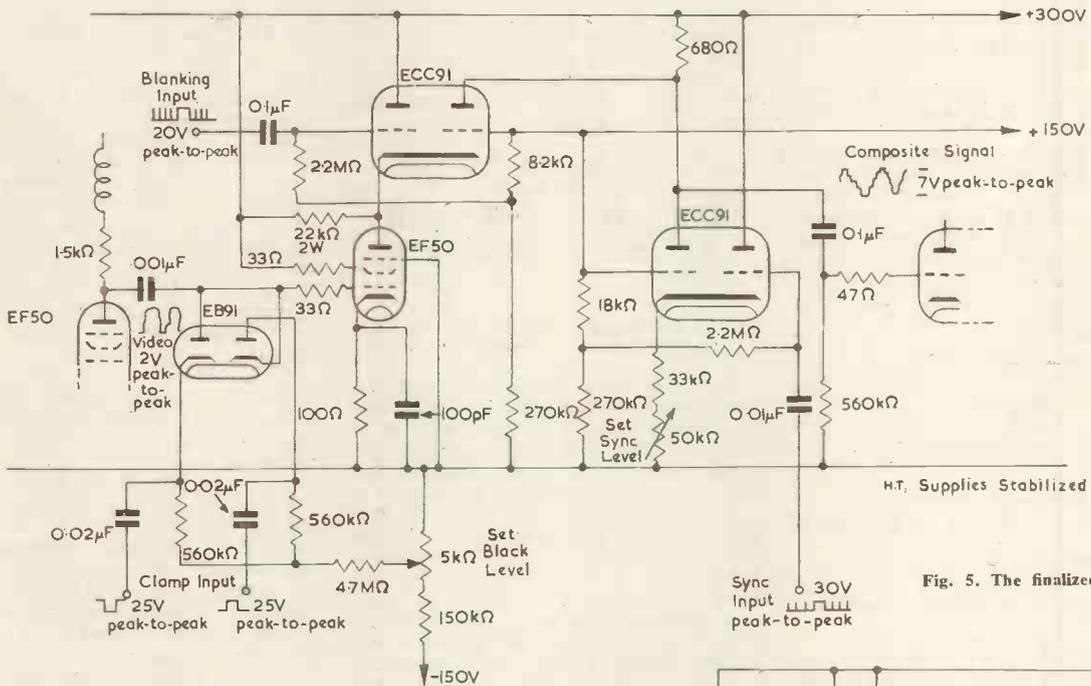
Fig. 5. The finalized circuit
