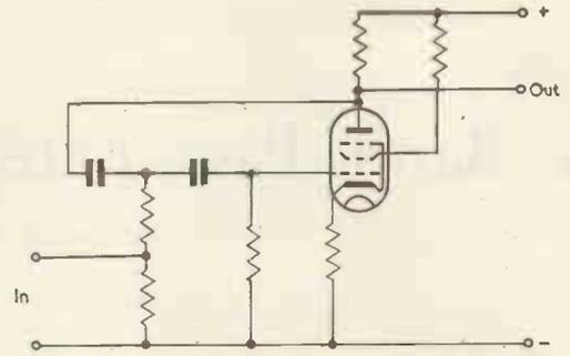
Fig. 3(a). Basic circuit of the single valve resonant network
