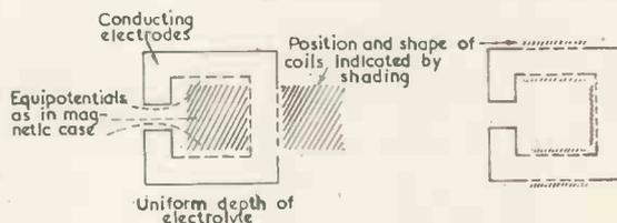
Fig. 6. Direct representation of a two-dimensional problem in an electrolytic bath in which electric potential in the bath is proportional to magnetic potential
