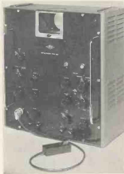
type 723 has been adopted, the cathode-ray tube being mounted vertically and viewed through a surface aluminized mirror. The instrument may therefore be used in conjunction with the Airmec oscilloscope camera type 758. The standard instrument is fitted with a fine focus cathode-ray tube having a 4 inch diameter flat screen providing a green trace. Blue (photographic) or long-persistence cathode-ray tubes may be fitted to special order.
