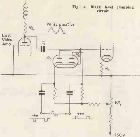
charged to the bias level set by  $VR_1$ , which is adjusted to give black level as zero anode current in  $V_{2b}$ . The critical time-constant here is  $(R_{s1} + R_D/2 + R_{s2} \cdot C_1)$  where  $R_{s1}$  is the source impedance of the video input signal,  $R_D$  is the effective resistance of one diode, and  $R_{s2}$  is the source impedance of the circuit supplying the clamping pulse. The clamping pulse period must be at least four times the critical time-constant indicated.
