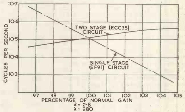
Fig. 7. Variation of frequency with stage gain
