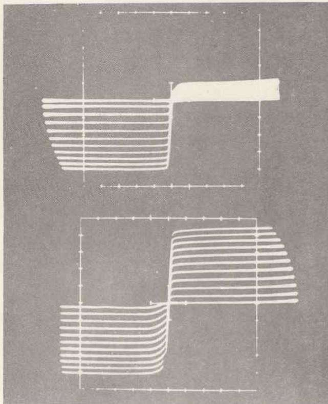
Fig. 13. Collector current/voltage curves for asymmetrical and symmetrical transistors
