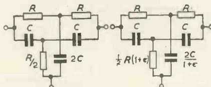
Fig. A. Null transmission network. Fig. B. Minimum transmission network.
