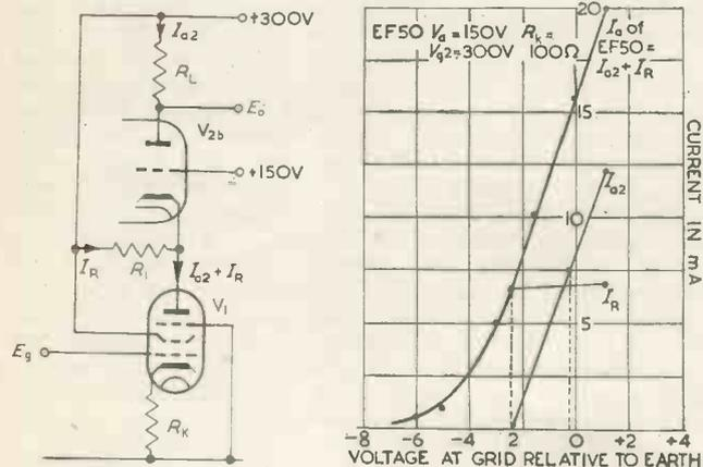
Fig. 1. Method of removing curvature of anode current near cut-off in  $V_{2b}$
