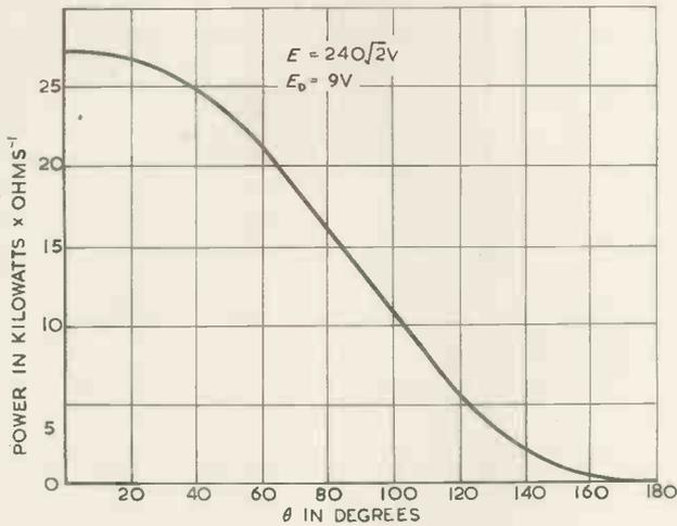
Fig. 4. Variation of power output with delay in firing (linear plot)
