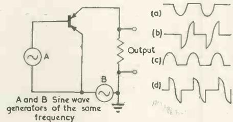
Fig. 17. Phase detector using symmetrical transistor
