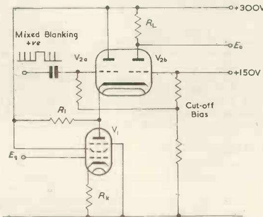
Fig. 3. Addition of  $V_{2a}$  to provide switching circuit
