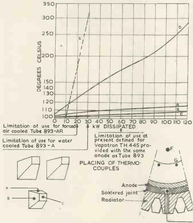
Fig. 3. Overload test in static operation (13kV D.C.) of Vapotron type TH445
