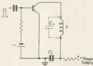
Fig. 14. Switching circuit for horizontal deflexion
