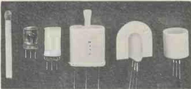
Fig. 1. Experimental transistors
