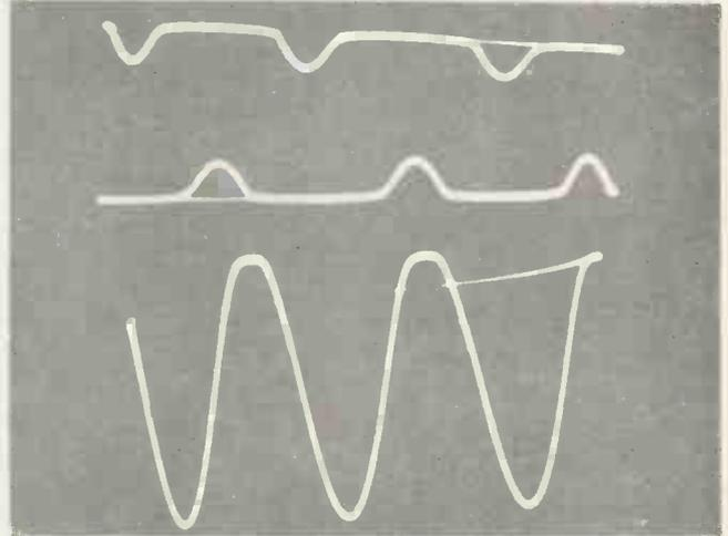
Fig. 6. Waveforms of push-pull amplifier
