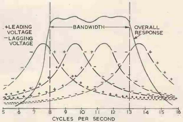
Fig. 4. Illustrating how the phase and amplitude of the voltage from each resonant circuit will vary throughout the band and so contribute to the overall characteristic
