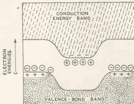
Fig. 12. Energy-level diagram of junction transistor
