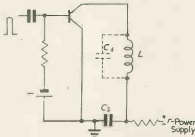
Fig. 14. Switching circuit for horizontal deflexion
