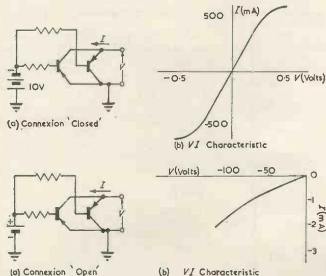
and "open" conditions. The symmetry and low effective resistance of the "closed" condition and the high effective resistance of the "open" condition are apparent.
