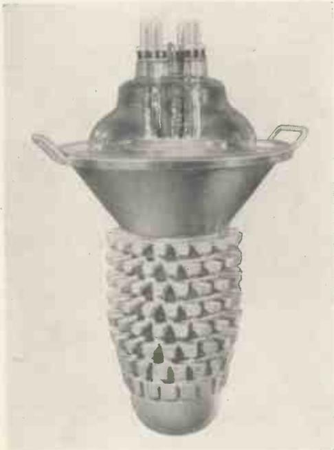
Fig. 1. A typical Vapotron
