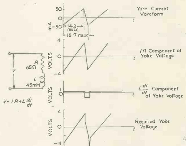
Fig. 19. Theoretical vertical yoke waveforms
