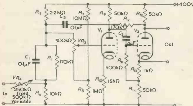
Fig. 2(b). Practical form of Fig. 2(a), using an ECC35 double triode valve
