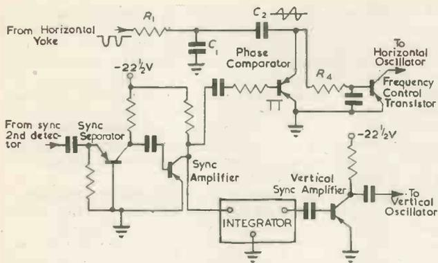
Fig. 26. Sync channel and A.F.C. circuits.
