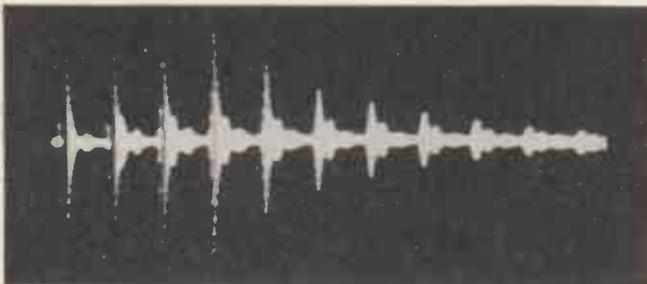
Fig. 2. Correct exposure for small amplitude pulses
