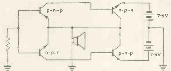
Fig. 8. Class-B push-pull transistor amplifier with complementary symmetry
