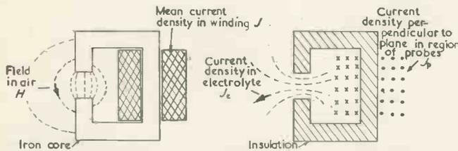
a) Actual electromagnetic arrangement (b) Representation in electrolytic bath
