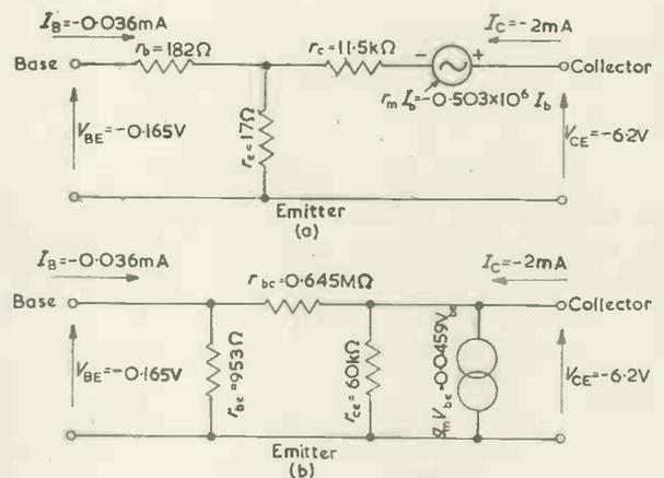
Fig. 2.  $T$  and  $\pi$  equivalent circuits of p-n-p junction transistor
