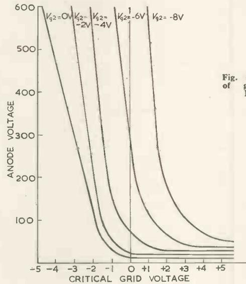
Fig. 6. Characteristics of gas-filled tetrode Mazda 20A2
