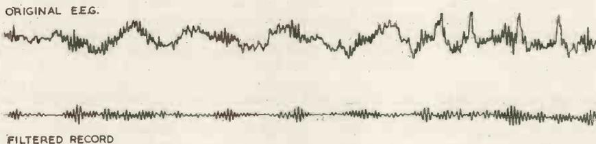
Fig. 11(a). The effect of filtering an electroencephalograph record
