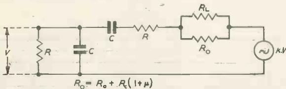
Fig. 9. Equivalent circuit of two-stage filter
