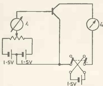
Fig. 10. Test set-up to check transistor symmetry
