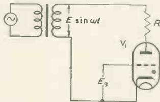
Fig. 1. Basic thyatron circuit
