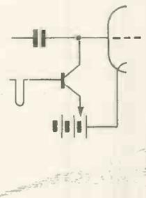
Fig. 16. Transistor clamp circuit
