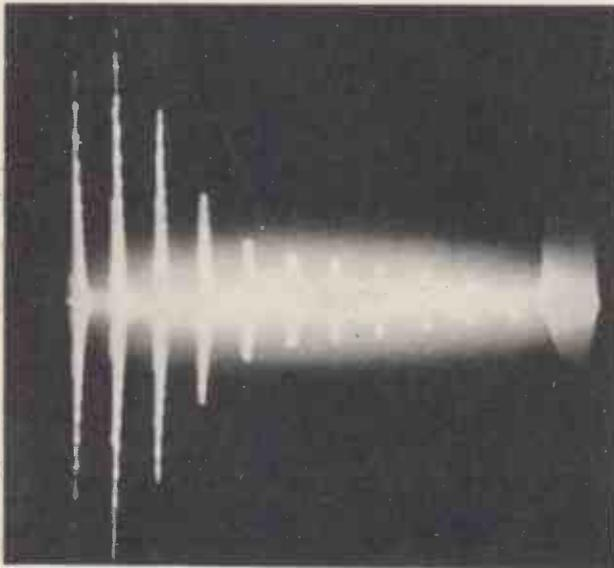
Fig. 1. Illustrating the different exposure time required for differing pulse amplitudes
