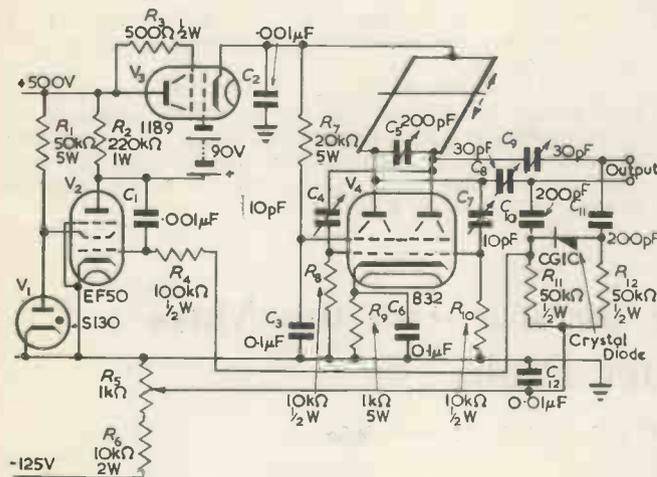
Fig. 1. Circuit of the oscillator
