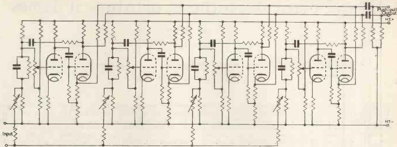
Fig. 10. Complete circuit of an alpha band filter
