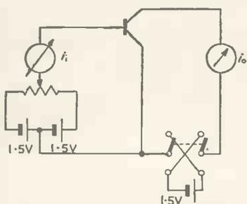
Fig. 10. Test set-up to check transistor symmetry
