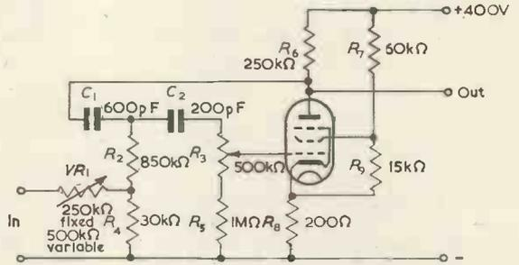
Fig. 3(b). Practical form of Fig. 3(a), using an EF91 pentode valve
