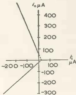
Fig. 11. Collector current symmetry in special transistors
