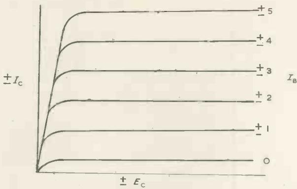
Fig. 4. Characteristic of n-p-n or p-n-p transistor
