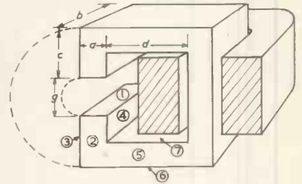
Fig. 4. The determination of the permeance between parts of a magnetic circuit by summing the contribution of easily defined components of the permeance
