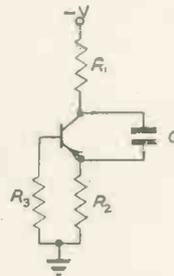
Fig. 20. Vertical oscillator
