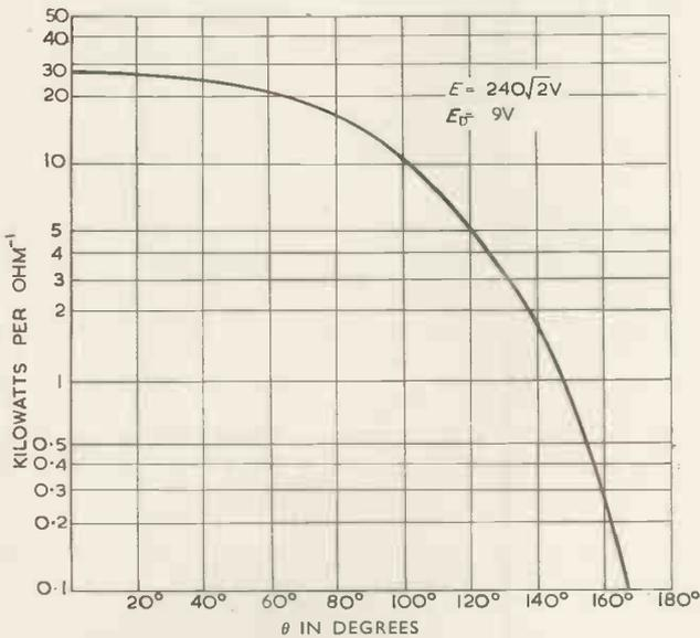
Fig. 5. Variation of power output with delay in firing (logarithmic plot)
