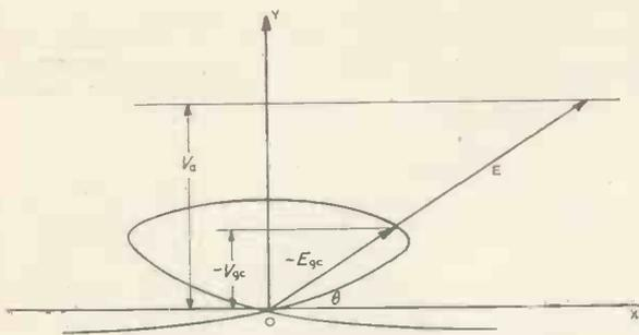
Fig. 7. Vector diagram showing relationship between the vectors and electrode voltages
