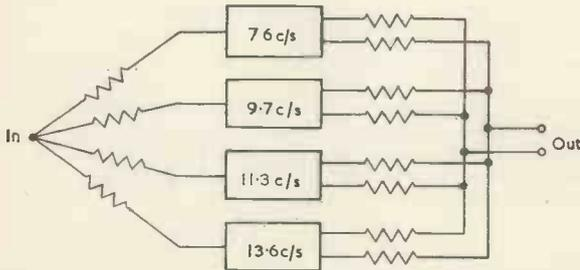
Fig. 1. General scheme of the band-pass filter, showing paralleling of a number of resonant circuits
