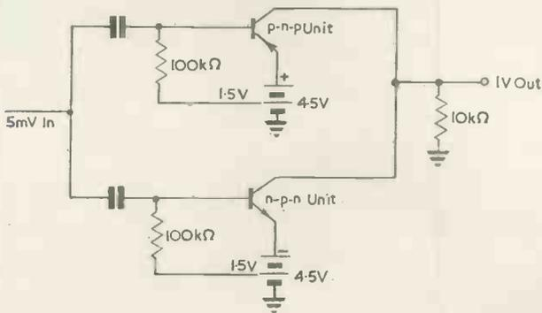
9V instead of 4.5V; thus the amplifier operates in class-A mode, and, since one unit acts as the load for the other, the external load impedance may be removed and a high voltage gain can be obtained for a number of special applications.
