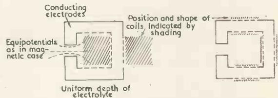
Fig. 6. Direct representation of a two-dimensional problem in an electrolytic bath in which electric potential in the bath is proportional to magnetic potential
