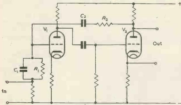
Fig. 2(a). The basic zero phase-shift resonant circuit
