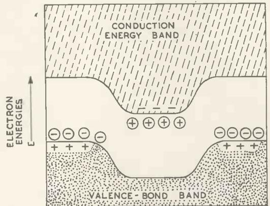
Fig. 12. Energy-level diagram of junction transistor
