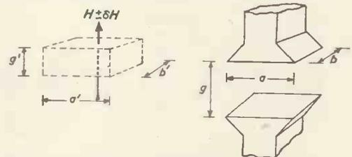
Fig. 1. How the specification of the field required is related to the actual pole dimensions
