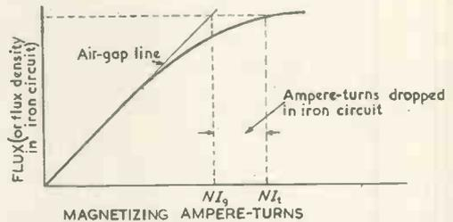
Fig. 7. Magnetization curve of a D.C. magnet from which can be deduced the field in the gap and the ampere-turns dropped in the iron circuit
