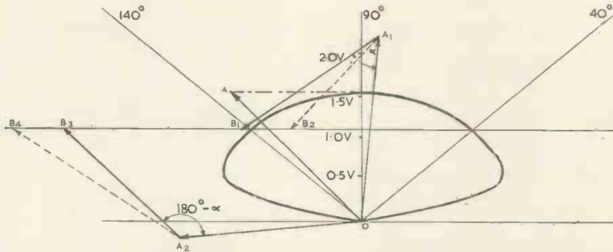
Fig. 9. Complete vector diagram showing two possible control signals to drift firing point from  $40^\circ$  to  $140^\circ$
