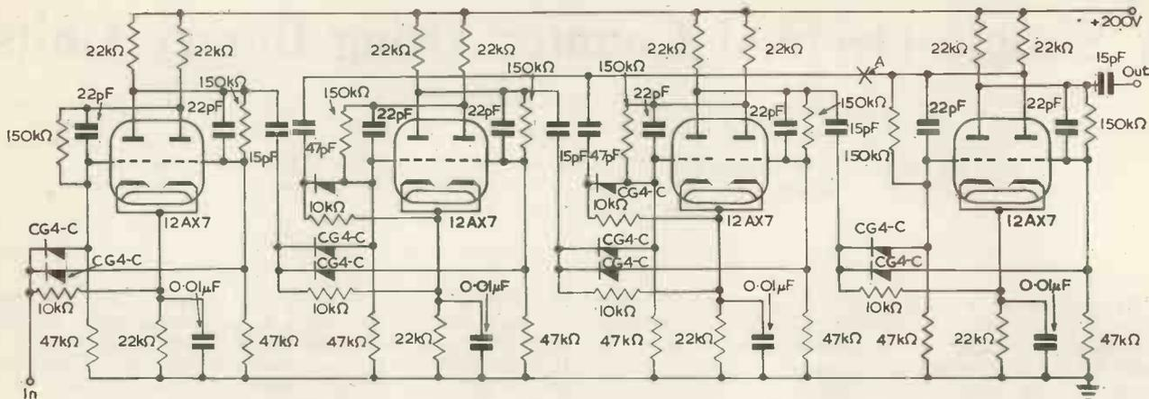
Fig. 1. A complete decimal counter Breaking the feedback loop at A converts to normal binary counting
