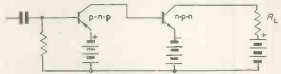
Fig. 7. Direct-coupled transistor amplifier
