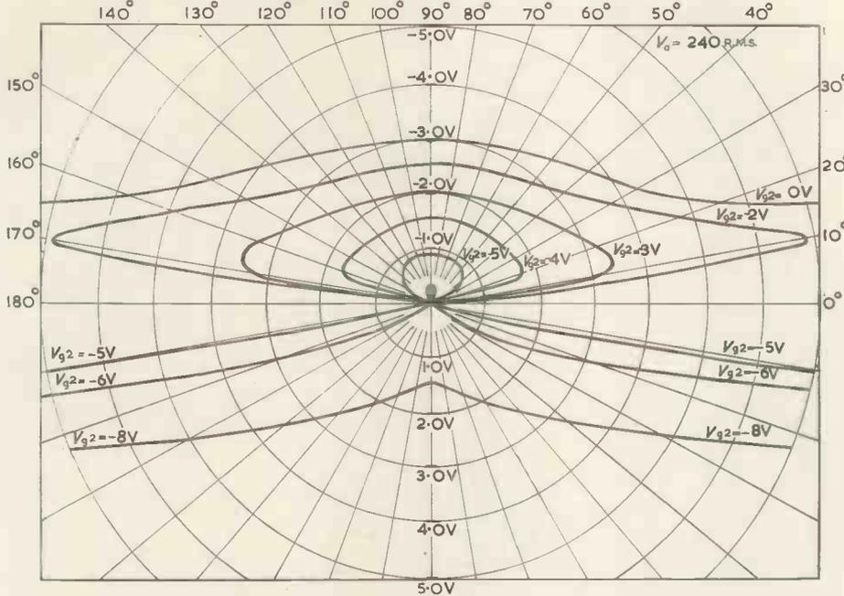
Fig. 10. Critical grid characteristics of Mazda 20A2 plotted in polar co-ordinates
