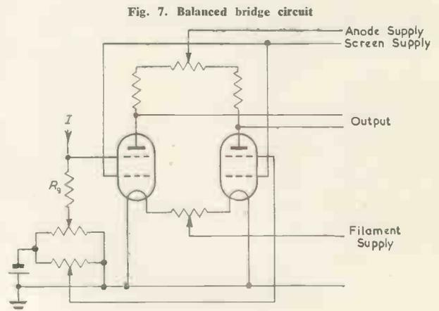
Fig. 7. Balanced bridge circuit
