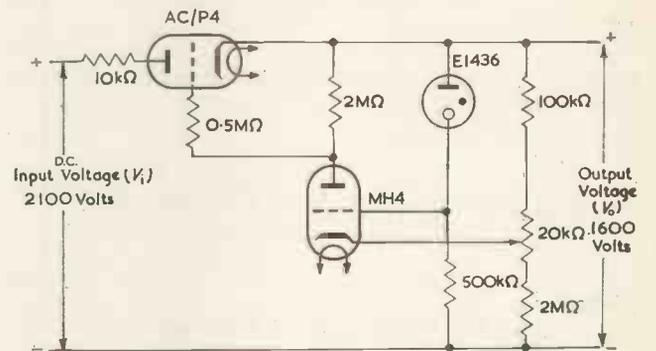
Fig. 5. Series parallel valve stabilizer for microwave oscillator
