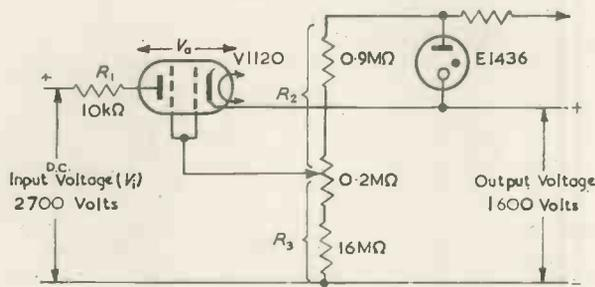
Fig. 3. Series valve stabilizer for microwave oscillator
