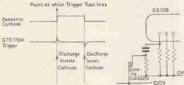
Fig. 3. Variation of potentials in carry circuit Fig. 4. Zeroing circuit
