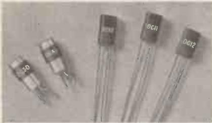
and OC12 are designed for economy in power supplies and, in both amplifier and oscillator circuits, they will operate satisfactorily from H.T. supplies as low as 1.5V, with current consumptions of similar low order. Under suitable conditions they will work with H.T. supplies of only a fraction of a volt.
