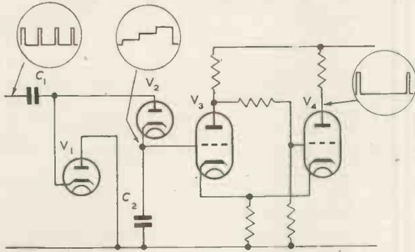
Fig. 3. Use of circuit shown in Fig. 1. as a discharger in a dividing chain
