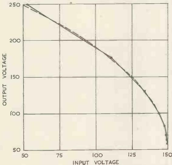
Fig. 1. Theoretical calibration curve composed of straight segments. The broken line represents an ideal parabola.
