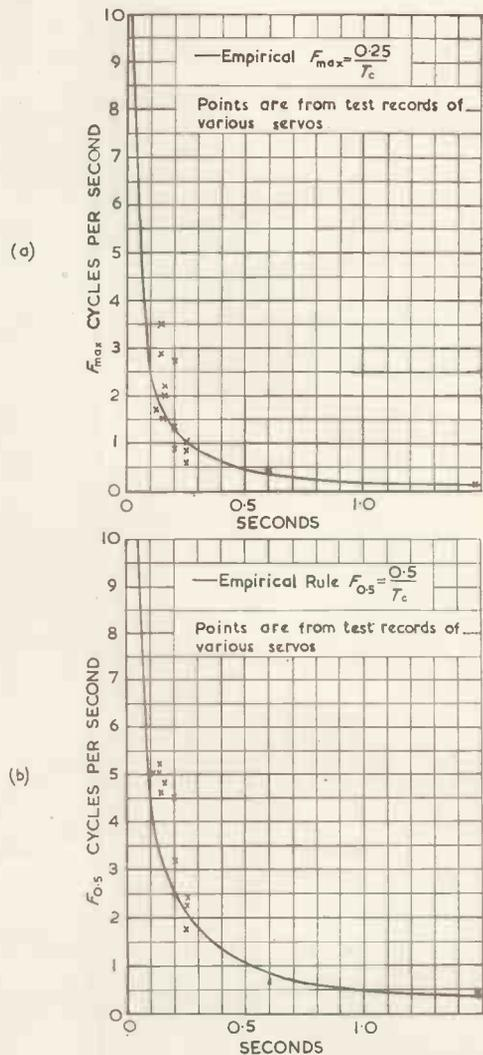
Fig. 21 (a). Experimental frequency at  $Q_{max}$ . (b). Experimental frequency at cut-off
