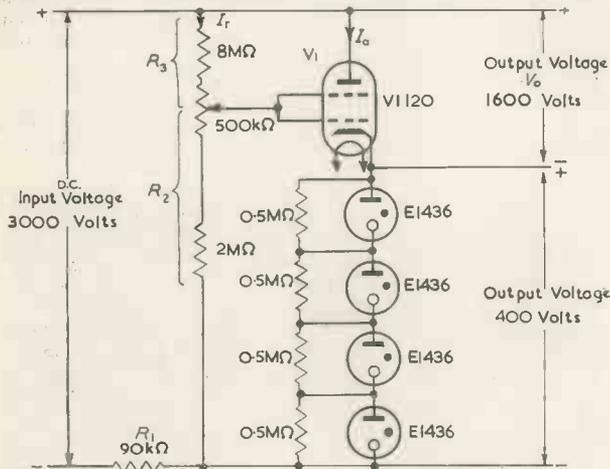
Fig. 1. Parallel valve stabilizer for microwave oscillator.
