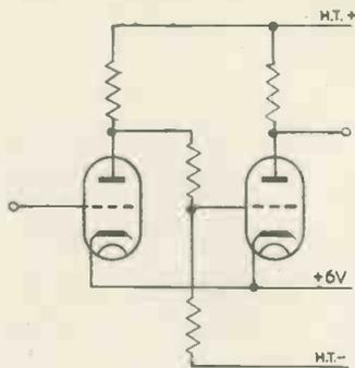
Fig. 22. Use of a potential divider with negative bias for interstage coupling
