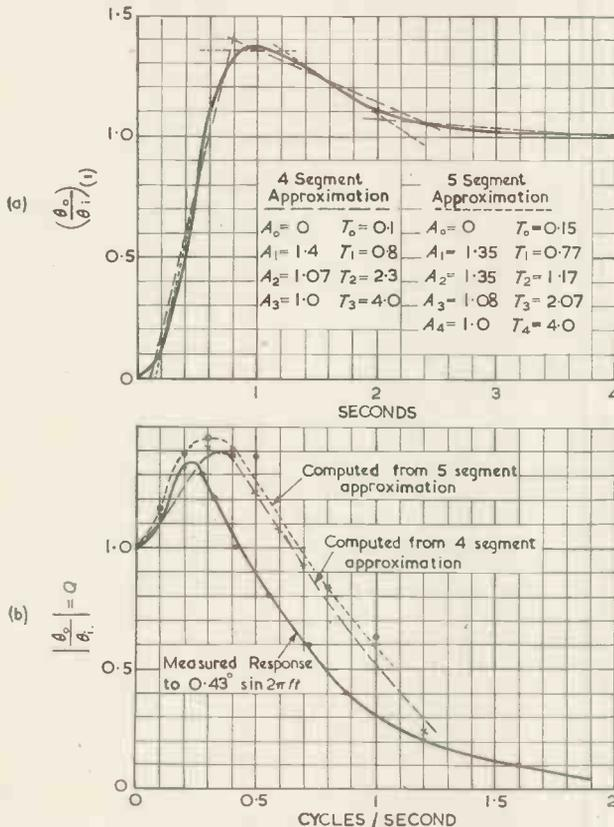
Fig. 19 (a). Measured Response to  $1^\circ (t)$ . (b) Auto follow radar servo
