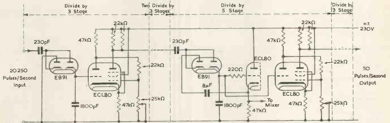
Fig. 5. Circuit for counting down from 20 250c/s to 50c/s for a television pattern generator
