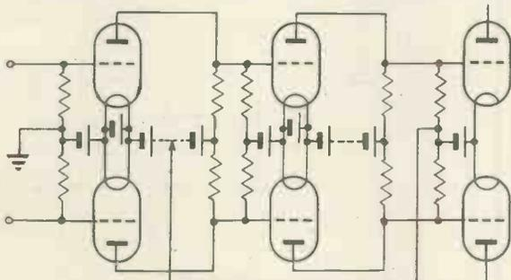
Fig. 23. Mean level feedback in a battery operated amplifier
