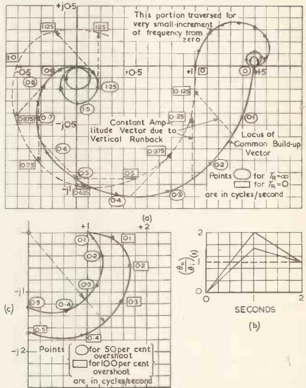
Fig. 17 (a). Vector loci for limiting cases of runback times  $\begin{cases} T_R = 0 \\ T_R = \infty \end{cases}$
