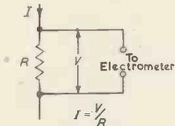
Fig. 2. Voltage drop method
