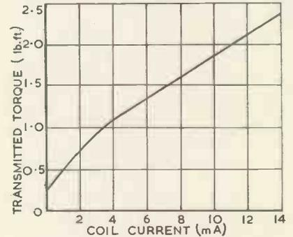
Fig. 1. Relation between output torque and coil current
