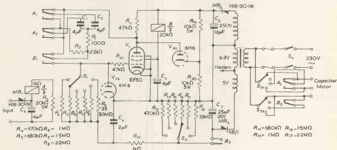
Fig. 1. Circuit of the controller
