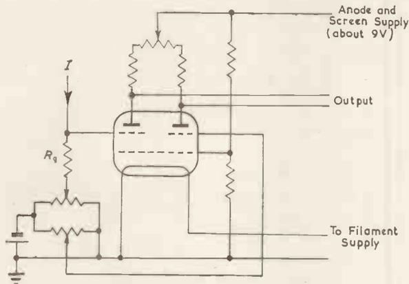
Fig. 8. Balanced tetrode circuit using double valve
