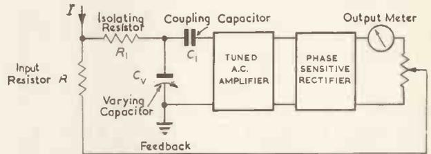
Fig. 9. Capacitance modulator electrometer
