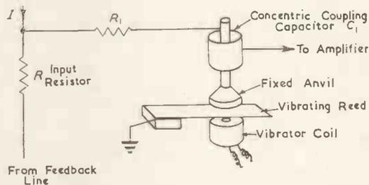
Fig. 10. Principle of vibrating reed electrometer
