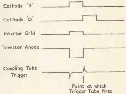
Fig. 6. Variations in potentials in carry circuit when an inverter is fitted
