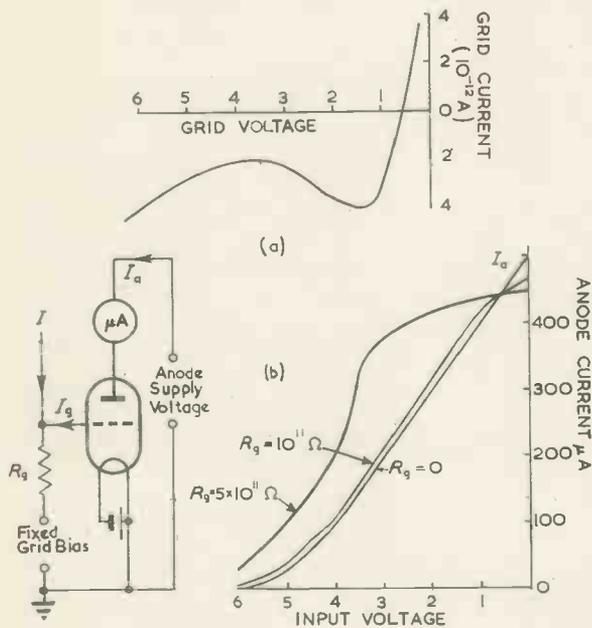
Fig. 5. Simple valve electrometer
