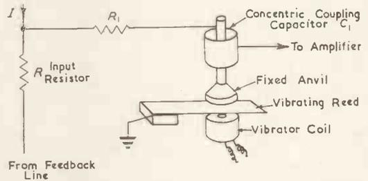
Fig. 10. Principle of vibrating reed electrometer
