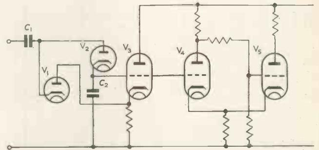
Fig. 4. Method of maintaining voltage steps at a uniform amplitude
