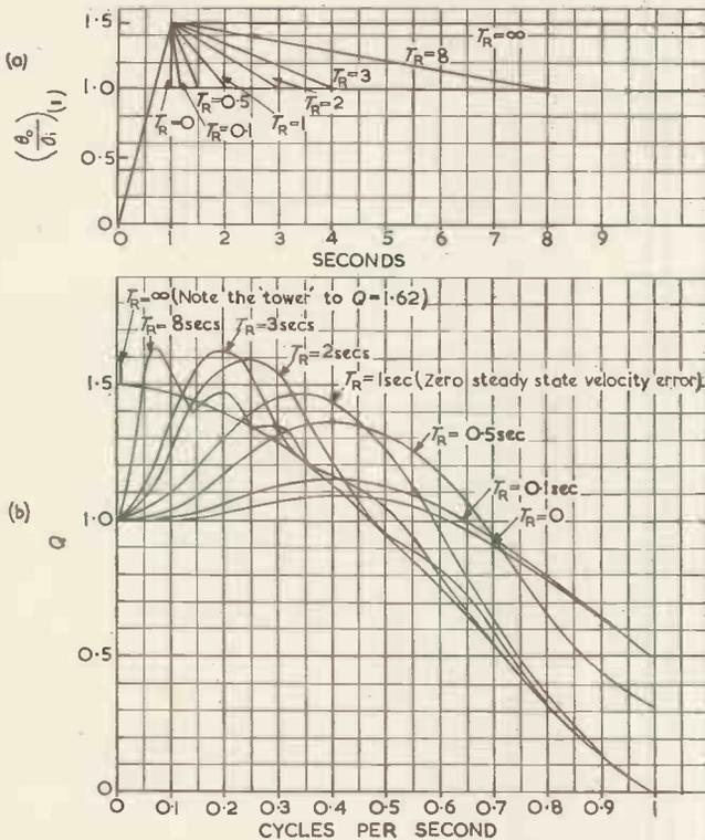
Fig. 16 (a). Two segment approximations to step response with single overshoot to  $A_{max} = 1.5$  at 1 second and various values of runback time  $T_R$ .
