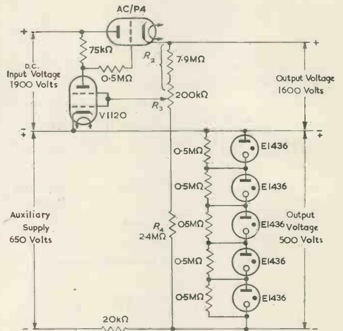
Fig. 7. Series parallel valve stabilizer for microwave oscillator
