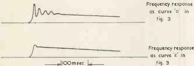
Fig. 4. Observed transient response
