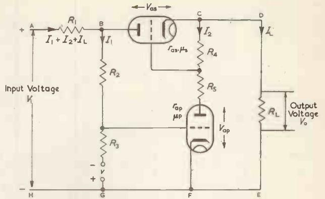
Fig. 10. Equivalent circuit of Fig. 9
