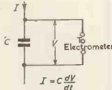
Fig. 3. Capacitor charging method.
