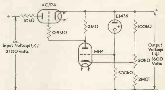
Fig. 5. Series parallel valve stabilizer for microwave oscillator
