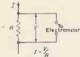
Fig. 2. Voltage drop method
