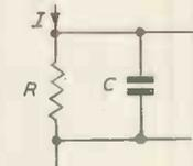
Fig. 4. Effective circuit of electrometer
