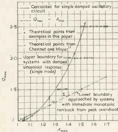
Fig. 18. Relation between  $Q_{max}$  and  $A_{max}$  for R.P.C. servos
