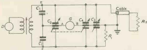
Fig. 2. Bridge for impedance measurements on coaxial cables
