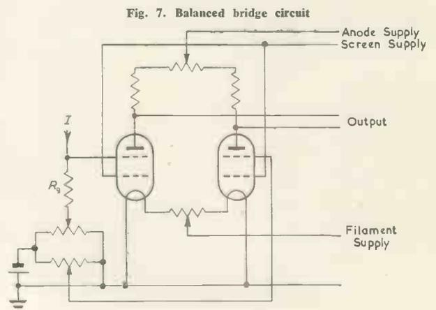
Fig. 7. Balanced bridge circuit
