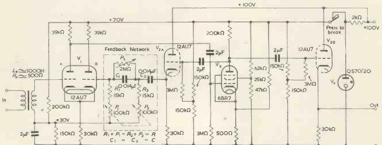
continuously changed by rotation of the ganged potentiometers  $P_1$  and  $P_2$ . The transient response can be modified by adjustment of  $P_3$ . The output of the unit is taken from the anode of  $V_3$  via a second cathode follower,  $V_{2b}$ . The filter has been designed for a 100 volt supply and it is therefore necessary to operate the "press to break" switch to ensure that  $V_4$  is struck.
