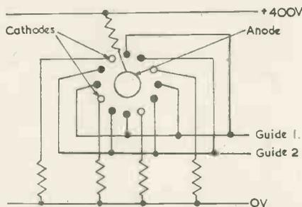
Fig. 1. Schematic diagram of Dekatron
