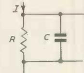
Fig. 4. Effective circuit of electrometer
