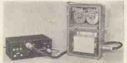
The input to the recorder is opposed by the feedback voltage from a resetting potentiometer which is controlled by the position of the pen. The error, being the difference between these voltages, is amplified and drives the pen movement until the feedback voltage balances the input.
