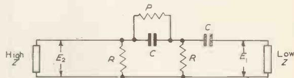
Fig. 5. Equivalent feedback circuit
