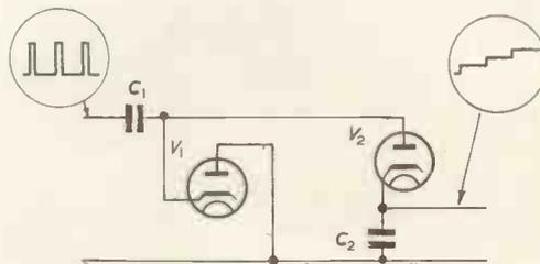
Fig. 2. Divider circuit
