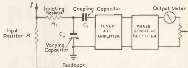
Fig. 9. Capacitance modulator electrometer
