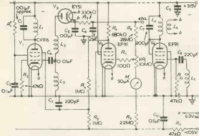
Fig. 2. The e.h.t. generator and stabilizer
