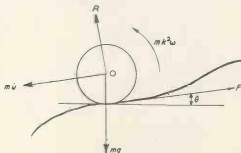
Fig. 1. Forces acting on a sphere moving on a sloping surface
