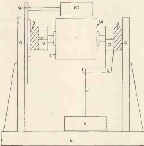
Fig. 3. Simplified mechanical arrangement of dynamic balancer
