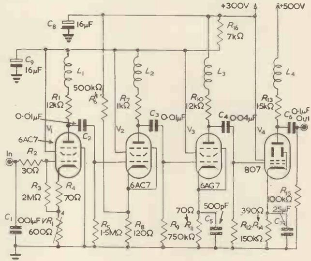
Fig. 4. The circuit of the video-amplifier
