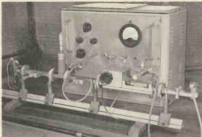
Fig. 1. A representative X-band test bench, including one klystron, variable attenuator, wavemeter, v.s.w.r. indicator and crystal detector
