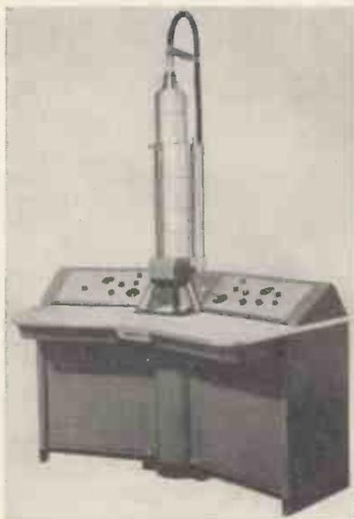
The type EMU-3A microscope. The overall dimensions are:—Height 7 ft. 8 in., Width 4 ft. 9 in., Depth 5 ft. 10 in.
