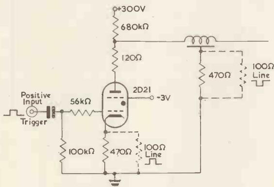
Fig. 2. First model of thyatron oscillator
