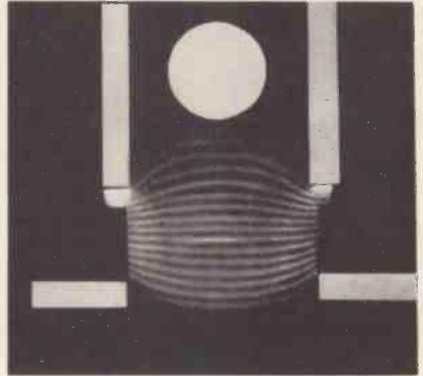
Fig. 5. Equipotential plot of the gun assembly obtained with the rubber sheet model
