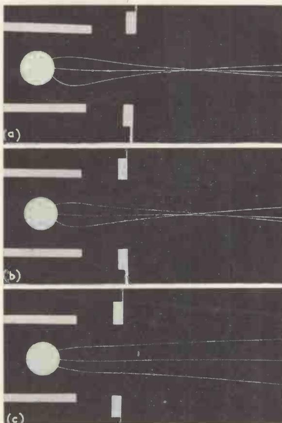
Fig. 3. Electron trajectories for spacings of (a) 0.035in, (b) 0.028in, (c) 0.018in between the front of the filament and the front of the grid using a cylindrical cross-section for the filament
