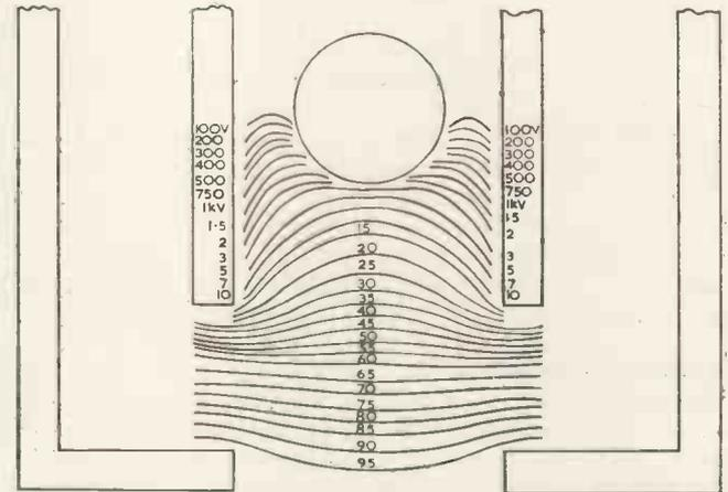
Fig. 6. The calculated field configuration obtained by the relaxation method (Compare with Fig. 5)
