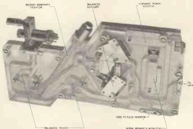
Fig. 4. An “integrated” version of the r.f. head in Fig. 3 (Demonstration block with Perspex replacing the top half.)
