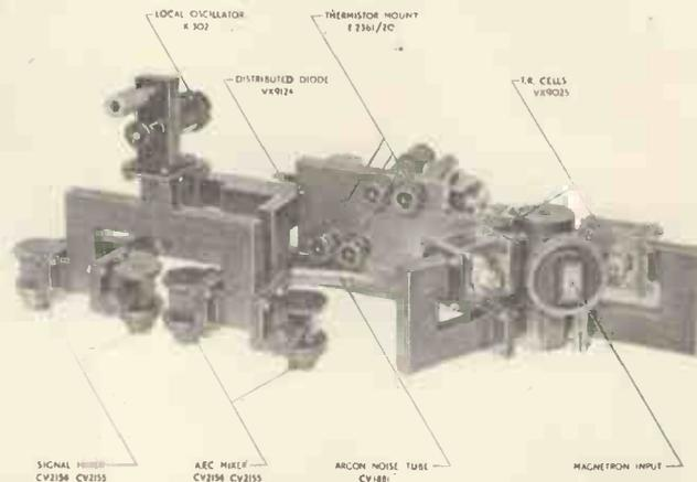
Fig. 3. A representative r.f. head in orthodox waveguide “plumbing”
