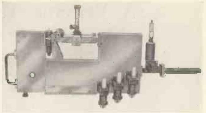
Fig. 5. An "integrated" r.f. production test bench for X-band t.r. cells, including 3 klystron feed, variable attenuator, dummy load and power monitor
