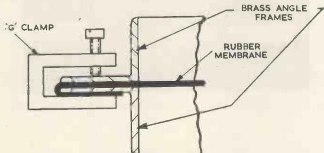
Fig. 2. Method of clamping rubber sheet
