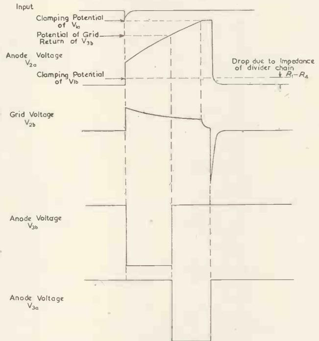
Fig. 3. Scaling circuit waveforms
