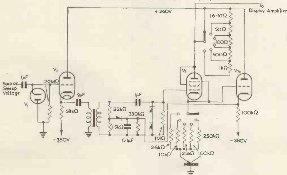
The circuit for step and sweep currents is shown in Fig. 7. The input voltage is transformer coupled, rendered positive going by germanium diodes, and applied between the grid of  $V_5$  and the cathode of  $V_{7a}$ . The reason for connecting to the cathode of  $V_{7a}$  rather than to the emitter terminal is that interwinding capacitance causes spurious pulses in the emitter circuit. A small portion of the 150V peak waveform is rectified and used to bias  $V_5$  to cut-off.
