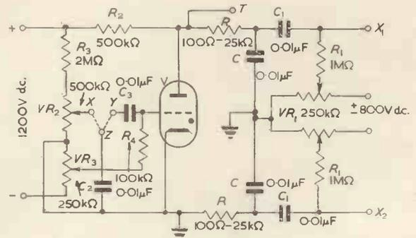
Fig. 5. The time-base circuit
