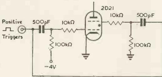
Fig. 6. Triggering circuit in which both grids are pulsed simultaneously
