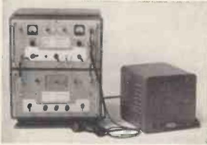
as the transmitter and one on 200kc/s. Services provided are c.w., m.c.w., and r.t. and loudhailer. The output of the transmitter is approximately 50W. The receiver has a built-in vibrator power supply, while the transmitter is fed from a separate rotary transformer unit.
