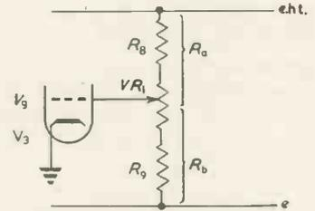
Fig. 3. Calculation of output voltage
