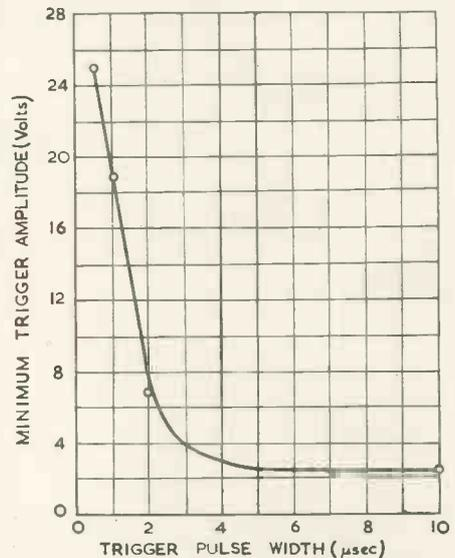
Fig. 5. Trigger amplitude/pulse width for fixed bias (-4V)
