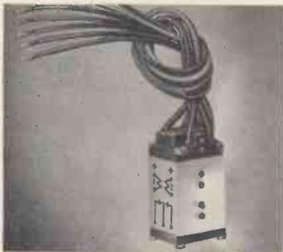
This relay is a magnetically self-shielded unit capable of operating from a power input of 10μW and being of balanced construction functions efficiently in any position. The overall measurements of the relay are 1½in by ¾in by ¾in.
