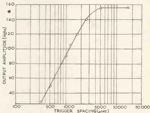
Fig. 3. Output amplitude/input trigger spacing for a fixed load and a 680  $\mu\text{sec}$  anode time-constant
