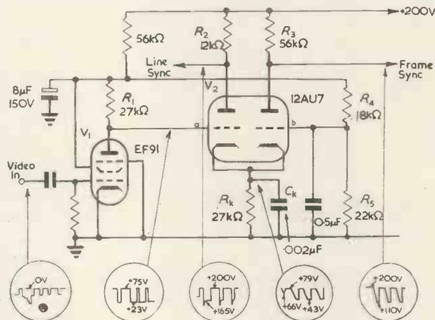
Fig. 2. Improved synchronizing separator
