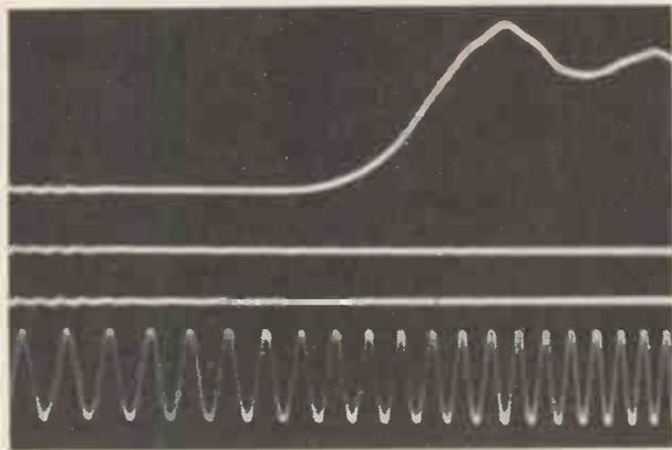
Fig. 6. Oscillogram of a pulse due to the impact of a bullet
