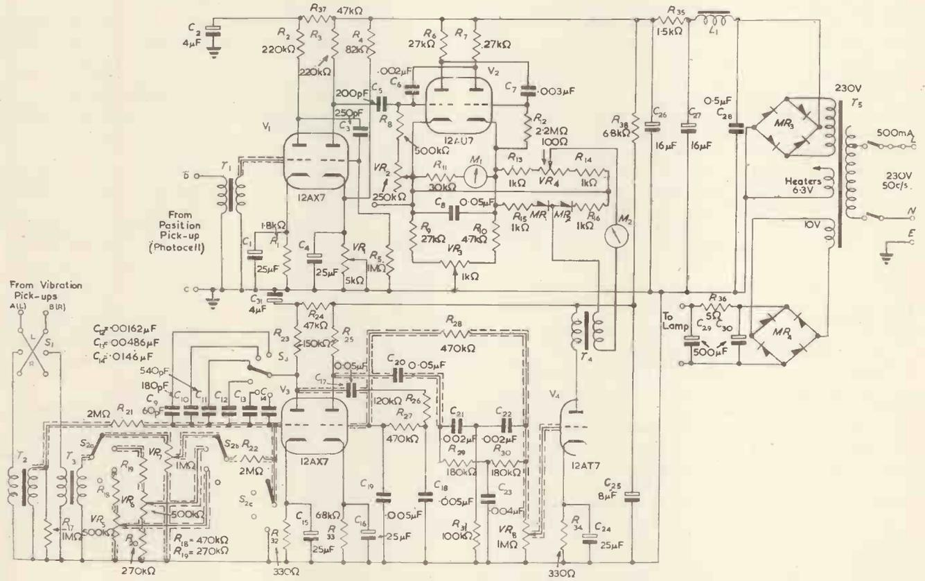
Fig. 5. Circuit of dynamic balancer
