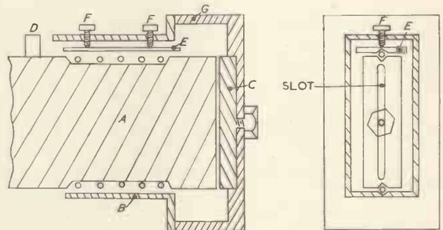
Fig. 7. Capacitor unit for use with a bar of rectangular cross-section
