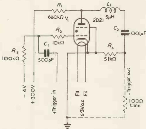
Fig. 7. The final circuit
