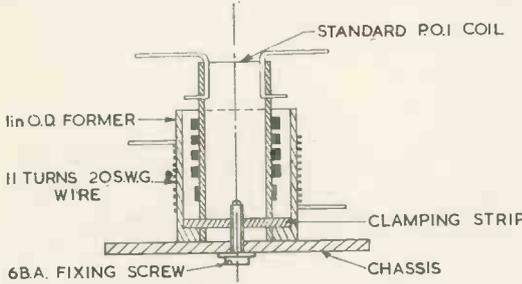
Fig. 1. The r.f. heater supply coil
