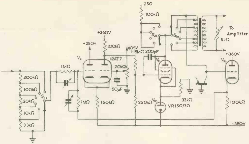
Fig. 8. (above) Collector voltage amplifier.
