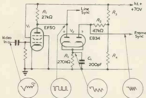
Fig. 1. Pye synchronizing separator
