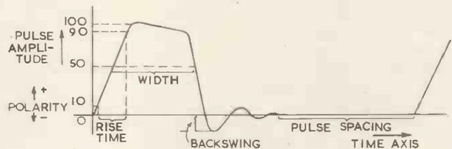
Fig. 1. Pulse waveform
