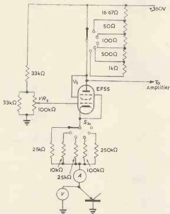
Fig. 6. Emitter current amplifier (direct voltage input)
