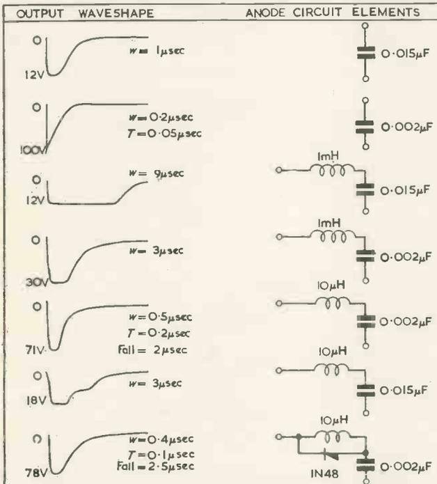
Fig. 4. Anode circuit networks and relative waveshapes
