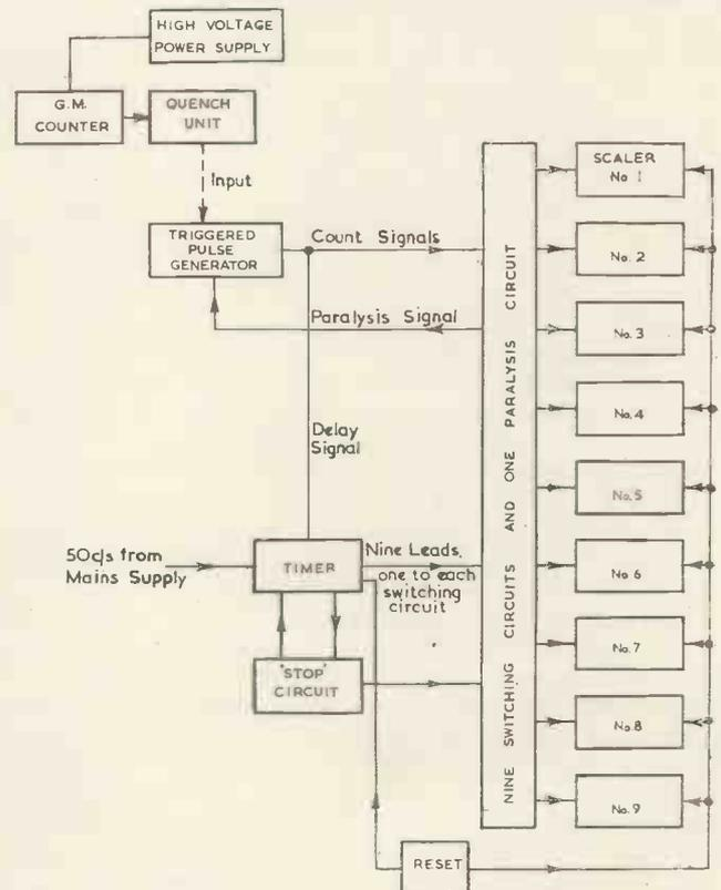
Fig. 1. Equipment for the determination of mean lives
