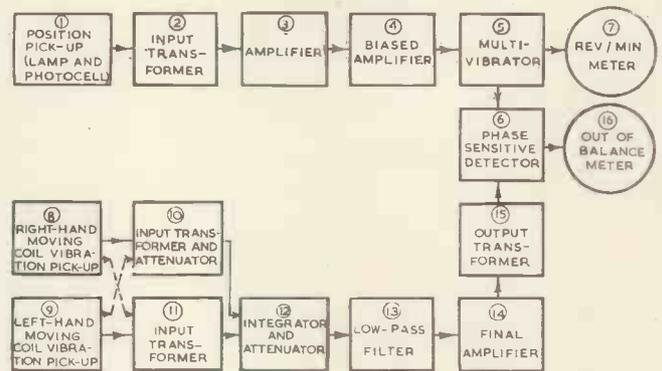
Fig. 4. Arrangement of electrical equipment of dynamic balancer
