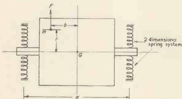
Fig. 1. Gyroscope running in spring-restrained bearings
