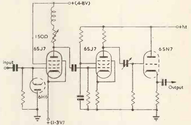
Fig. 5(b). Pentode slicer circuit with phase inverting amplifier and differentiator
