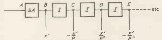
Fig. 4. Effect of coupling between outputs
