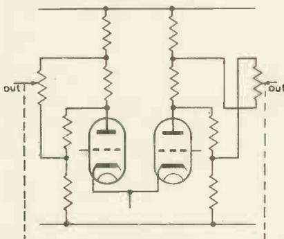
Fig. 2. The principle applied to a push-pull circuit
