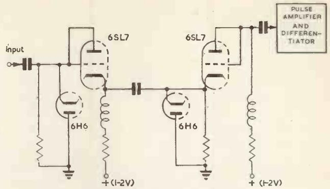
Fig. 5(a). Double diode slicer circuit
