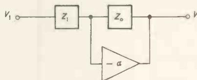
Fig. 6. Transfer function of amplifier
