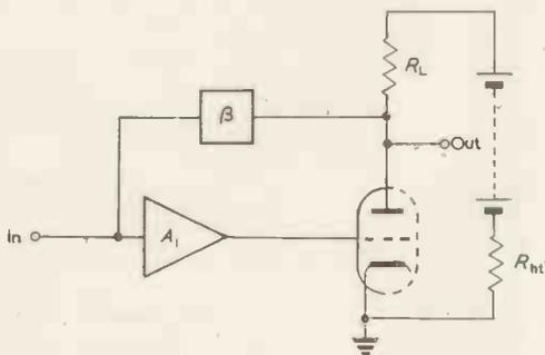
Fig. 5. Transfer from anode to common h.t. resistance
