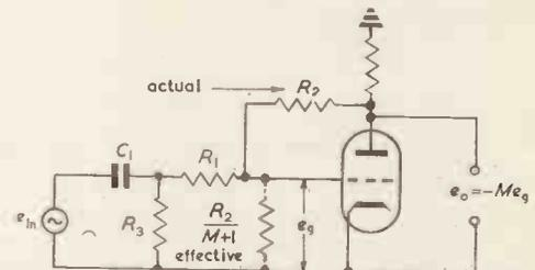
Fig. 12. High-pass filter, showing actual and effective circuit components
