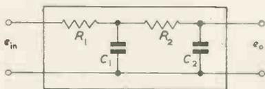
Fig. 5. Two section RC network—low-pass
