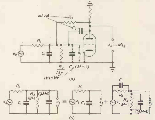
Fig. 11(a). Low-pass filter, showing active and effective circuit components (b). Low-pass equivalent circuit, showing how cut-off frequency is independent of  $M$ , if  $C_1 R_1 = C_2 R_2$
