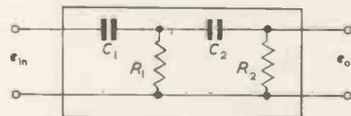
Fig. 6. Two section RC network—high-pass
