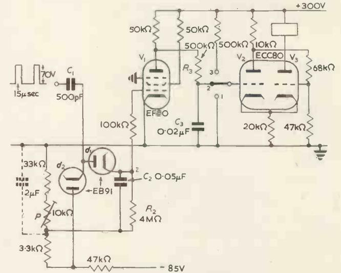
Fig. 12. Practical circuit of frequency-sensitive relay (Values for switching frequency of 500p/s)
