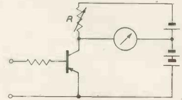
Fig. 1. Transistor voltmeter showing bridge arrangement
