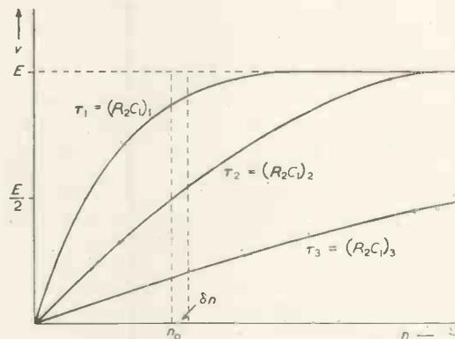
Fig. 10. Family of curves showing  $v = E \cdot n \tau / 1 + n \tau$  for different values of  $\tau$ .
