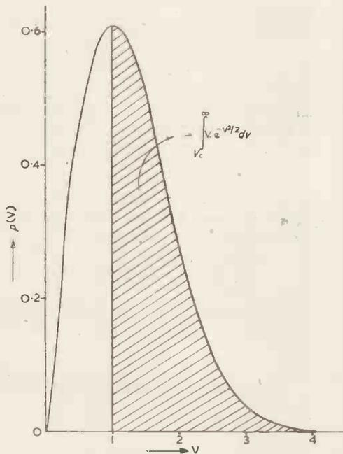
Fig. 3. Probability distribution of noise voltage
