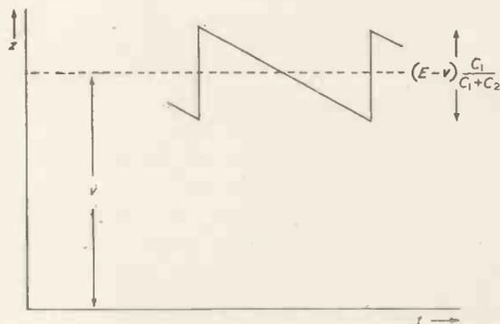
Fig. 8. Integrator output waveform
