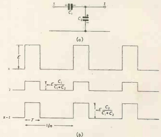
Fig. 2. Basic integrator without diodes
