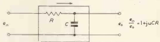
Fig. 3. Single section low-pass RC network
