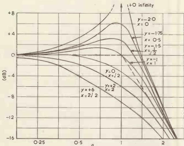
Fig. 2. Filter response curves numbered with their y value in the expression
