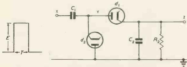
Fig. 1. Circuit of diode pump integrator
