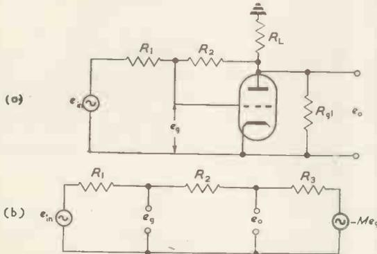
Fig. 13(a). Negative feedback over single stage
